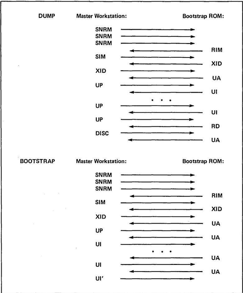
**Figure 2-1. Communications Dump and Bootstrap Protocol.**
