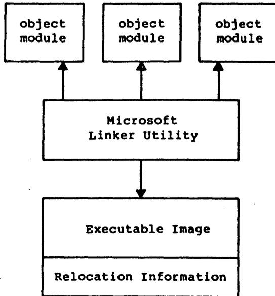
Figure 1. MS-LINK Operation
