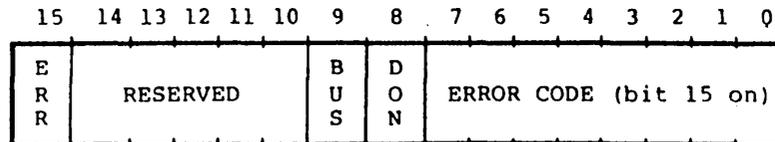
The status word is zero on entry and is set by the driver interrupt routine on return.
