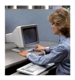
The keyboard consists of a standard alphanumeric "typewriter style" section, 14-key numeric pad, and 8-key status/control function pad, 6-key cursor control pad, 4-key page control pad and 10 programmable function keys. The keyboard also provides software controllable LED indicators on 8 keys.
