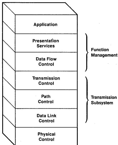
Figure 4-1. Layers of an SNA Network
