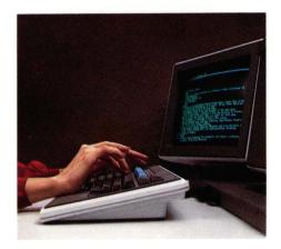
The 98-key keyboard has a typewriter-style sculptured surface, contoured keycaps, and a palm rest for operator comfort. It is detachable and connected to the video display unit *via* a 5-foot coiled cable. The keyboard provides a 14-key numeric pad, an 8-key status/control function pad, a 6-key cursor control pad, a 4-key page control pad, and 10 user-definable function keys. The keyboard also provides software-controllable LED indicators on 8 keys.
