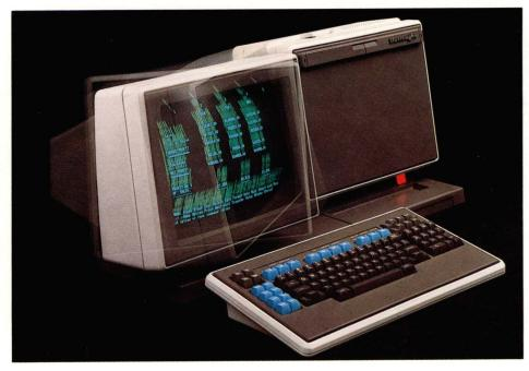
The 15-inch, high quality video display unit is mounted horizontally in "landscape" mode. The unit is fully articulated and may be tilted from 10 degrees to 30 degrees above the horizontal plane, and rotated  $\pm$  30 degrees for easy viewing. The display screen has an 18 MHz monitor, green phosphor to help reduce eyestrain, and an etched surface that eliminates glare. A brightness control can be easily accessed by the operator.
