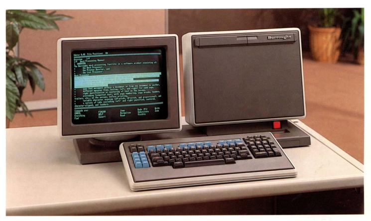
Burroughs family of B 21 workstations is the entry level member of Burroughs B 20 Series of desktop micro-computers.
