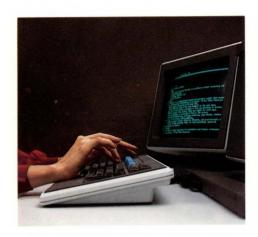
The 98-key keyboard has a typewriter style sculptured surface, contoured keycaps, and a palm rest for operator comfort. It is detachable and connected to the display unit with a coiled cable. The keyboard provides a 14-key numeric pad, an 8-key status/control function pad, a 6-key cursor control pad, a 4-key page control pad, and 10 user-definable function keys. The keyboard also provides software controllable LED indicators on 8 keys.
