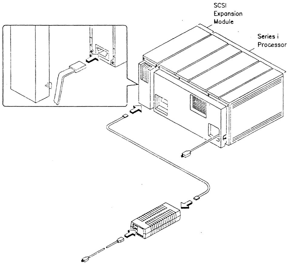
Figure 2-7. Connecting Power to a Series i System
