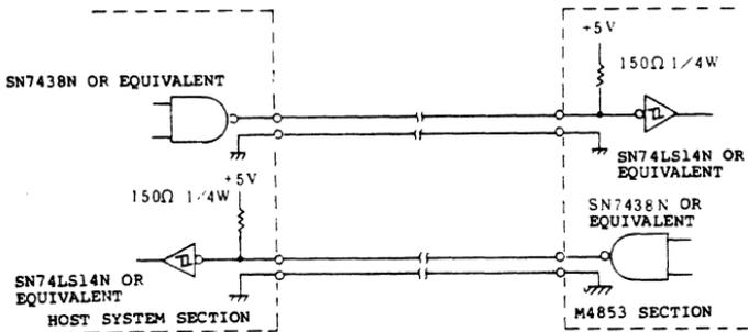
Fig. 3-2 Recommended Line Driver and Line Receiver Circuits
