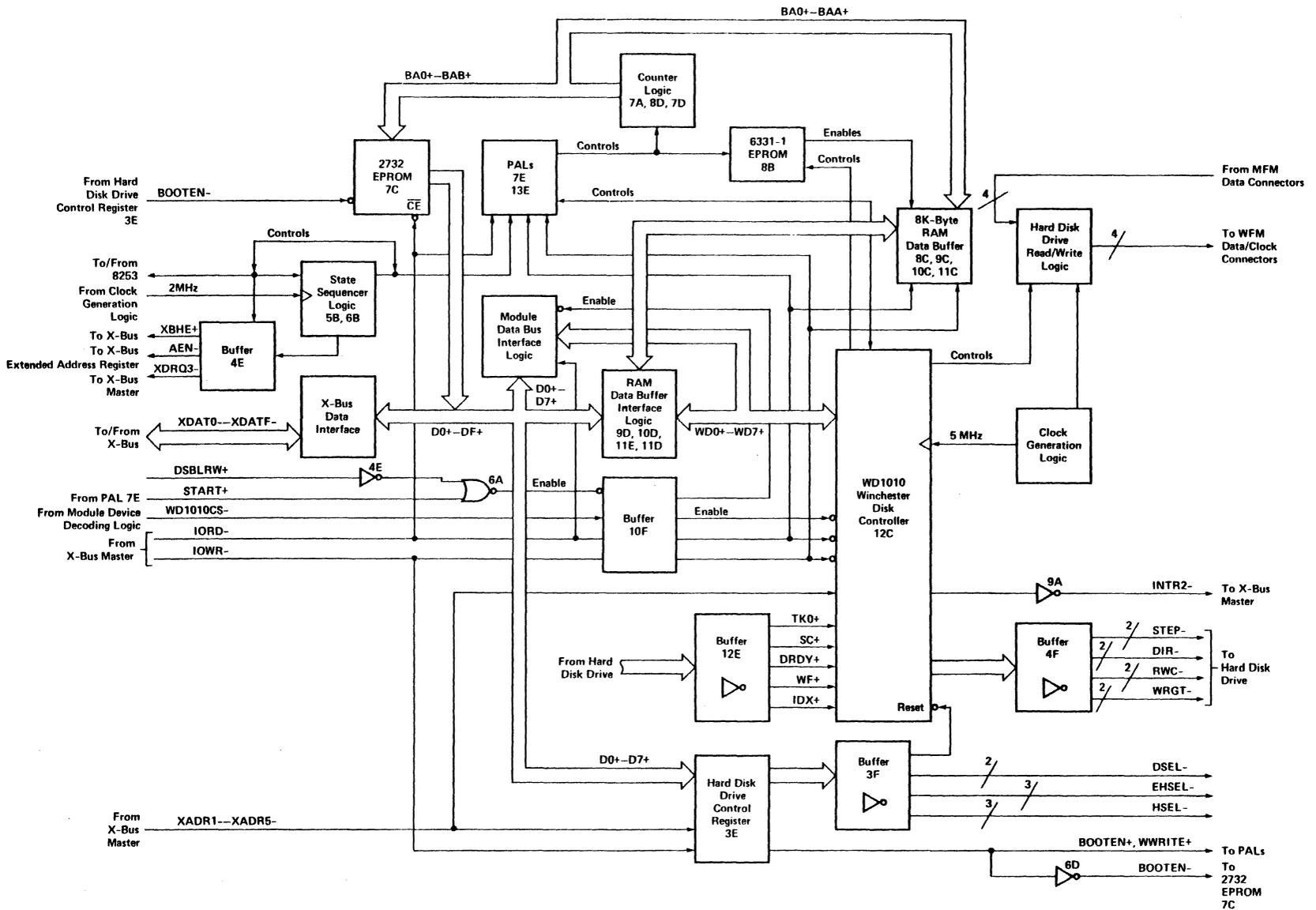
Figure 3-3. Hard Disk Controller Logic Functional Block Diagram.
