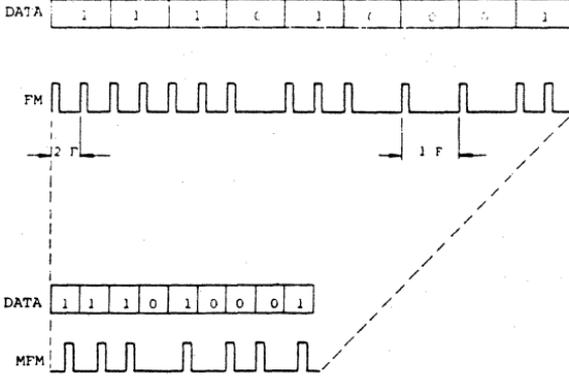
Fig. 4-2 Comparison of FM and MFM Encoding Systems
