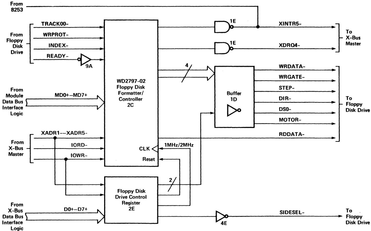
3-2. Floppy Disk Controller Logic Functional Block Diagram.
