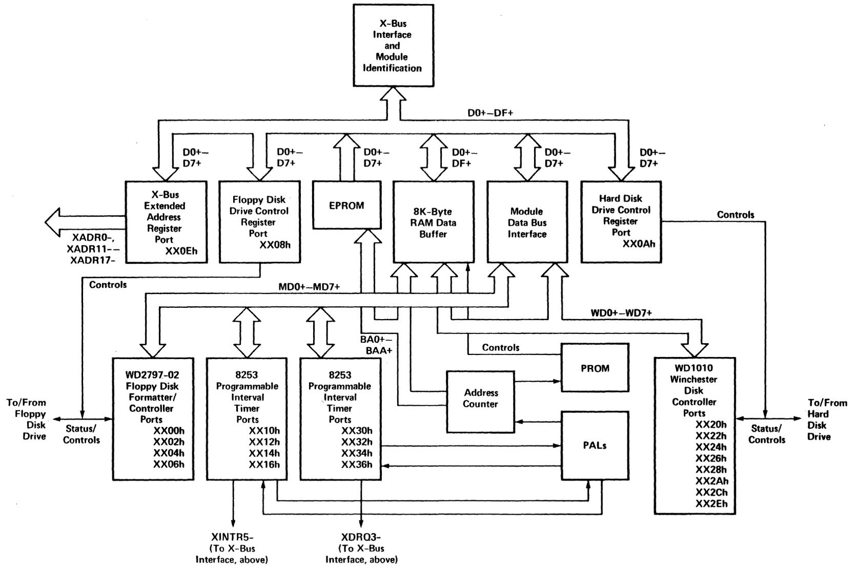
Figure 2-1. Floppy/Hard Disk Module Functional Logic Block Diagram.
