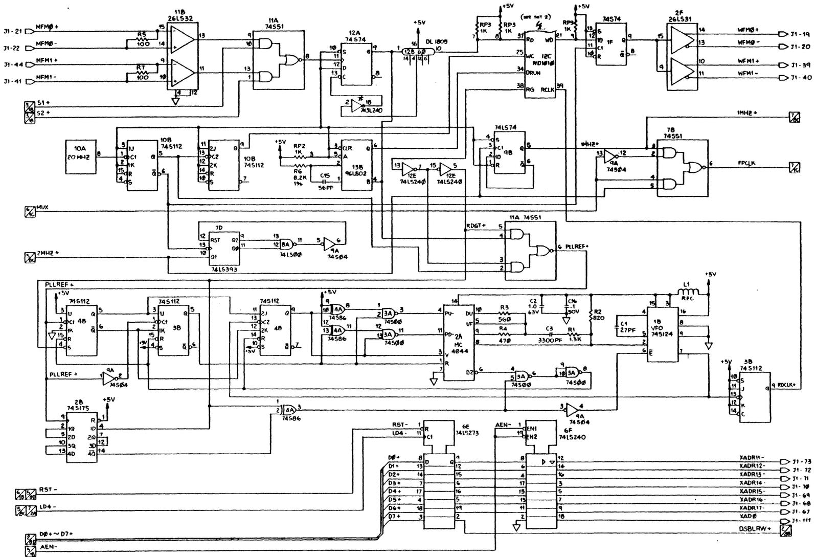
Figure 3-1. Floppy/Hard Disk Module Schematic Diagram. (Page 4 of 7)
