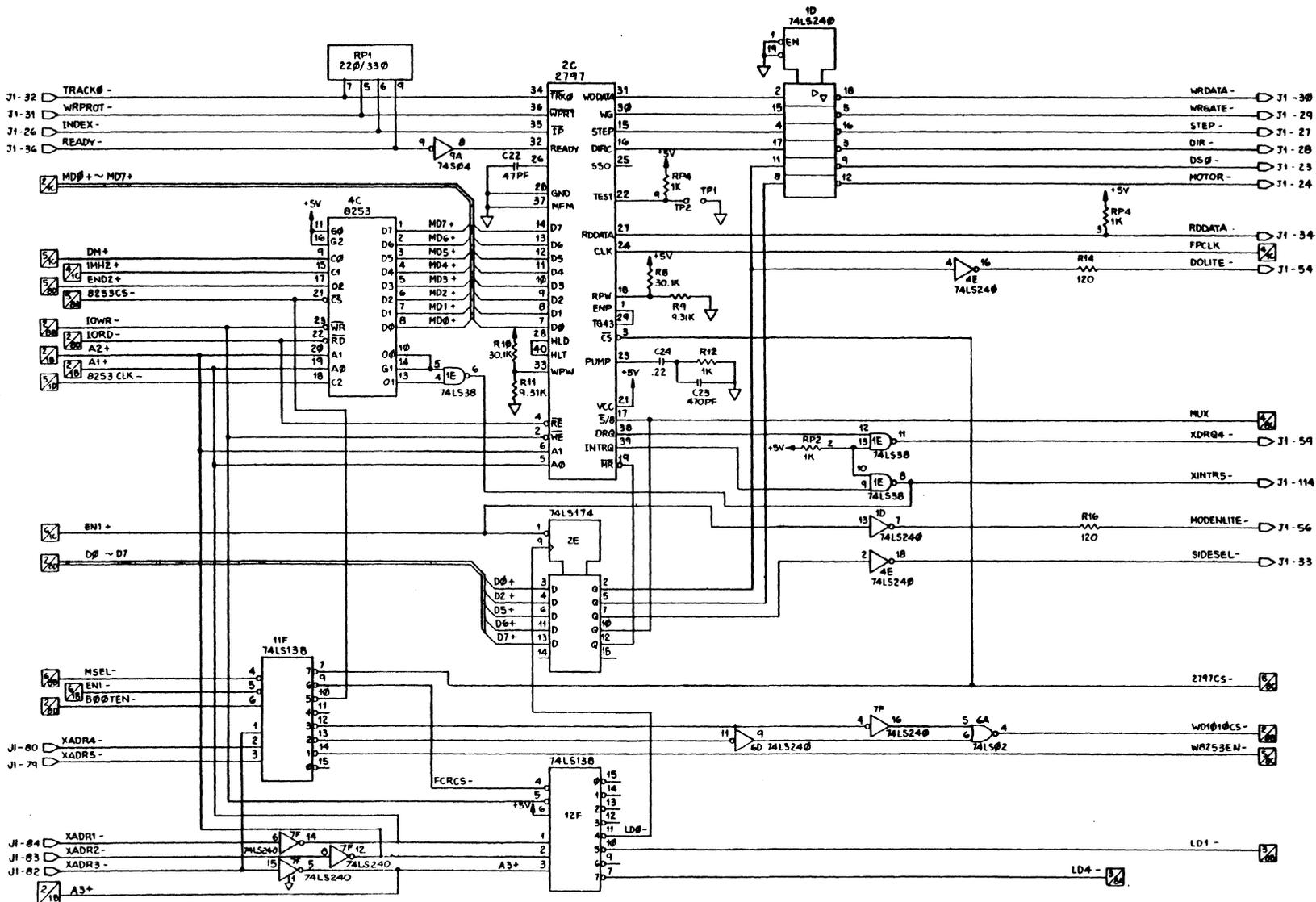
Figure 3-1. Floppy/Hard Disk Module Schematic Diagram. (Page 7 of 7)
