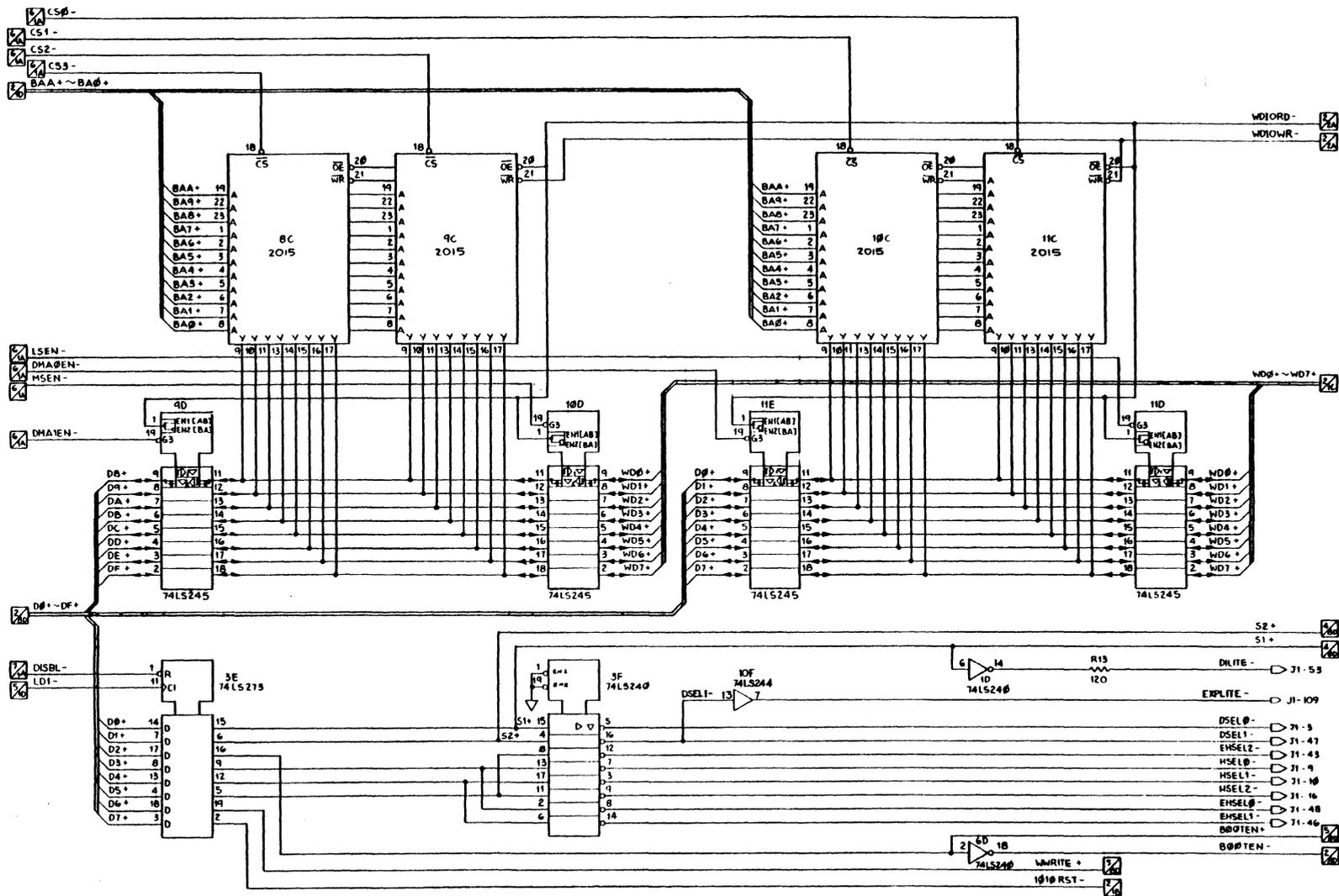
Figure 3-1. Floppy/Hard Disk Module Schematic Diagram. (Page 3 of 7)
