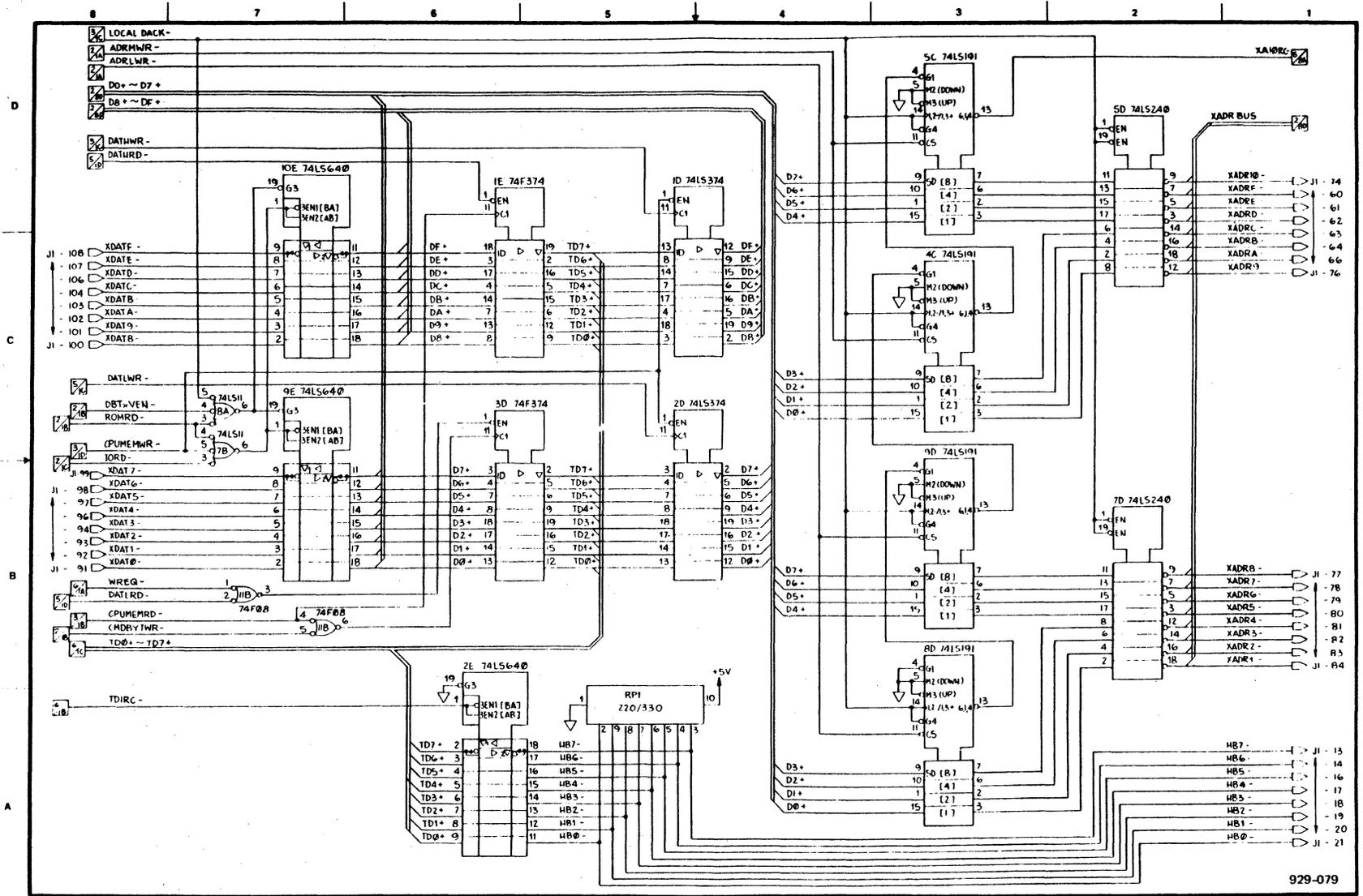
Figure B-1. Tape Control Board Schematic Diagram (Page 4 of 6)
