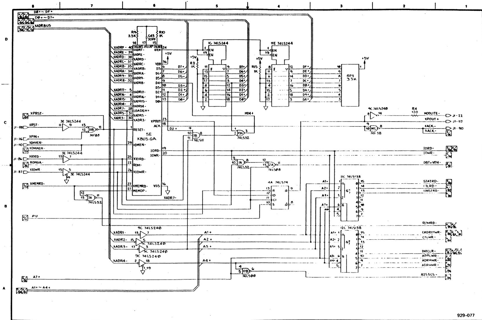
Figure B-1. Tape Control Board Schematic Diagram (Page 2 of 6)
