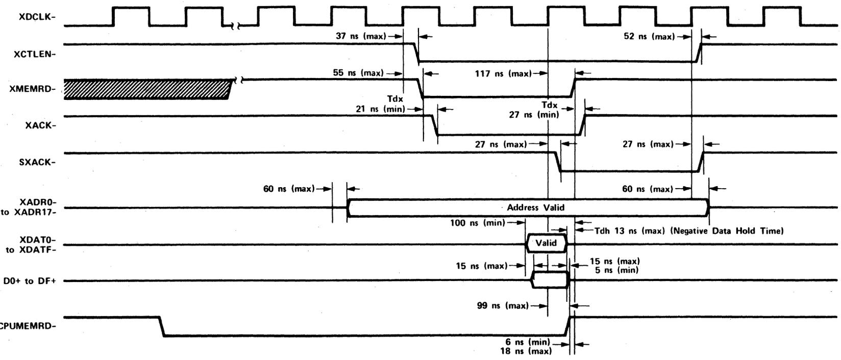
Figure 3-4. Mode 3 DMA Memory Read Timing Diagram (Page 2 of 2)
