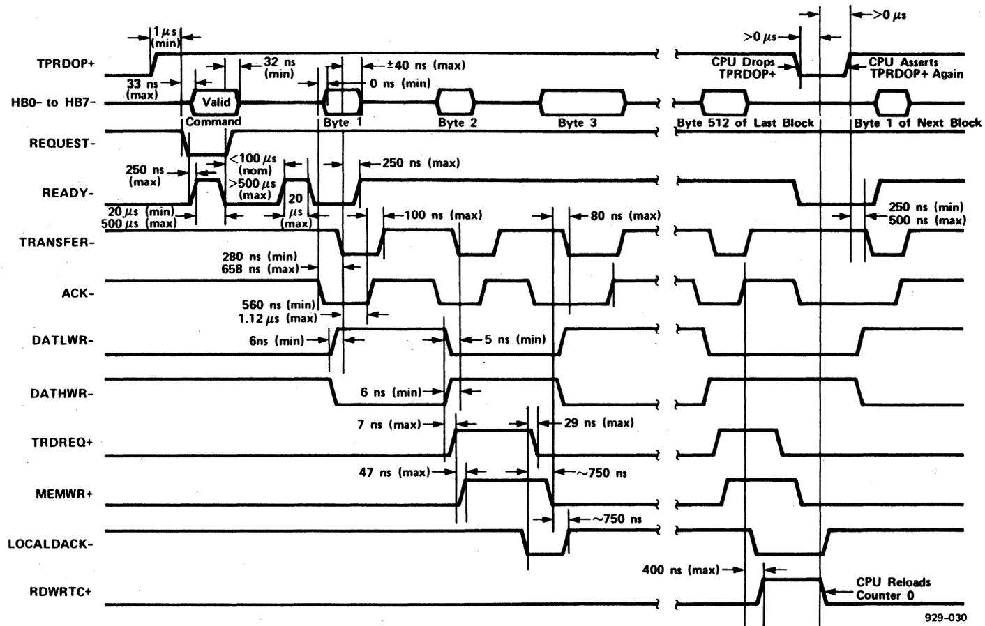
Figure 3-2. Read Tape Data Command Timing Diagram
