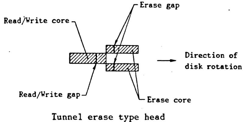
Fig. 302 External Appearance of Magnetic Head Core
