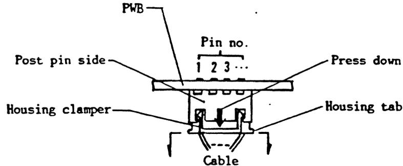
Fig. 401 Removing White Connectors (J4, J5)
