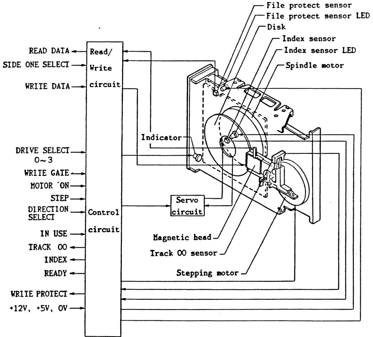
Fig. 301 Overall Block Diagram
