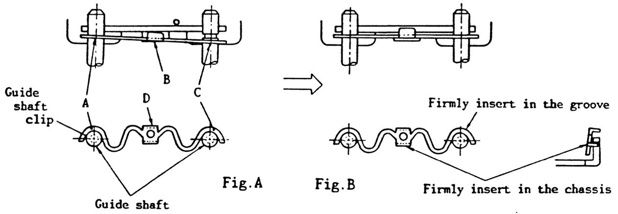
**Fig. 422-2 Guide Shaft Clips Attaching**
