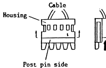
Fig. 402 Removing White Connectors (J3, J6)
