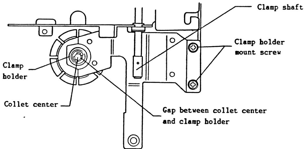
Fig. 406-c Gap between the clamp holder and collet center
