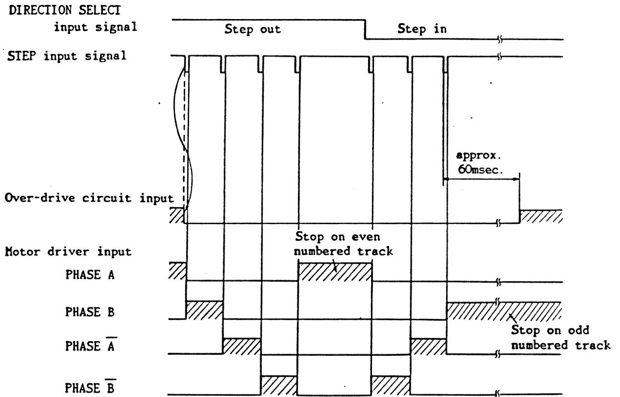
**Fig. 307-2 Typical Stepping Motor Control Circuit Operation Waveforms
