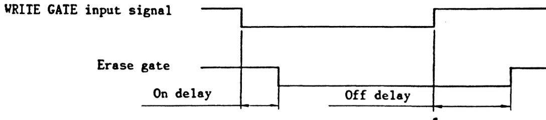
Fig. 310 Typical Waveforms
