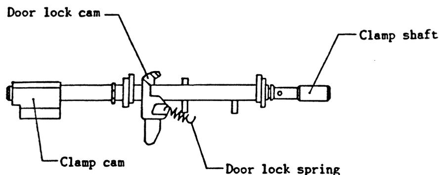
Fig. 423 Clamp Cam Assembly Replacement
