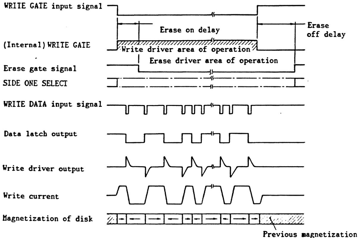
Fig. 305 Typical Write Circuit Operating Waveforms
