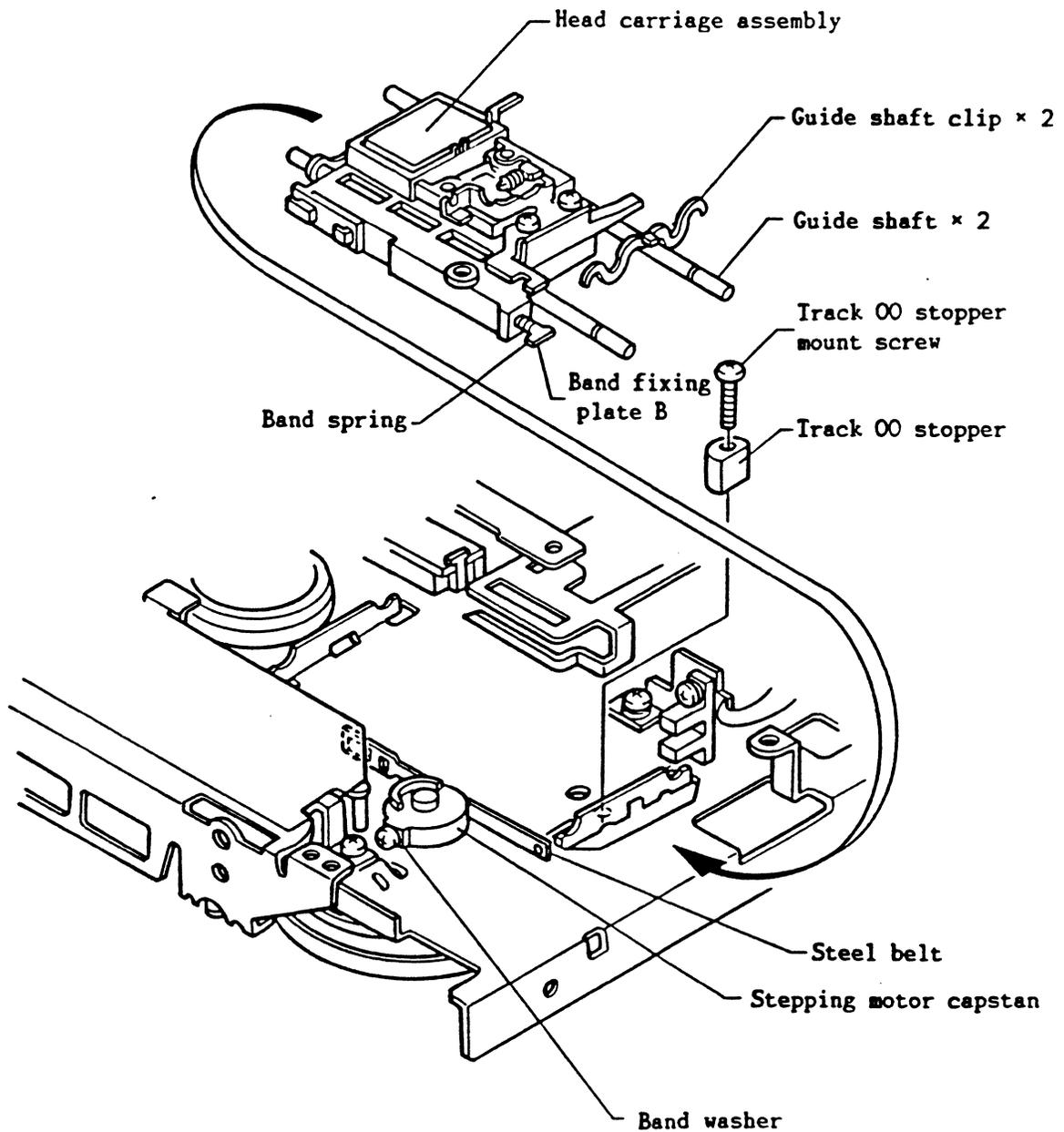
Fig. 422-1 Head Carriage Assembly Replacement
