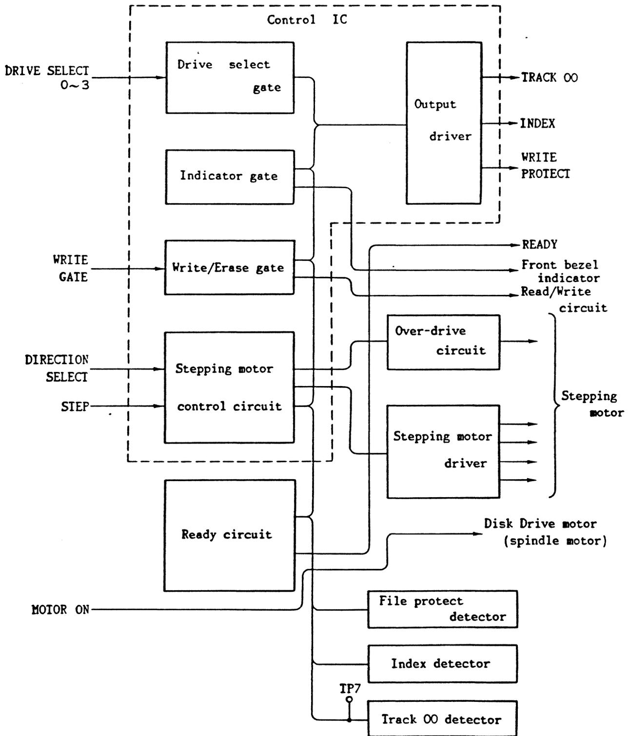
Fig. 306 Control Circuit Block Diagram
