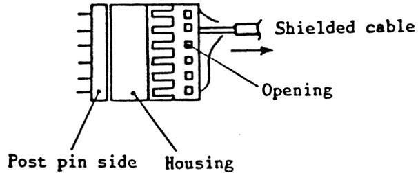
Fig. 403 Removing J7 (head connector)
