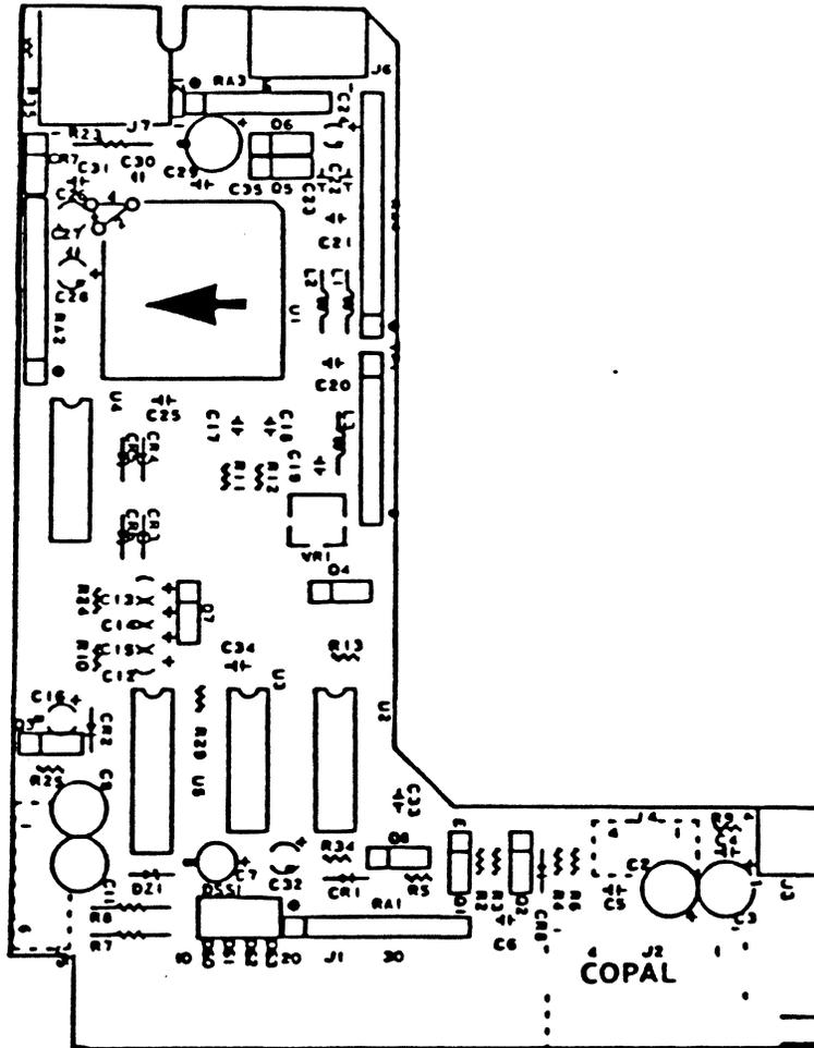
Fig. 506 Main PWB, Parts Location
