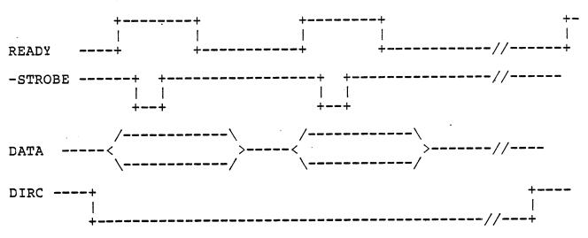
The drive starts a computer read sequence by lowering the DIRC line. The drive then puts a byte to the data lines and raises the ready line. The computer then pulses the -STROBE line, capturing the data on the rising edge. The drive then lowers the READY line until the next data byte is ready to send. After the last byte is transferred, the drive raises the DIRC line prior to raising the READY line.
