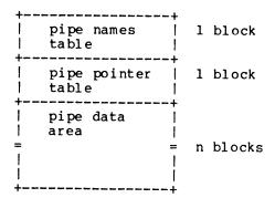
The pipe names table contains 64 entries of 8 bytes each. The first and last names in the table are reserved for system use. The first name is "WOOFW00F" and the last name is "F00WFOOW".
