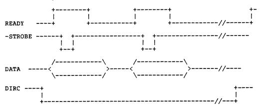
The drive starts a computer read sequence by lowering the DIRC line. The drive then puts a byte to the data lines and raises the ready line. The computer then pulses the -STROBE line, capturing the data on the rising edge. The drive then lowers the READY line until the next data byte is ready to send. After the last byte is transferred, the drive raises the DIRC line prior to raising the READY line.
