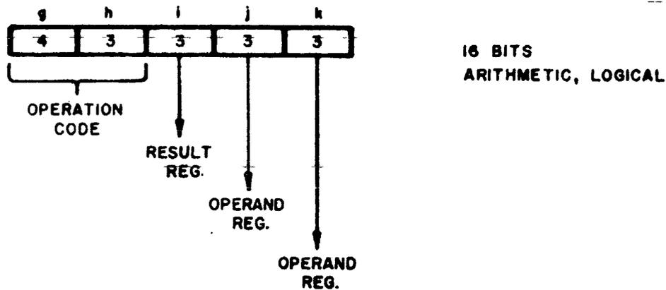
Figure 4-2. Format for arithmetic and logical instructions
