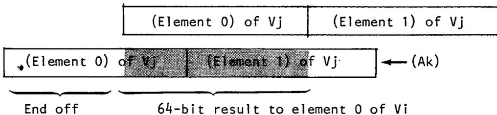
If ( $VL$ ) were 1, element 0 would have been joined with 64 bits of zero and only the one operation would be performed. If ( $VL$ ) > 2, the operation continues by joining element 1 with element 2 and transmitting the 64-bit result to element 1 of  $V_i$ . This is illustrated as follows:
