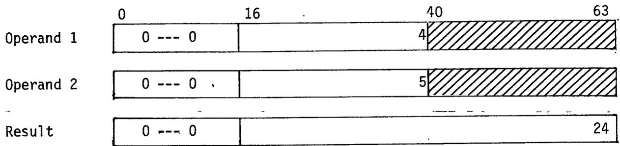
Floating point reciprocal approximation unit - For the floating point reciprocal approximation unit, an incoming operand with an exponent less than or equal to  $20001_8$  or greater than or equal to  $60000_8$  causes a floating point range error. The error flag is set and an exponent of  $60000_8$  is sent to the result register along with the computed coefficient.
