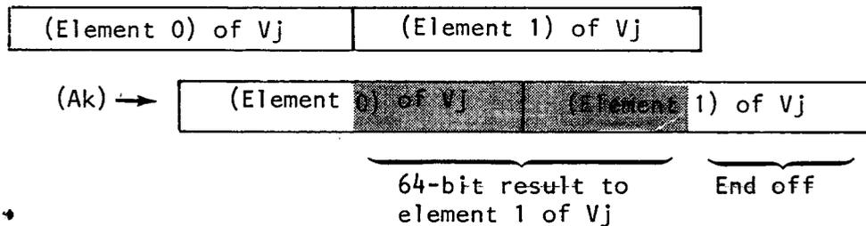
The last operation performed by the instruction joins the last element of  $V_j$  as determined by  $(VL)$  with the preceding element. The following figure illustrates this operation.
