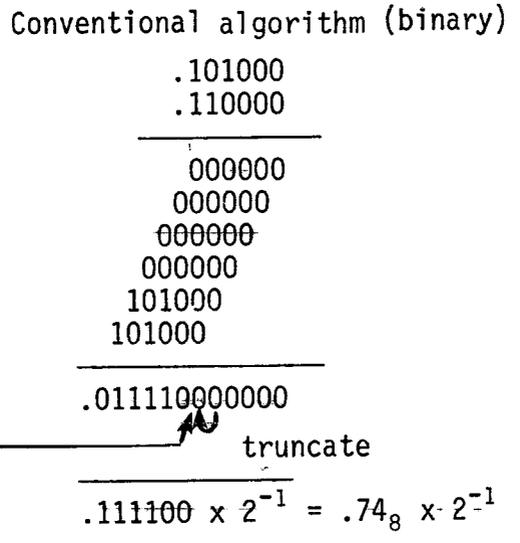
CASE 2 - CRAY-1 ALGORITHM ROUNDS CORRECTLY AND IS COMMUTATIVE
