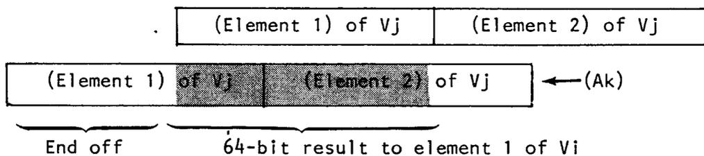
If (VL) were 2, however, element 1 would have been joined with 64 bits of zero and only two operations would be performed. Thus, the last element of  $V_j$  as determined by (VL) is joined with 64 bits of zeros. The following figure illustrates this operation.
