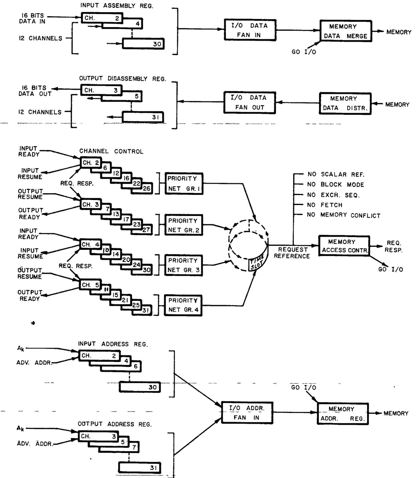
Figure 6-2. Channel I/O control
