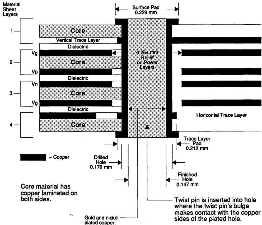
Table 11 describes the layers in a circuit board by showing what each layer is used for as well listing the specifications of each layer.
