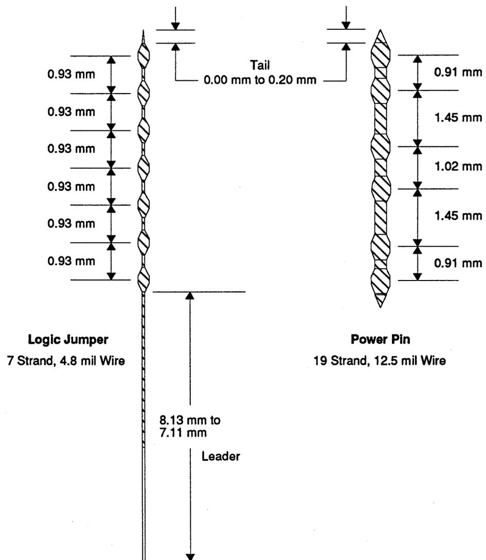
Both the twist pins used for logic jumpers and the twist pins used for power pins are made using Hughes Twist Pin machines. The beryllium-copper wire is
