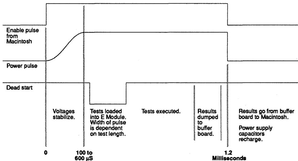
When the test results have been received by the buffer board, a signal is sent to the Macintosh to turn off the power supply pulse. The results of the tests are then sent back to the Macintosh to be displayed on the monitor for the test person to examine. The process is started again after a pause time calculated by the duty cycle previously selected. Figure 127 illustrates these timing relationships.
