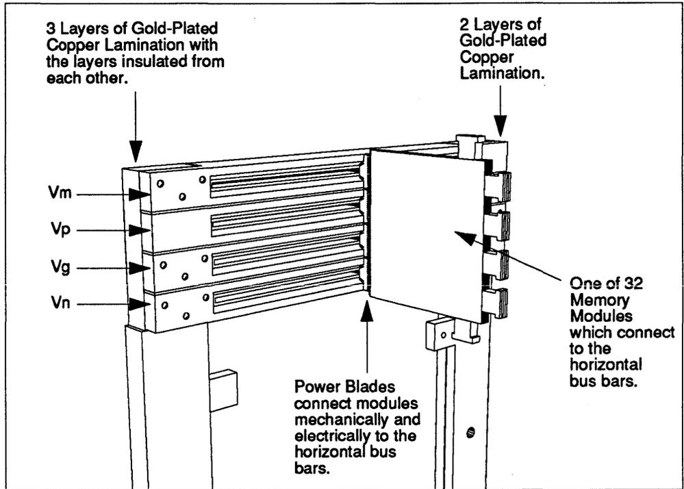
**FIGURE 142. Horizontal Power Buses for the Memory Modules.**
