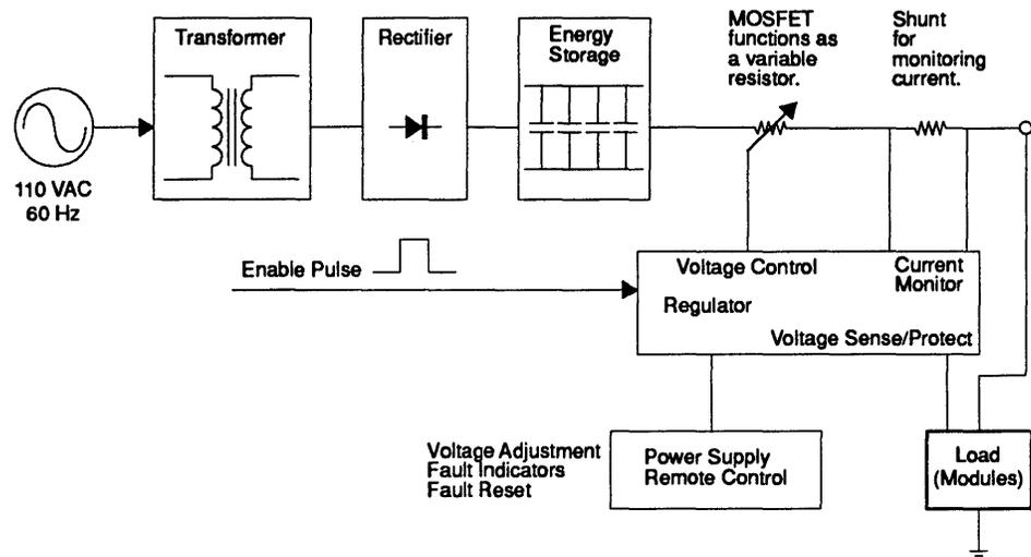
The voltages are regulated and can be adjusted individually from a remote control box. This allows the CRAY-3 modules under test to be tested at voltages different from their ideal voltage in order to find their operating margins. The voltages can be checked by probing a module power pin with an Oscilloscope or by reading the listed voltages in a window on the test station Macintosh monitor.
