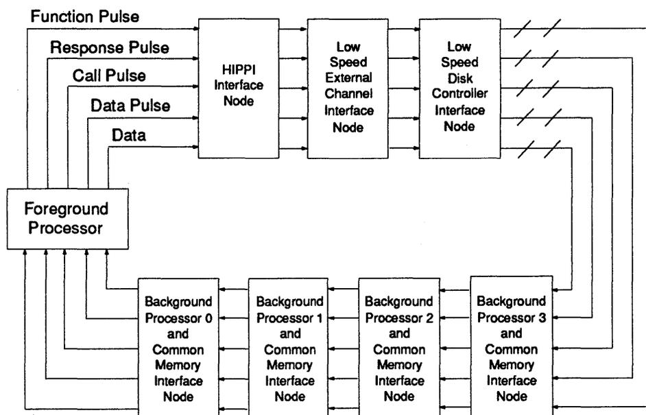
The primary function of the Foreground Processor program is to poll the four communication channel loops for requests from the Background Processors and control the communications on the four channel loops to facilitate data transfers between controllers on the channels. Many of the requests that will be recognized by the Foreground Processor require responses within a microsecond or less.
