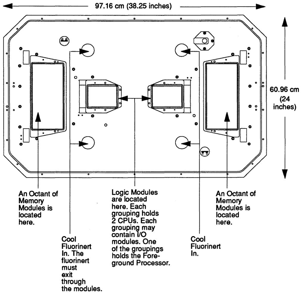
**FIGURE 136. Top Plate for an Eight-Processor CRAY-3.**
