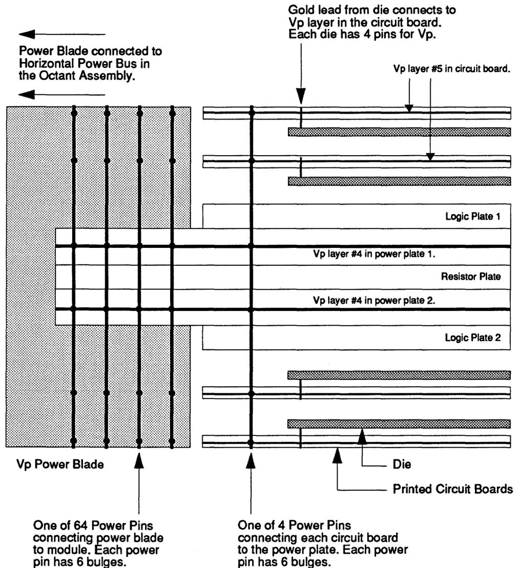
The distribution of power and ground throughout a module begins at the power blades. The power blades receive power from the power supplies through their attachment to the horizontal power bus. The blades transfer power to the power plates where the electrical power is distributed to all of the power pins located
