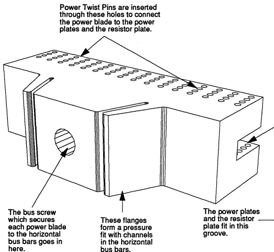
The module power blade is tapered and is forced into a rectangular slot in the horizontal bus bar by a screw. Each insertion of the module results in a sliding
