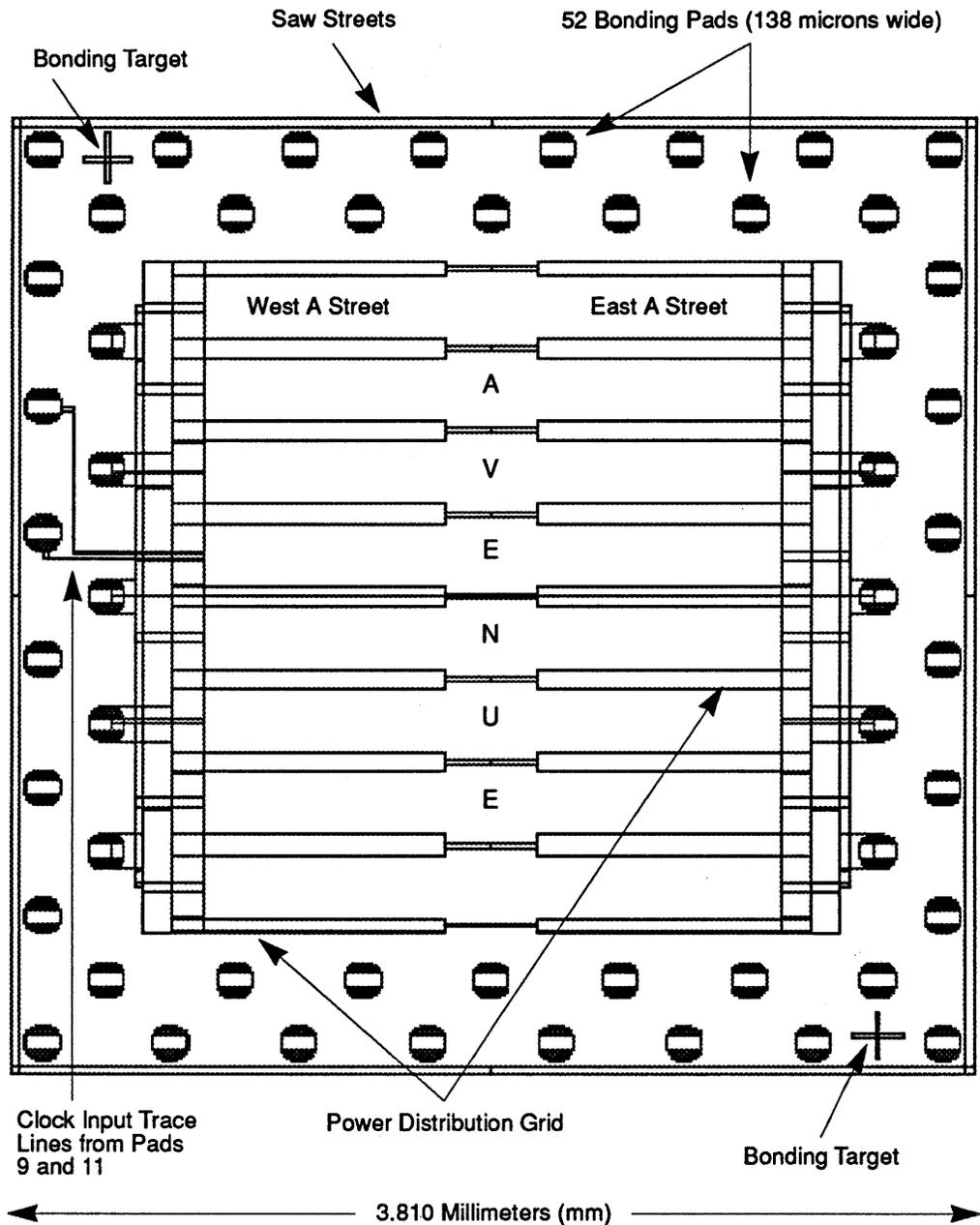
There are eight streets and one avenue in each generic IC assembly. The avenue runs north and south down the center of the IC, so each of the eight streets are divided into a west side and an east side (see Figure 56). Each half of each street has four cell positions on the north side of the street and four cell
