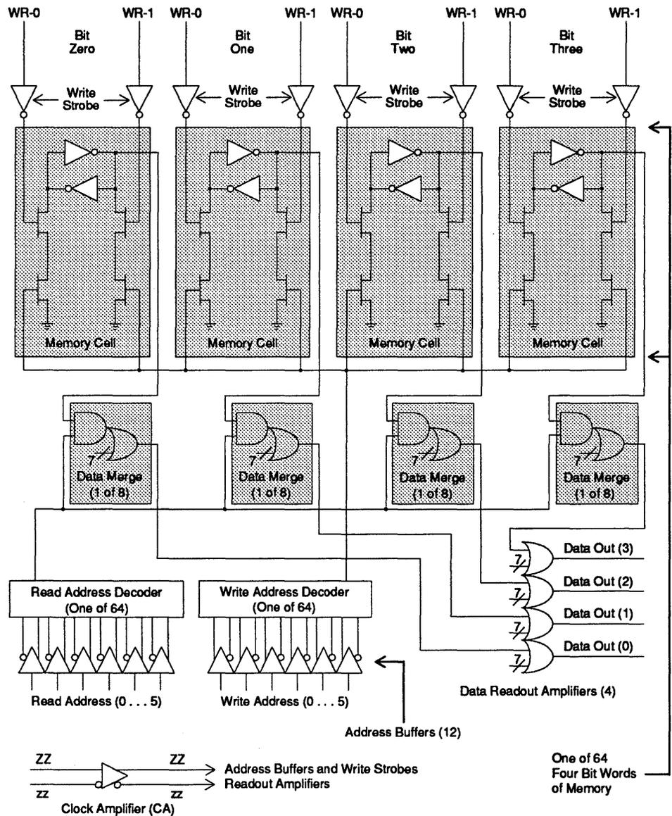
The VR package contains a 256-bit memory with a 64 element address and four data bits. Six address bits are delivered to the package for readout
