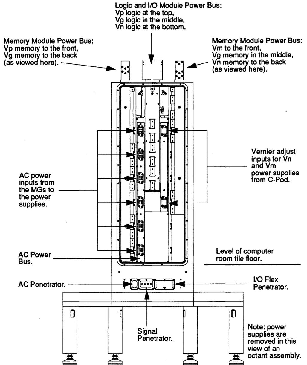
**FIGURE 141. Horizontal Power Buses for Memory from Module Side.**
