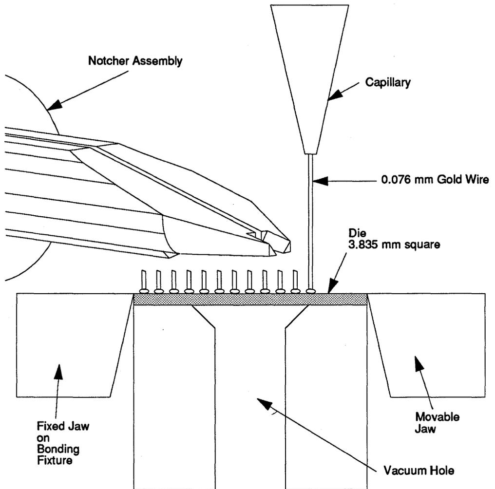
**FIGURE 91. Gold Leads Bonded to a Portion of a Die.**
