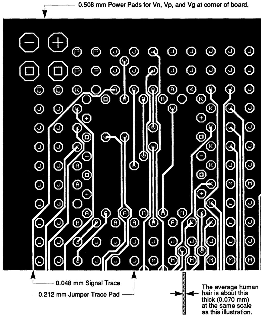
Figure 98 gives a view of one of the inside trace layers of a circuit board. These trace lines are drawn in the Artwork Department using CrayDraw. The circuit
