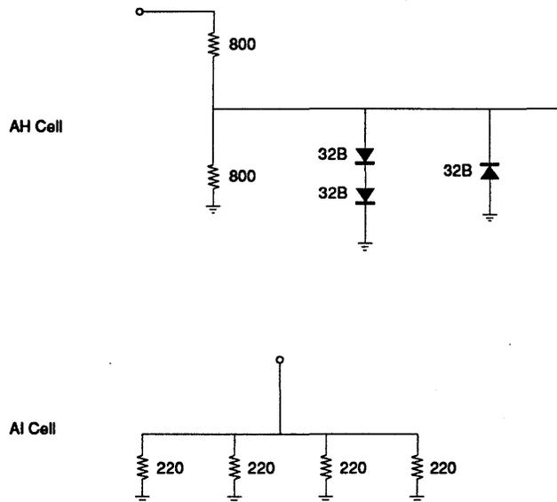
The two 800 ohm resistors divide the voltage in half when the input voltage is 3.0 to 1.5 volts. This produces a 1.0 volt output to the logic cells when 2.0 volts is at the input with only 1.25 mA. The 32B diodes-to-ground provide voltage clamping for protection.
