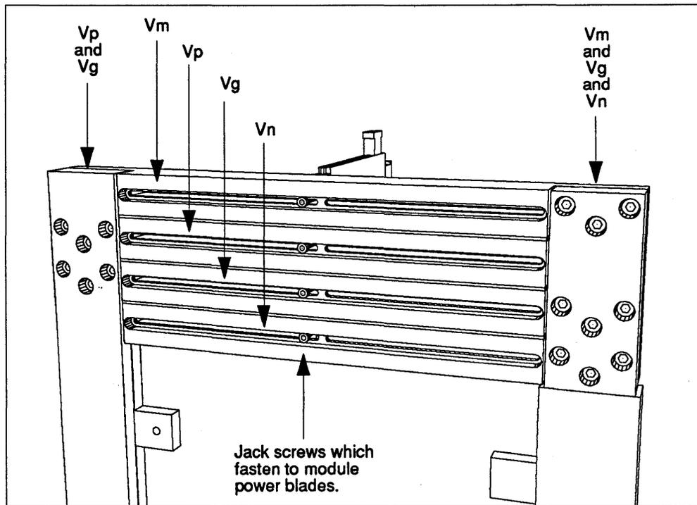
**FIGURE 143. Horizontal Power Buses for Logic Modules from Module Side.**
