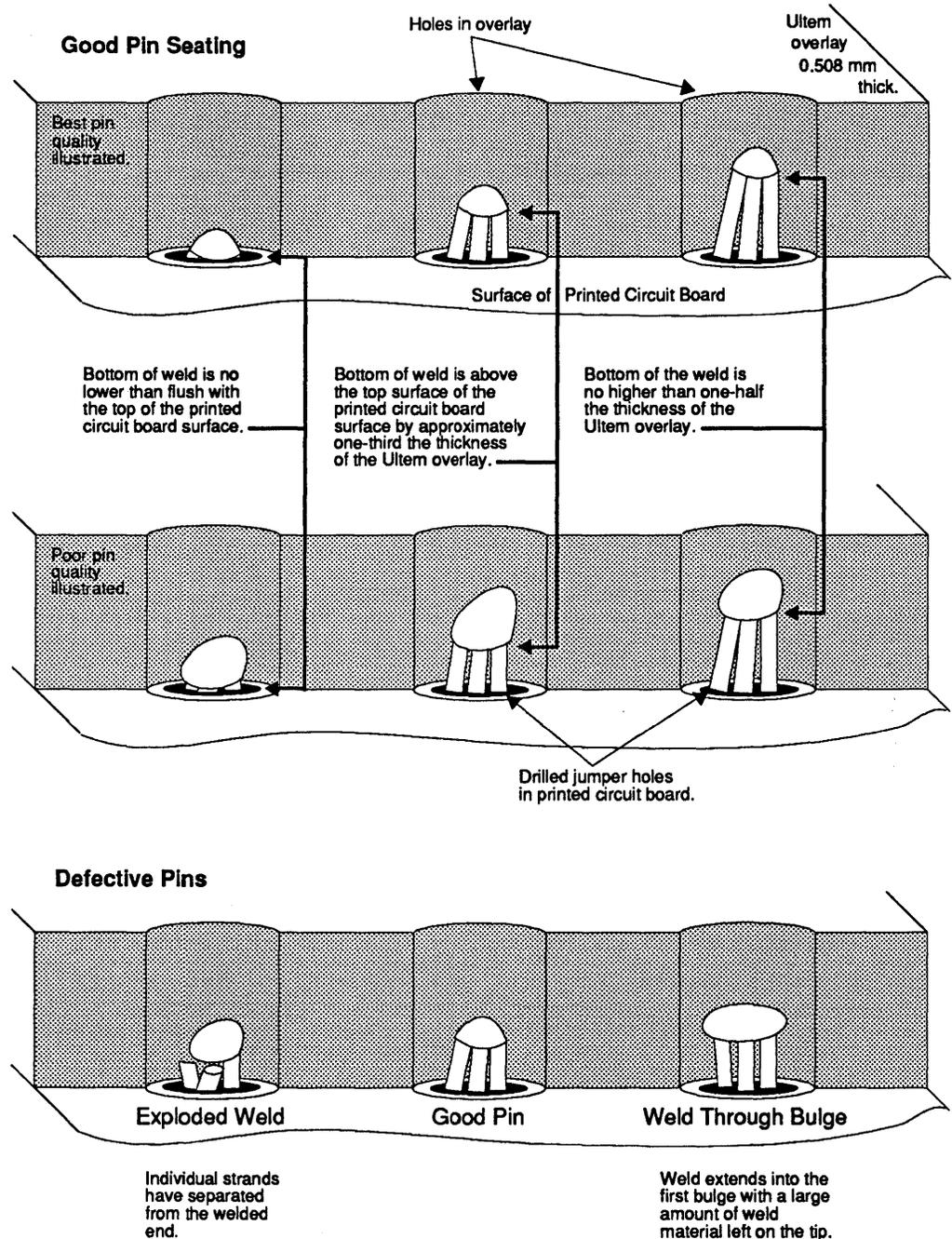
Using a tweezer, the operator inserts a twist pin, leader end first, into the hole as deep as the first bulge. The leader protrudes below the module by about 1.52 mm. When the operator has properly inserted the twist pin, a foot switch is depressed and the puller-cutter cycle begins.
