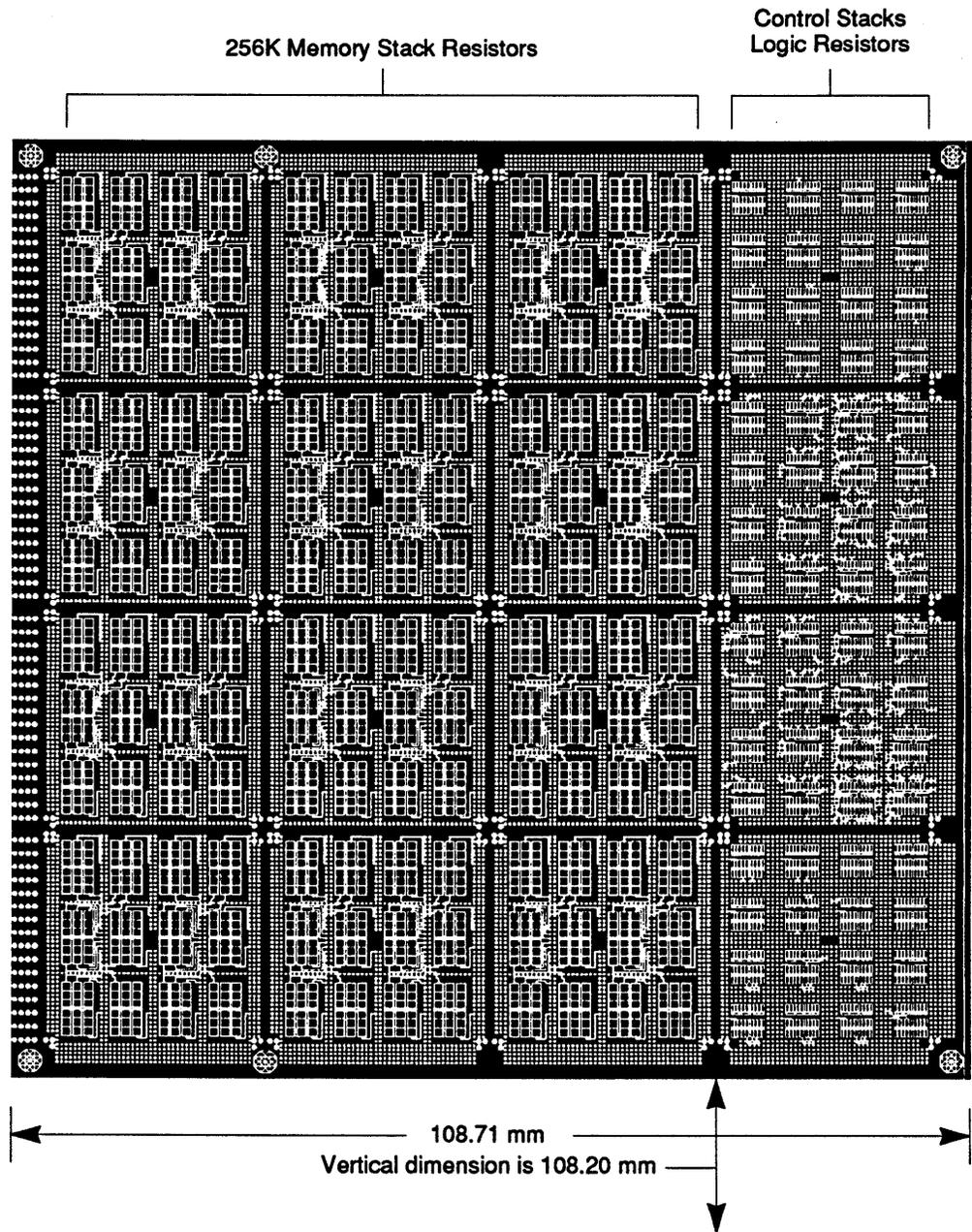
**FIGURE 104. Resistors on a Logic Module Resistor Plate.**
