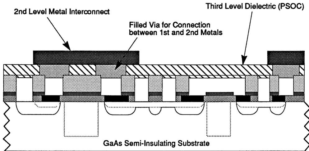
The eighth step in the process is the addition of second level metal (see Figure 86). This metal is also electron beam evaporated onto the wafer. The metal which is used consists of titanium and then gold. This metal layer is thick and requires a special retro-grade photoresist profile for the subsequent metal lift-off process. Again, the unwanted metal is removed by the lift-off process.
