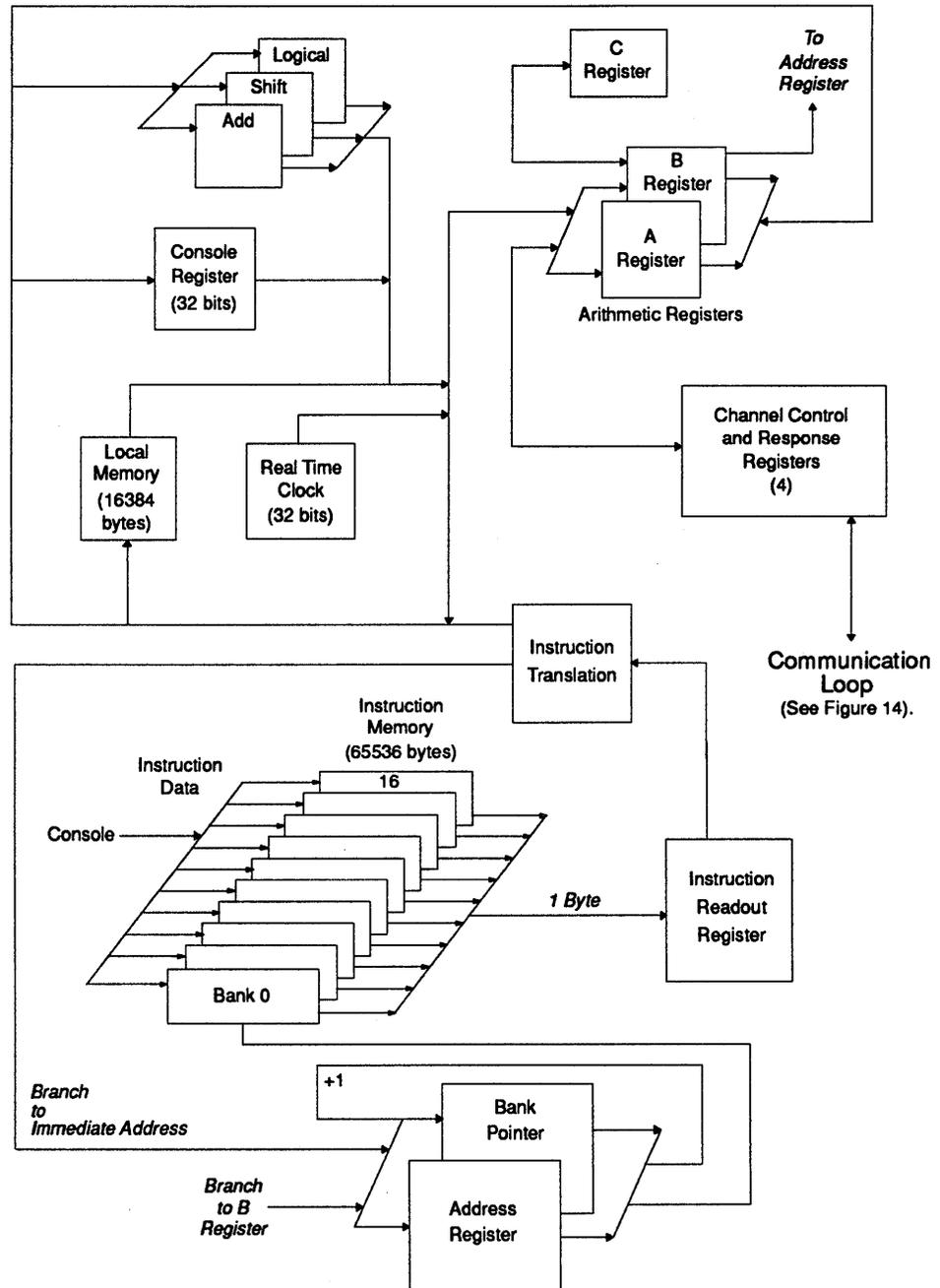
The Foreground Processor is divided into seven operational sections: 1) deadstart circuits, 2) instruction issue mechanism, 3) local data memory, 4) channel communication, 5) functional units, 6) console communications and
