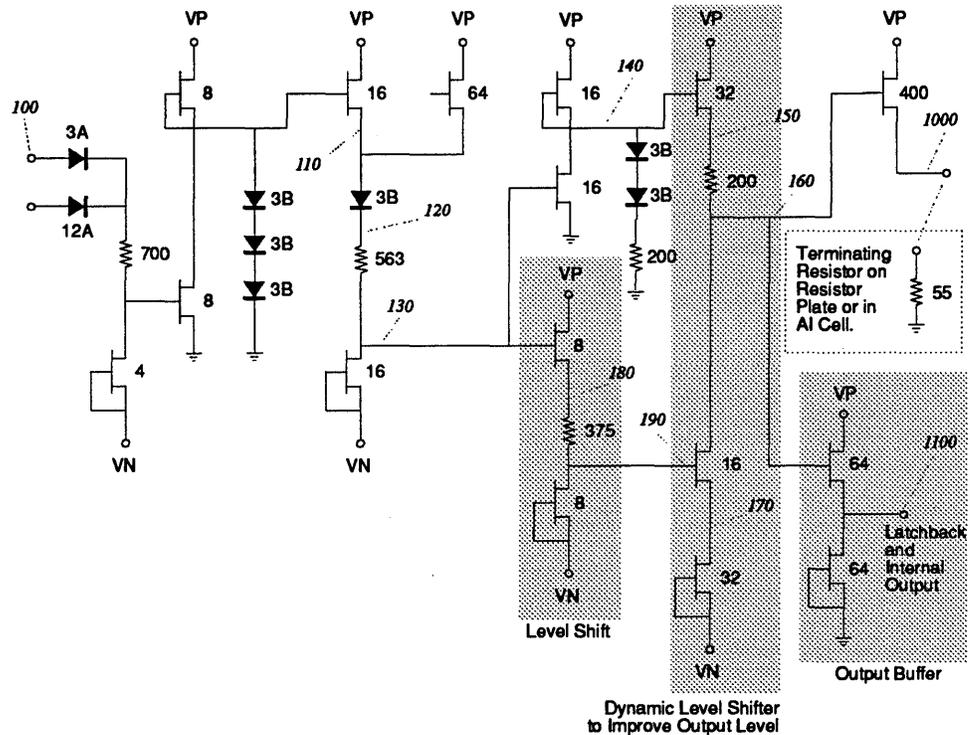
The new F cells are FAST tested (see the section on FAST testing in Chapter 5) for a Voh (voltage output high) of 1.35 volts and a Vol (voltage output low) of 0.45 volts, whereas the FA through FE series were FAST tested for a Voh of 1.30 volts and a Vol of 0.58 volts. As you can see, the greater improvement was accomplished at the lower end of the voltage swing.
