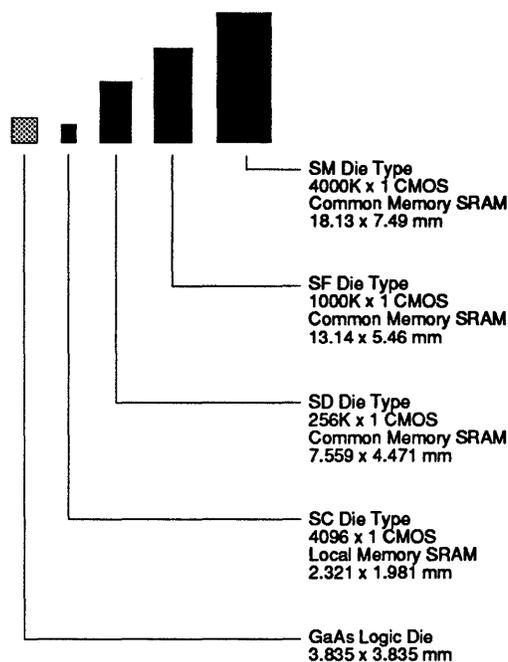
The SD die are 256K by 1 static memory circuits used for Common Memory. Four packages are used in parallel to provide 1,024K bits of memory per bit position in each Common Memory bank. The circuit has a 34 nanosecond write cycle and a 34 nanosecond read cycle. The data is sampled at 24 nanoseconds into the read cycle.
