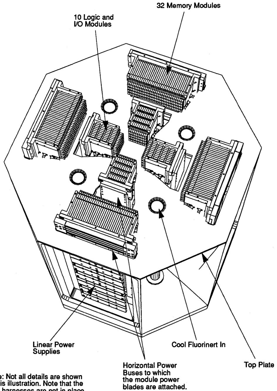
**FIGURE 138. Top Plate for a Prototype One- or Two-Processor CRAY-3.**
