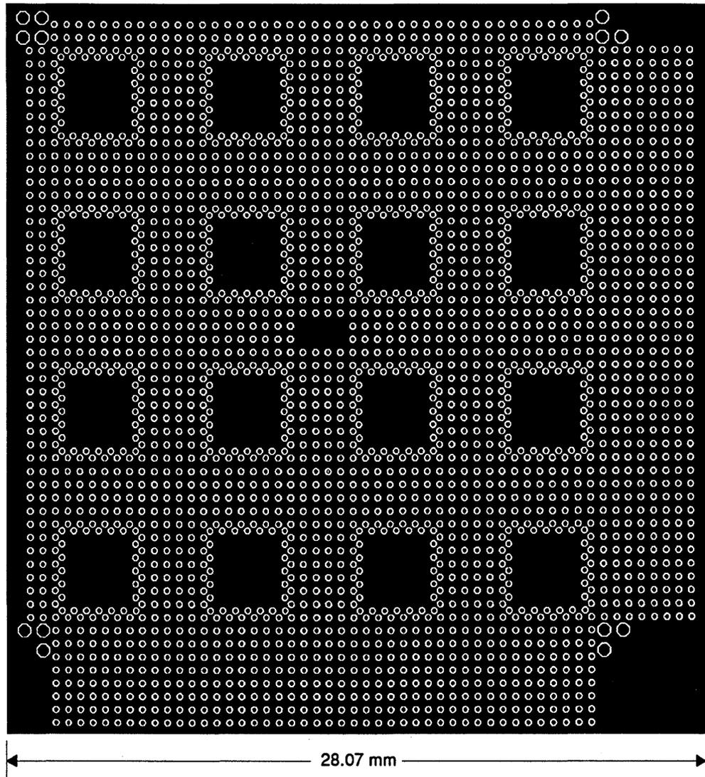
The holes for the gold leads from the die can be seen directly around the square areas empty of any jumper holes. Since the board shown in Figure 97 mounts at the corner of a module this P stack logic board has wirebond jumper holes
