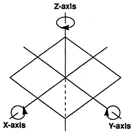
All of these factors added together results in a single  $180^\circ$  rotation about the Y-axis prior to the data being fractured. This is easily accomplished with the Fracture program. The program has a default setting that requests a  $180^\circ$  rotation about the Y-axis.
