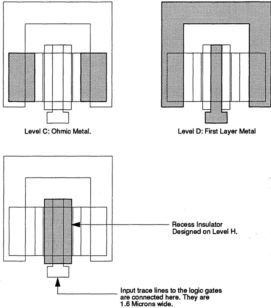
A type B diode with a 4.0 square micron diode contact area is illustrated in Figure 25. These dimensions are considerably more relaxed than the dimensions for the type A diode. The anode finger for this configuration is the right metal path in the drawing for level D. The cathode is the left metal path. The area of the diode in this configuration is 4.0 microns by 1.0 micron.
