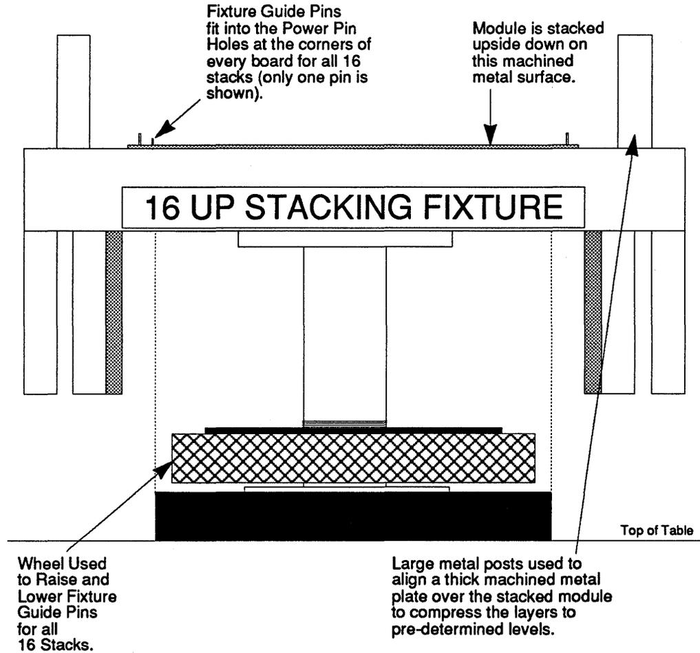
Once all layers of the module have been stacked, the fixture guide pins can be retracted leaving the permanent guide pins, which were inserted during the stacking process (four per stack), holding the module assembly together.
