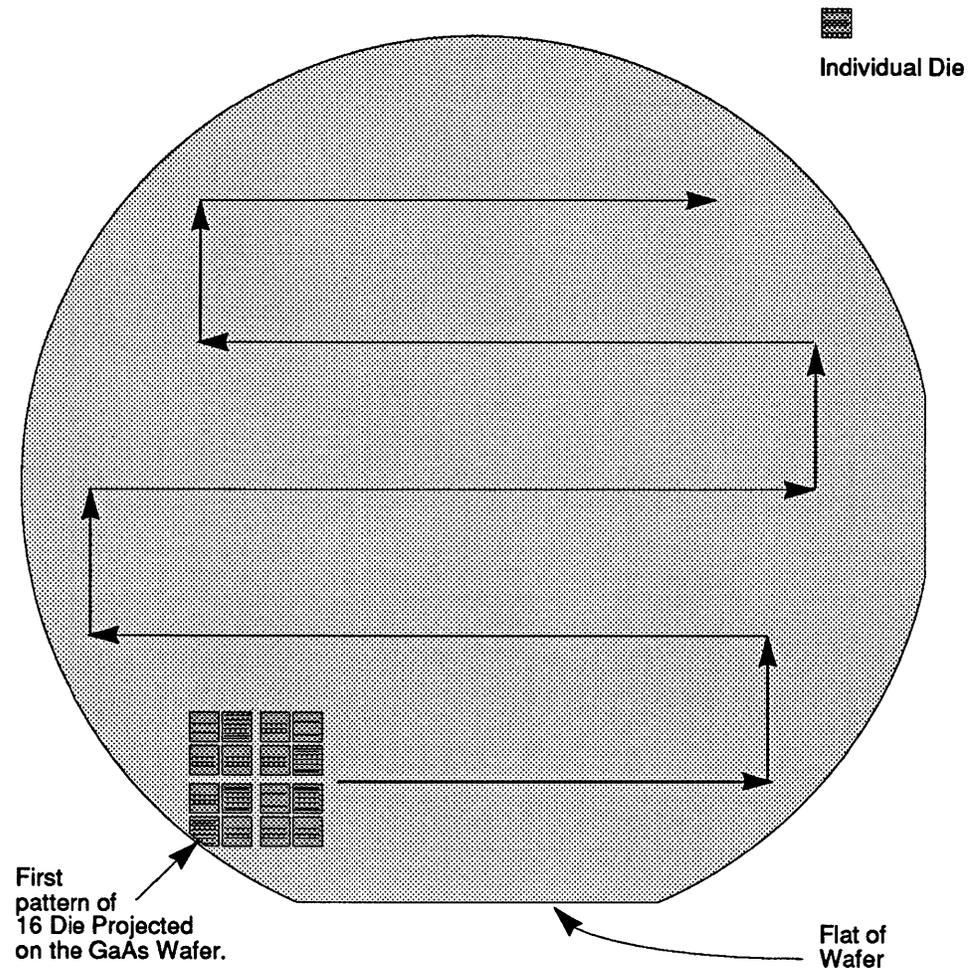
The Canon photolithography machine is called a wafer stepper because the pattern projected on the wafer covers only a small portion of the available wafer surface (see Figures 80 and 81). The wafer is then moved, or stepped, and the pattern is repeated. Each reticle may contain the layout for 4, 8 or 16
