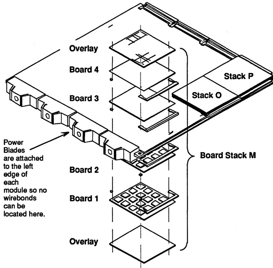
The module's basic mechanical integrity is provided by the 104 mm circuit boards or plates at the center of the module sandwich. The smaller boards, and hence the stacks, are attached to the plates with power and alignment pins, as well as the complement of twist pin logic jumpers used on each board stack.
