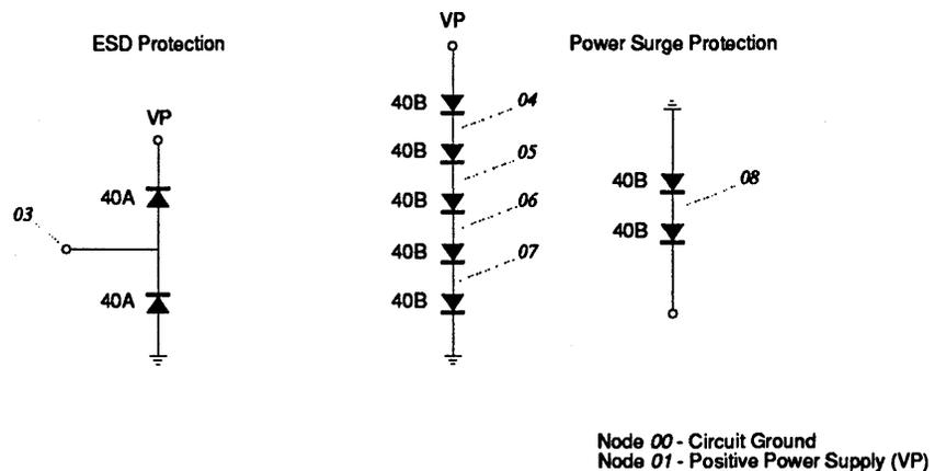
The ESD diodes are connected to all inputs of the GaAs die. This allows voltage excursions 0.7 volt higher than  $V_p$  and 0.7 volt lower than  $V_g$  to be shunted away from the inputs. This voltage excursion, if received by the input structures of the logic cells, could be destructive. Power surges above 3.5 volts and below -1.4 volts will be absorbed by the diode circuitry in the AF cell. The AF cell requires one cell site. It is placed in all cell sites not used by other cells.
