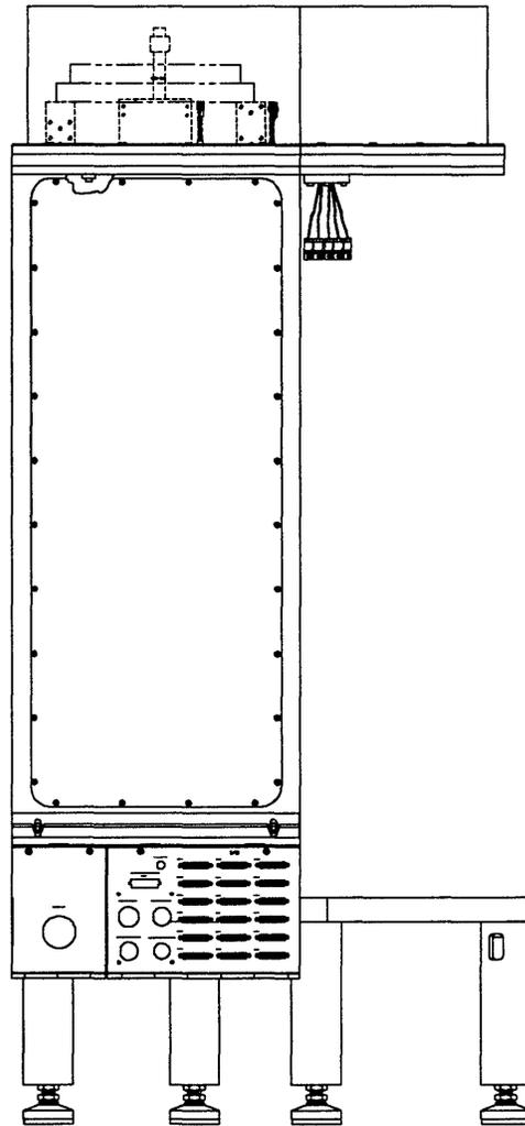
**FIGURE 133. Sub-Floor Mounting of the System Cabinet.**
