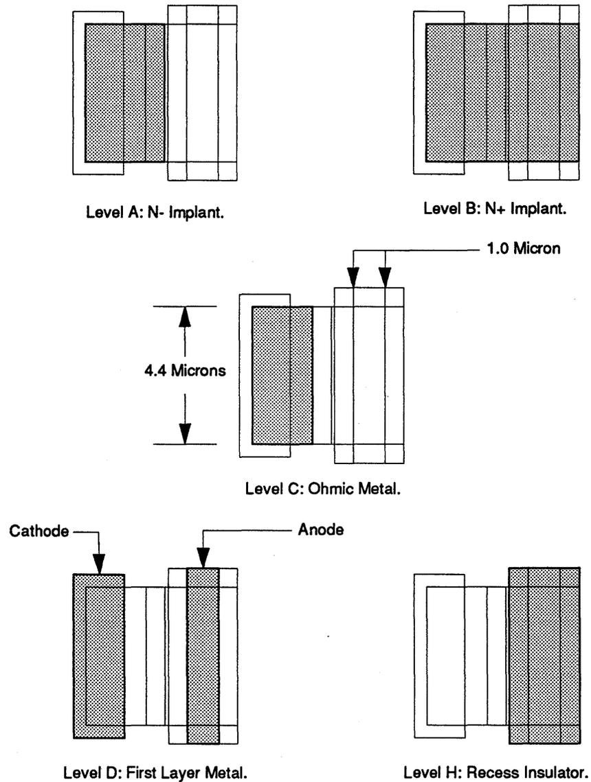
The implant areas are identical in this design as they were in the design of the type A diode. The advantage of the type B diode is the better process yield and the greater diode area in a given amount of package real estate.
