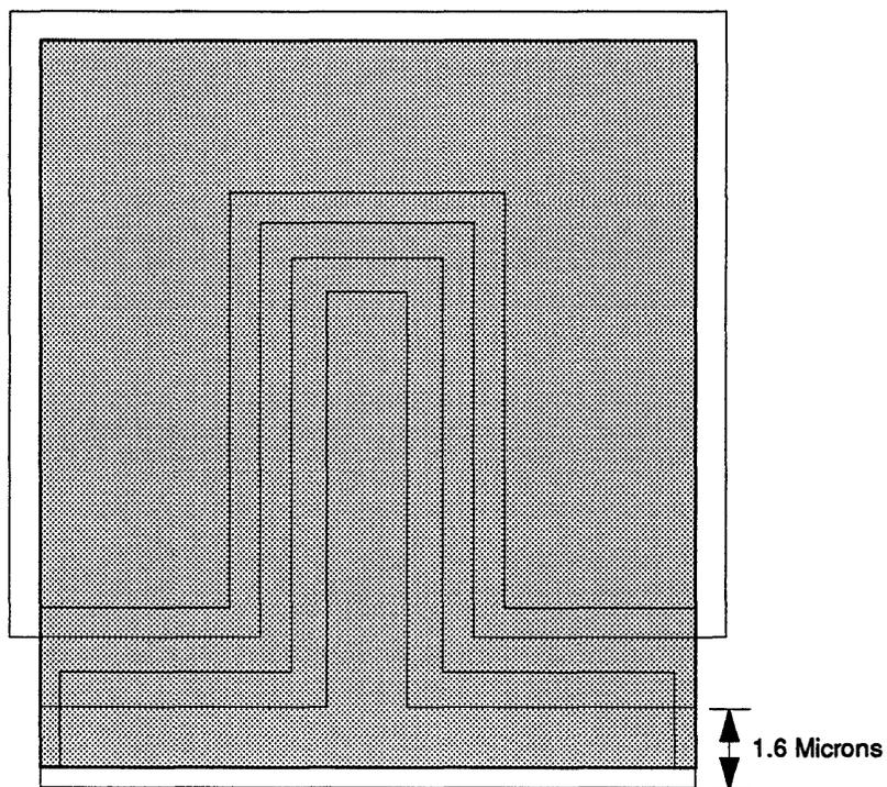
Level A (N- Implant) and Level B (N+ Implant).
