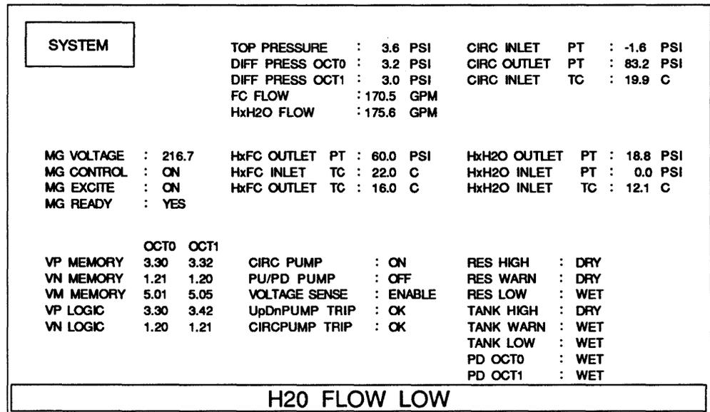
The flow meters measure the rate of flow of both the chilled water and the Fluorinert in gallons per minute. The thermocouples measure the temperature, in degrees Celsius, of the Fluorinert and the chilled water at various points throughout the system. The pressure transducers measure the pressure in
