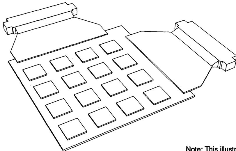
Note: This illustration shows Flex cable instead of individual twisted pair wires.
