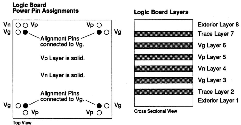
**FIGURE 110. Power Distribution in 256K Memory Modules.**
