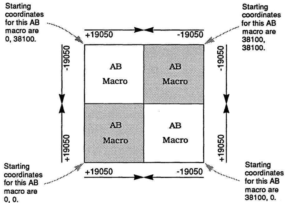
The next portion of the AA macro which we will examine is that part which calls up the AC macro (the bonding pad), placing it fifty-two times at the correct locations around the perimeter of the IC package. Only four of the fifty-two calls are shown in Figure 61.
