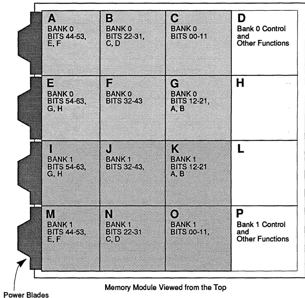
There are two memory banks on each Common Memory module. Each memory bank occupies six out of the sixteen stacks on a module. The remaining four stacks are control stacks (see Figure 11). A memory bank can utilize 16 background processor memory access ports. Total memory bandwidth is 128 gigabytes per second. Total memory capacity is eight
