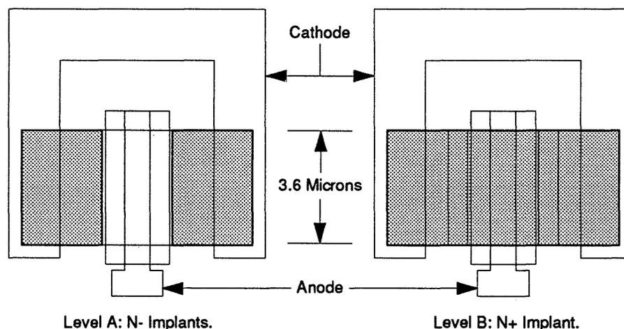
The contact area of the diode is that portion of the anode finger which is over the implant field. This is a rectangular area 0.8 microns by 3.6 microns in size. Total area is approximately 3 square microns. There is an ohmic contact on each side of the anode finger. This design is aimed at a configuration with minimum diode resistance per unit area.
