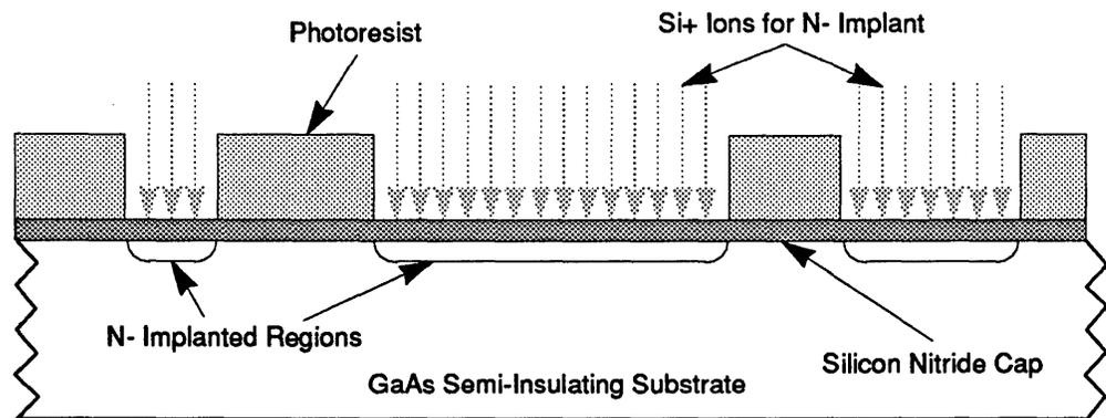
GaAs Substrate is 635 microns thick.
