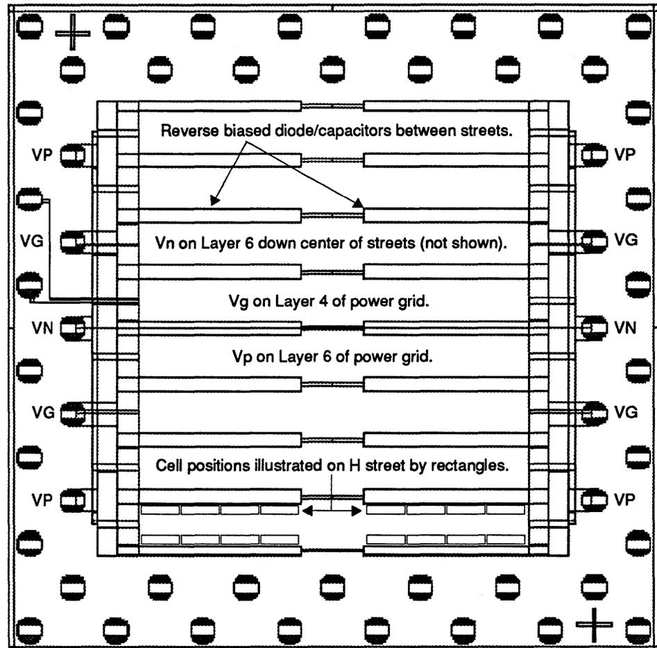
There are three power supply paths required for each cell in the IC package. The positive voltage ( $V_p$ ) has a value of +3.3 volts with respect to ground. The negative voltage ( $V_n$ ) has a value of -1.2 volts with respect to ground. The third path is the ground connection ( $V_g$ ) for the reference potential.
