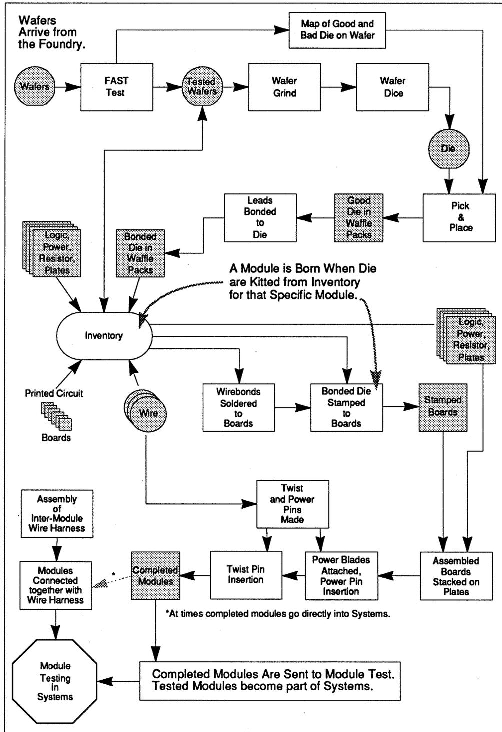
The assembly of a module takes from three to eight days, depending on the complexity of the module. The process begins by choosing the appropriate die types needed for each one of the 64 boards of that particular module and then placing those die in kits that are used by Die Attach. This first step in the assembly of a specific module is called “kitting”.
