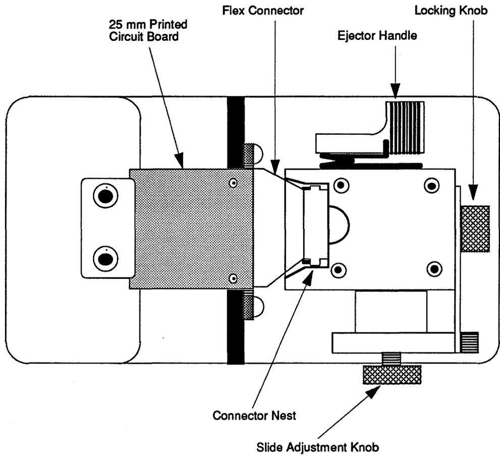
**FIGURE 118. Flex Circuits Attached to Board Wirebonds.**
