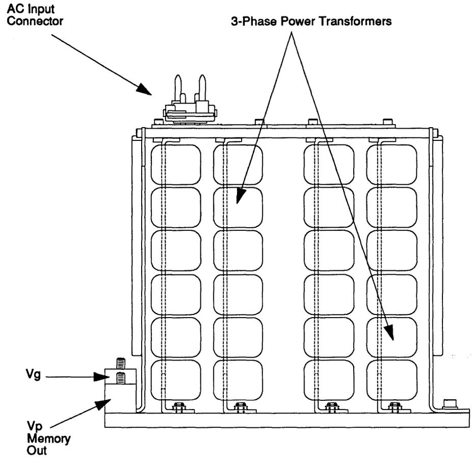
**FIGURE 148. Simplified Top View of a Vm Power Supply.**
