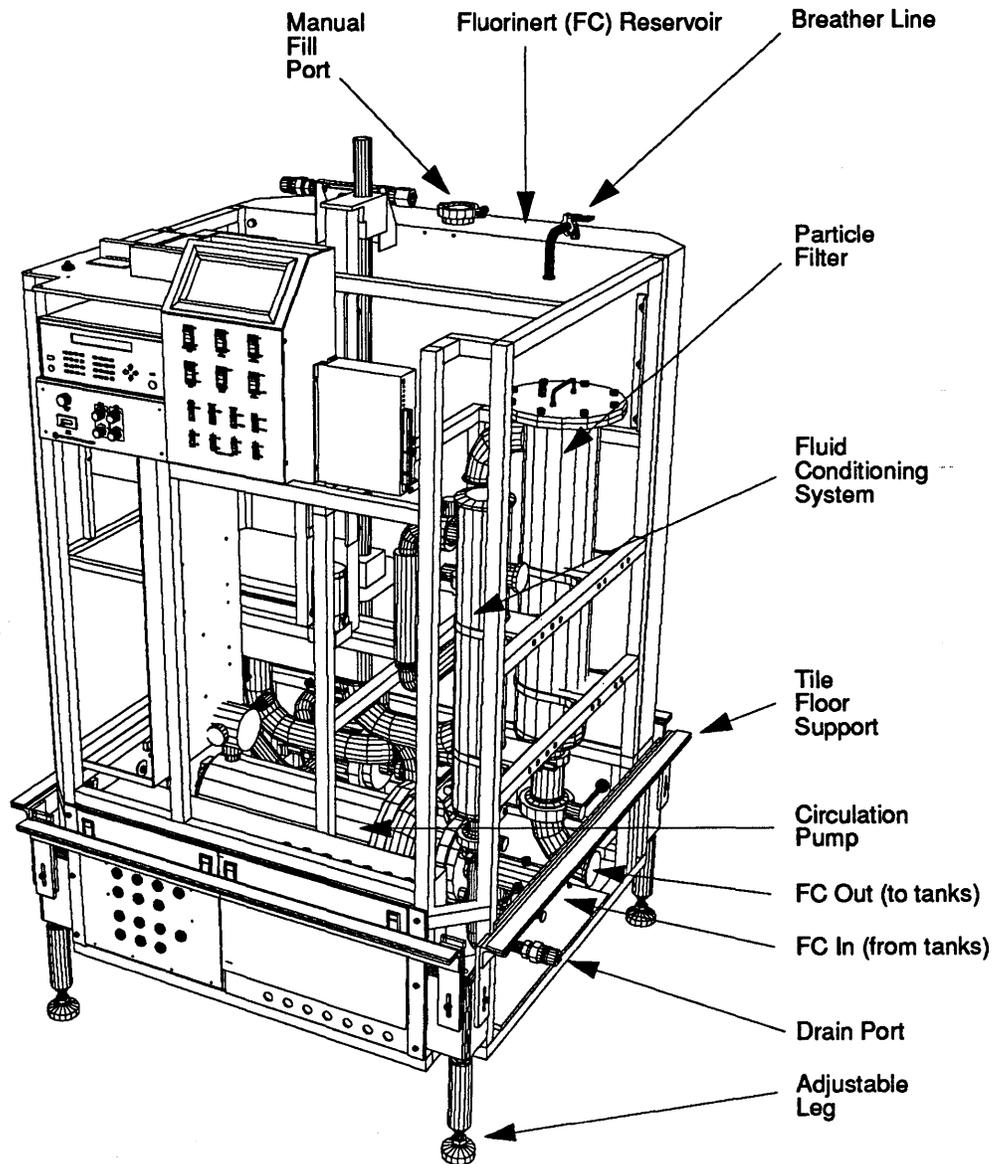
**FIGURE 154. C-Pod Cooling Components—Front Left View.**
