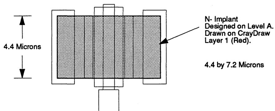
Figure 17 has the areas of N+ implant shaded. The sheet resistance of the N+ implant is approximately 400 ohms per square and the sheet resistance of the N- implant is approximately 440 ohms per square. The double implanted area essentially terminates the effective transistor channel. The N- implant continues the length of the N+ implant and overlaps it. This makes the implant under the ohmic metal as highly doped as possible.
