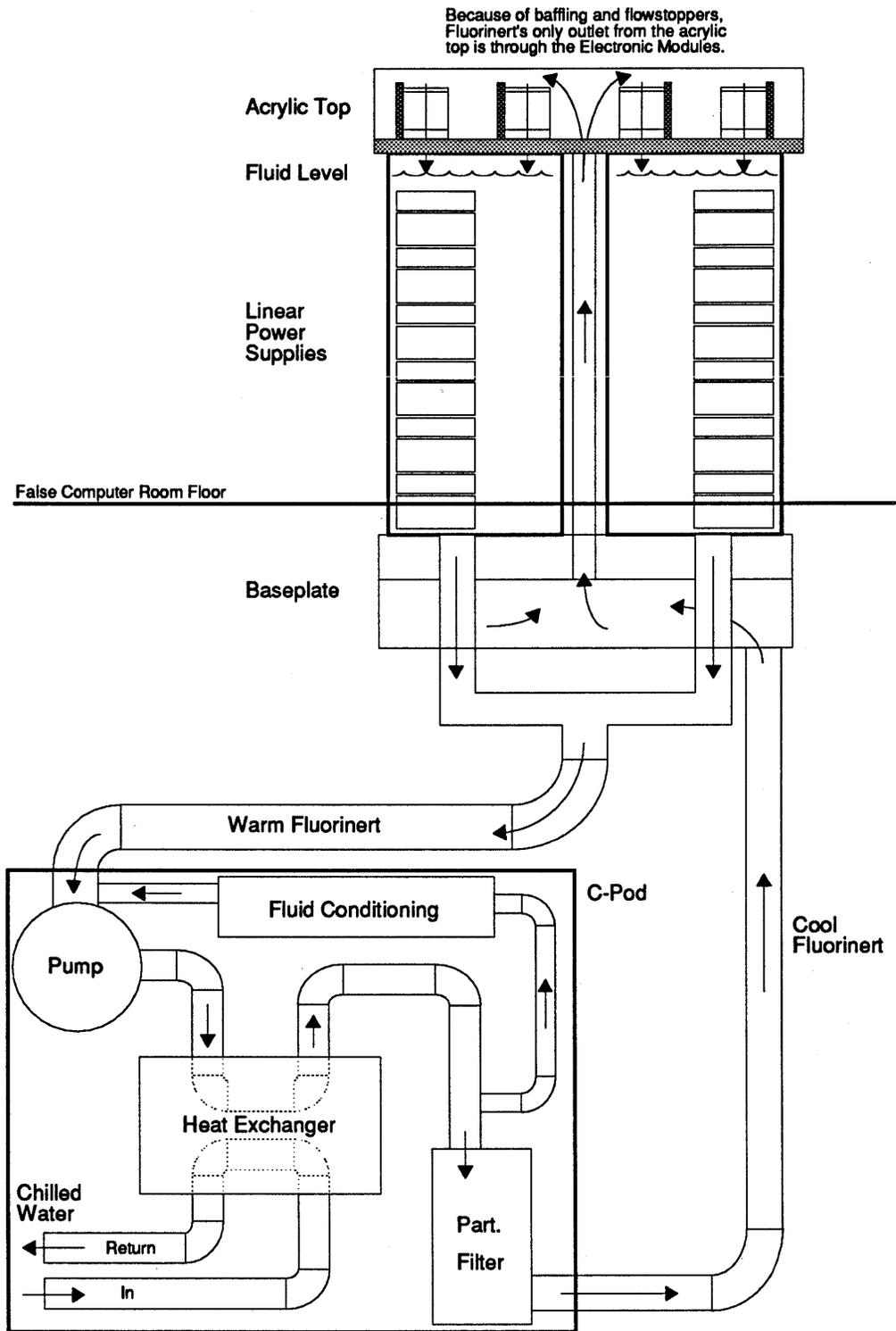
A fluid reservoir is located in the C-Pod to serve as a holding tank while servicing one of the tanks. When the system is not operating, any one or two tanks may be simultaneously emptied for servicing. The reservoir is also used to supply continual make-up fluid to the circulating loop during system operation.
