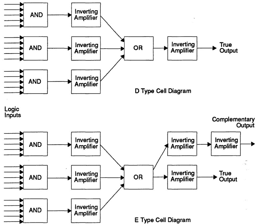
The logical functions illustrated in the block diagram are called 5 by 3 logic. This means that each of the “and” circuits may have five input signals and there may be three such circuits with inputs to the common “or” connection. This is the average level of complexity in CRAY-3 logic cells. The maximum depth of logic allowed by the cell designs is 5 by 5. Each cell type has a number of “or” configurations which are defined in Table 7 at the end of this chapter.
