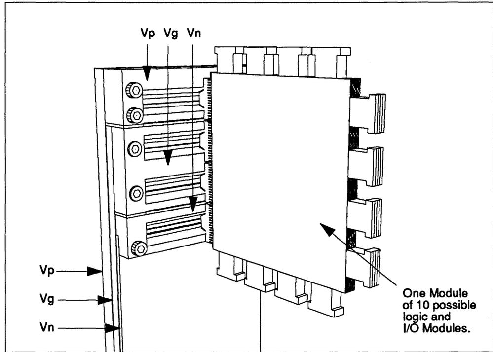
**FIGURE 144. Horizontal Power Buses for Logic Modules.**
