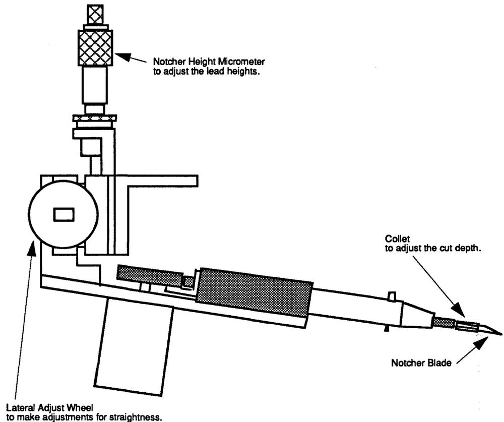
The capillary is then withdrawn from the die surface exposing the gold wire as the head is raised. At this point an automatic notching mechanism moves into the area of the exposed gold wire and strikes both sides of the wire with a steel blade. This is essentially a scissors action which cuts most of the way through the gold wire. The notch is made 0.432 mm above the surface of the die. This step in the process is illustrated in Figure 90.
