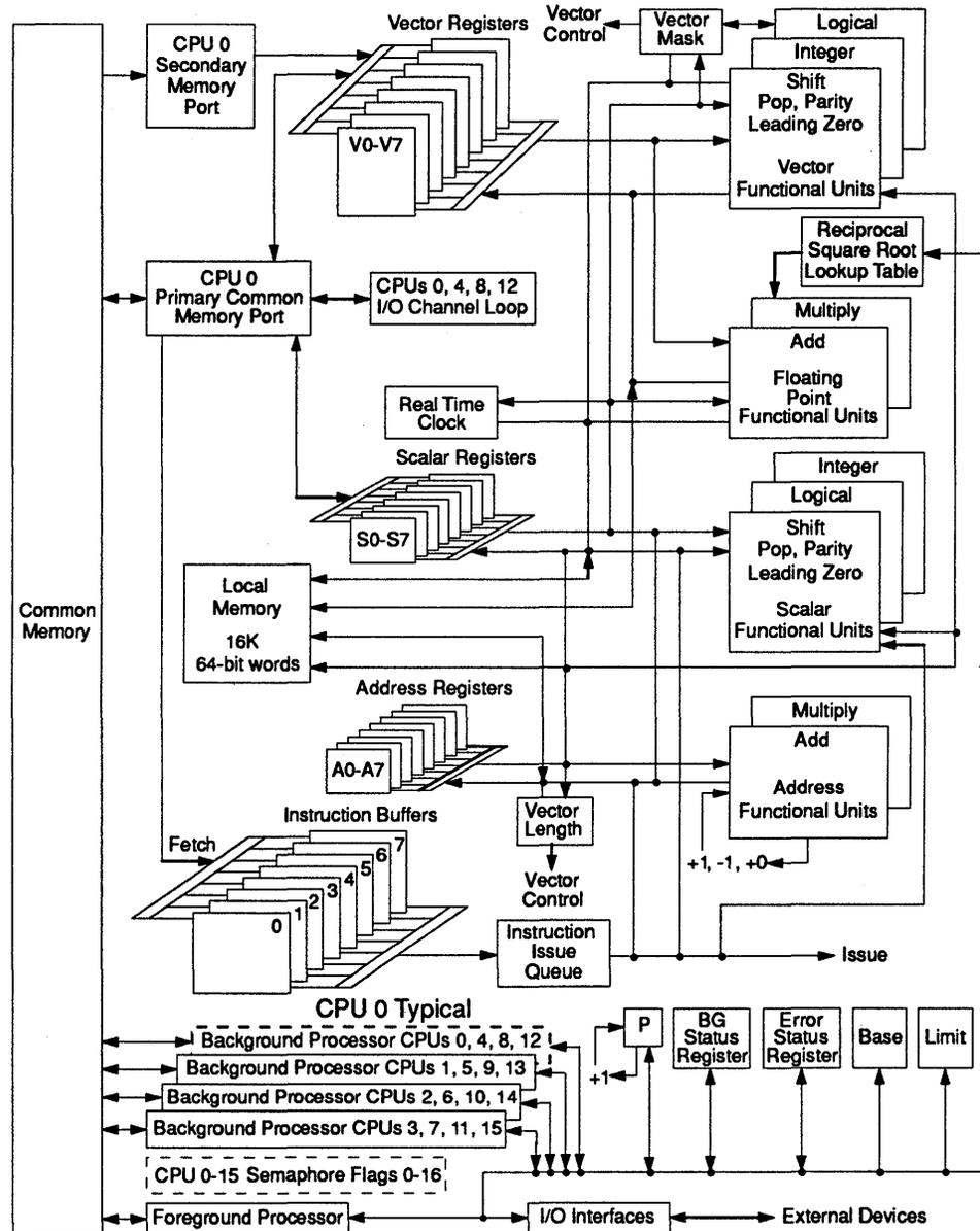
Each background processor has a small high speed local memory to hold scalar or vector operands during a computation (16,384 words are available for each Background Processor). Data is moved from the Common Memory to the local memory and returned at the end of each computation. Arrays of data are addressed by the Background Processors directly in the Common Memory. The access to data common to multiple Background Processors is interlocked by the Background Processor semaphore flags.
