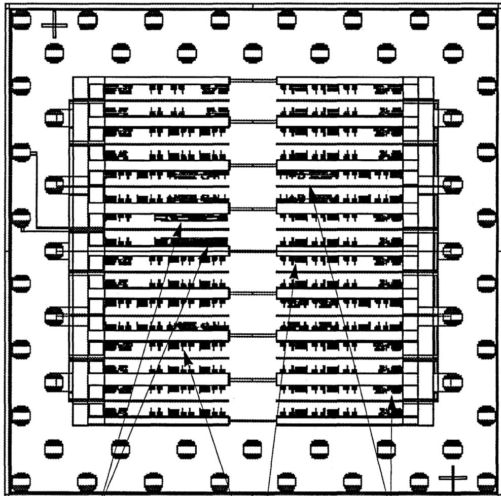
The clock amplifiers (the CC cells) have been placed in their proper location on the north and south side of west D street.
