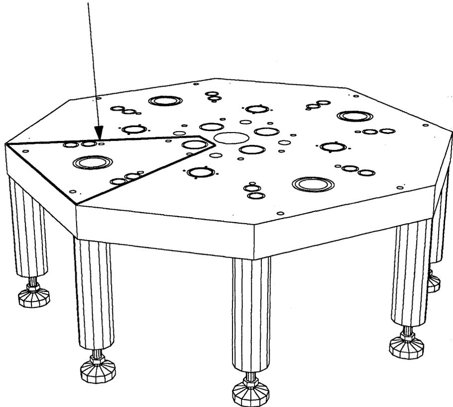
**FIGURE 135. Top Plate for a Four-Processor CRAY-3.**
