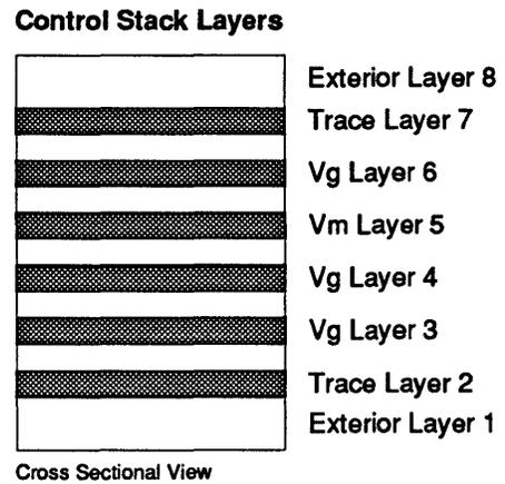
Note: On memory modules all the board stacks use memory boards except for D, H, L, and P. These are the control stacks.
