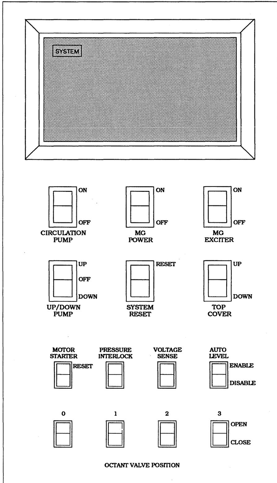
There are six switches on the front panel for primary operation of the CRAY-3. The switches are mounted to the user switches board which is located behind the front panel. These six user switches include 1) the on/off switch for the circulation pump, 2) the on/off switch for the motor generator power, 3) the on/off switch for the motor generator exciter, 4) the direction of the up/down pump, 4) the system reset switch, and 6) the lift switch for the top cover.
