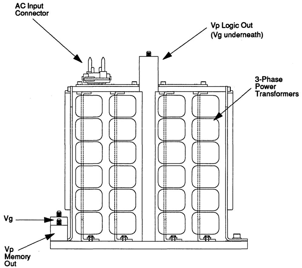
**FIGURE 147. Simplified Top View of a Vp Memory Power Supply.**
