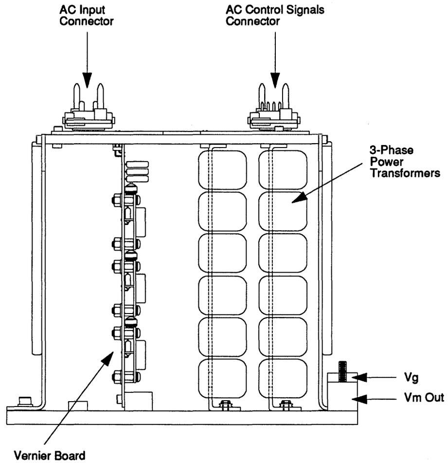
**FIGURE 149. Simplified Top View of a Vn Power Supply.**
