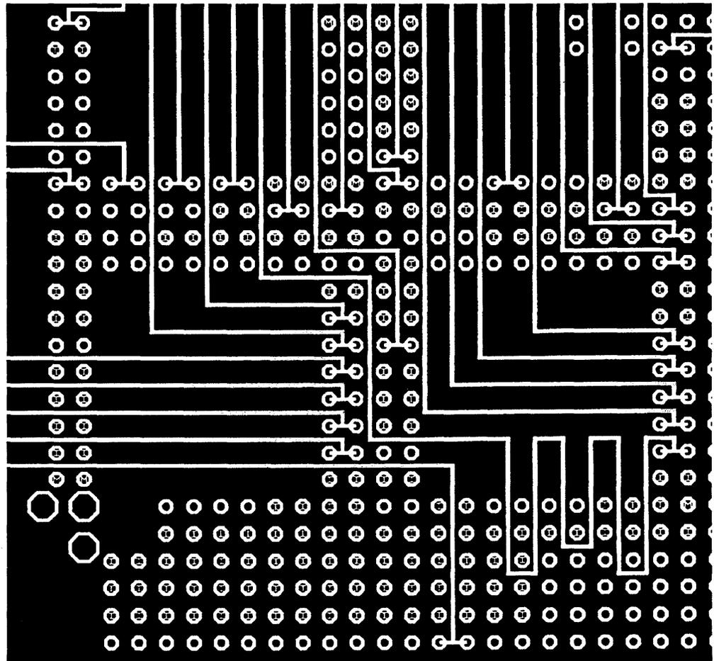
Note: Because the resolution is not high enough the trace lines shown above appear to be only one solid line. However, in reality they are paired lines which only separate near the destination jumpers. Only one of each trace line contacts each of the paired jumpers.
