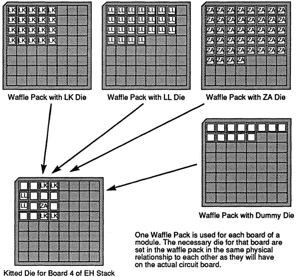
After all the die have been kitted for a module, the kitted waffle packs are delivered to Die Attach where the correct bonded die are attached to the printed circuit boards which have come from Board Solder.
