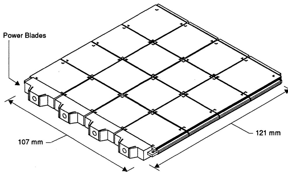
The modules are three dimensional structures measuring 121 mm by 107 mm by 7.14 mm thick. The circuit packages within the modules are unpackaged gallium arsenide or silicon die mounted directly on multi-layer circuit boards.
