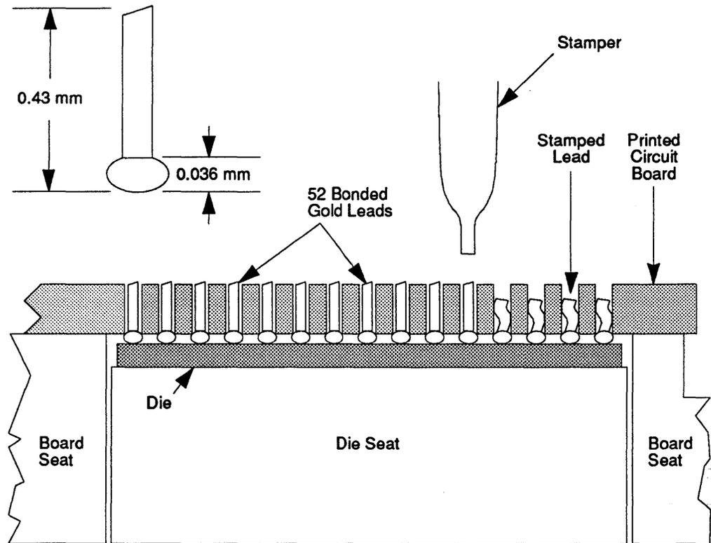
The complete fixture holding the board and the die is now placed in a stamper. The stamper is a modified Hughes bonding machine which forces a shaped hardened tool to compress the gold lead into the barrel of the printed circuit board. The compression is controlled by using a pre-determined force. The lead is compressed to a depth of about 0.178 mm into the barrel forming a plug. Notice the illustration of a stamped lead in Figure 119.
