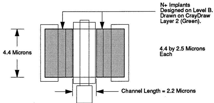
Figure 18 shades the areas of the transistor design which have ohmic metal. The ohmic metal breaks down the substrate surface barrier which would otherwise result in a Schottky diode. These two areas of ohmic metal are essentially the metal terminals of the transistor for the source and the drain elements.
