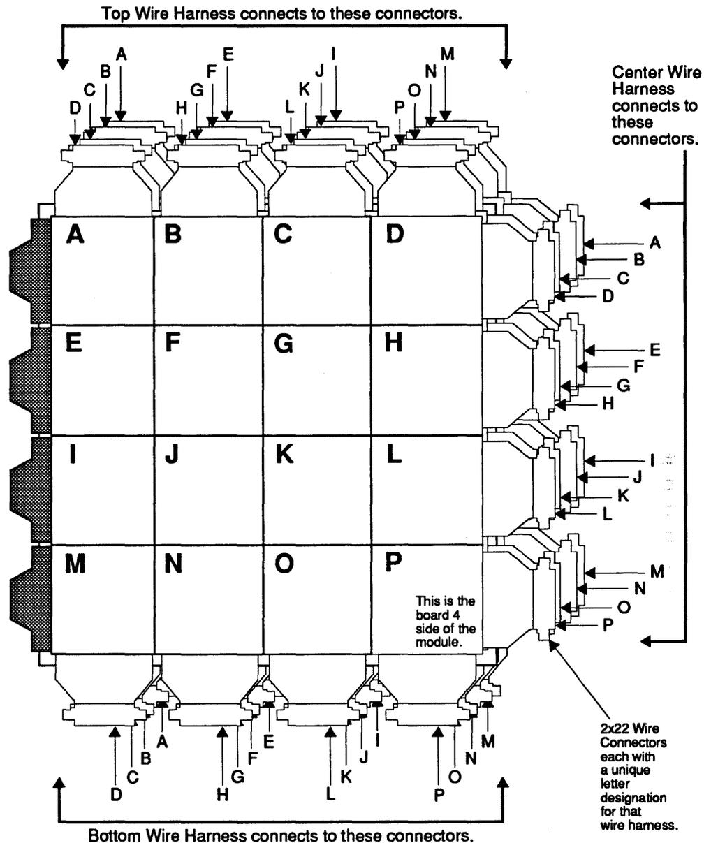
The connectors used are a molded plastic part with two rows of 22 pins. One row of pins connects to the true (logical zero in the CRAY-3) wires of a twisted pair of 34 AWG wire. The other row connects to the false (logical one in a CRAY-3) wires of the twisted pair. There are 22 twisted pairs of 34 AWG wire on each connector.
