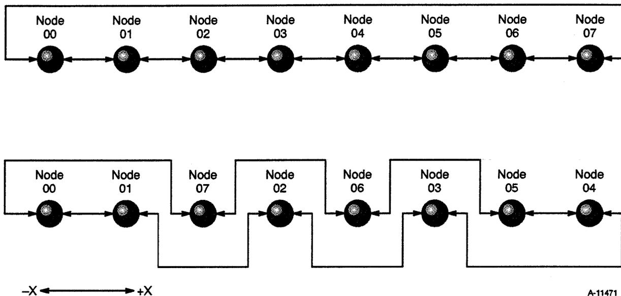
Figure 2-7. Interleaving
