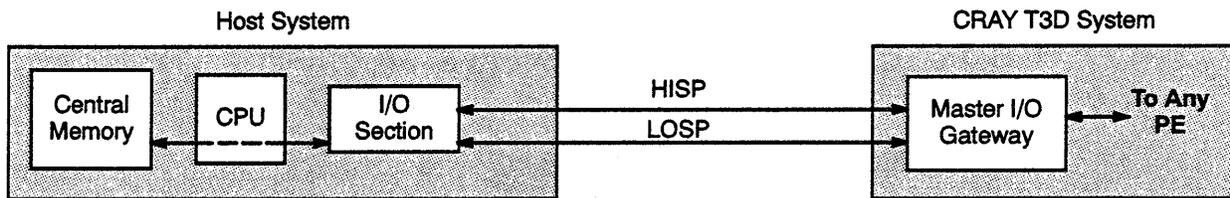
Figure 4-5. Phase 1 I/O Gateway Channel Configuration
