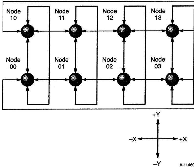
Figure 2-5. Two-dimensional Torus Network
