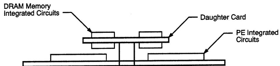
Figure 3-12. Side View of PE Circuit Board
