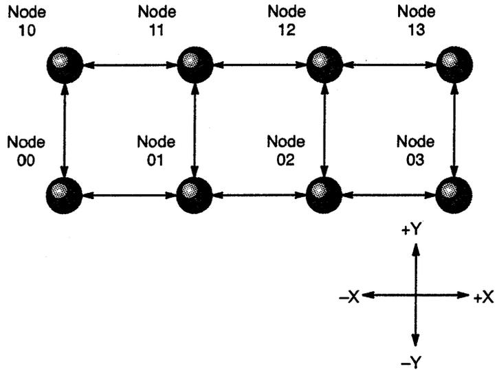
Figure 3-4. Virtual Node Numbers of a Two-dimensional Array
