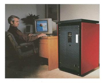
The CRAY EL92 deskside computer system delivers CRAY Y-MP and CRAY C90 compatibility to an office environment at a low price point. With up to two processors and 512 Mbytes (64 Mwords) of central memory, the CRAY EL92 system offers a clear upgrade path to large-scale parallel Cray Research supercomputing.
