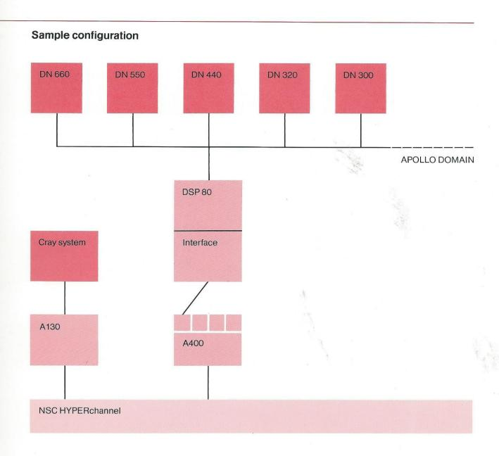
The Station Concentrator is a server process that resides on the node connected to the HYPER-channel. Users communicate with this module through the APOLLO mailbox utility. The Station Concentrator generates the appropriate Device Driver calls to send or receive messages and data from the CRAY. It also directs messages and data from the CRAY to the intended recipient.
