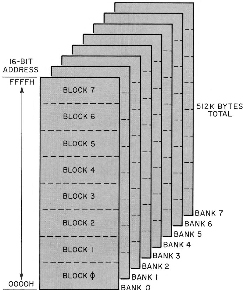
memory bank, and each reset bit (logic 0) disables its bank. Control byte bit 7 (MSB) controls memory bank 7, bit 6 controls memory bank 6, etc.
