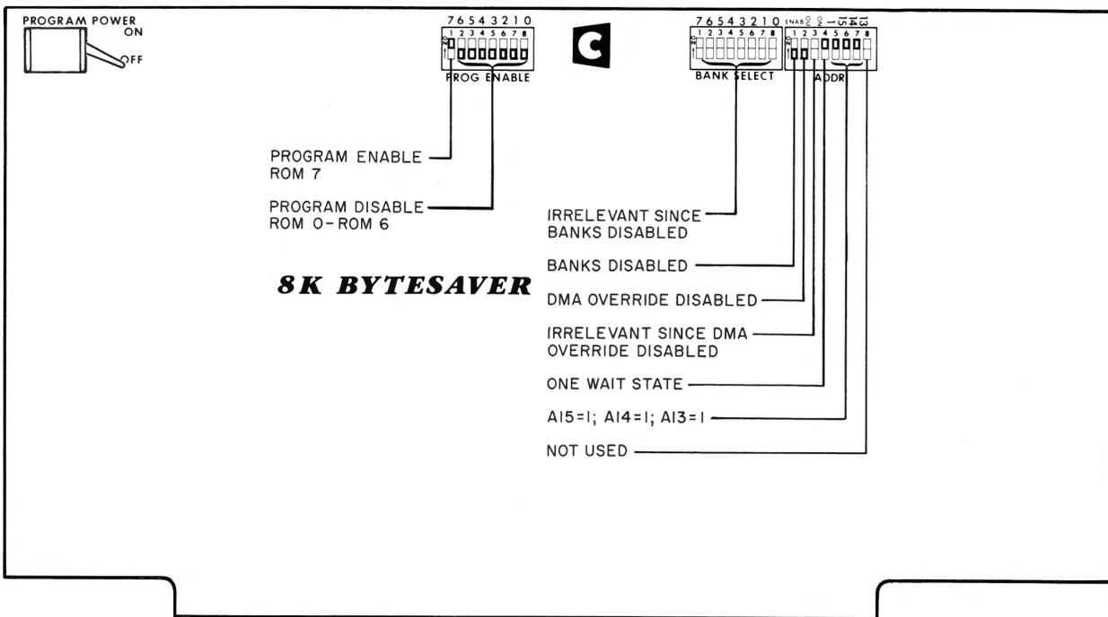
The correct BYTESAVER II switch settings for this configuration are then shown in Figure 4. ■
