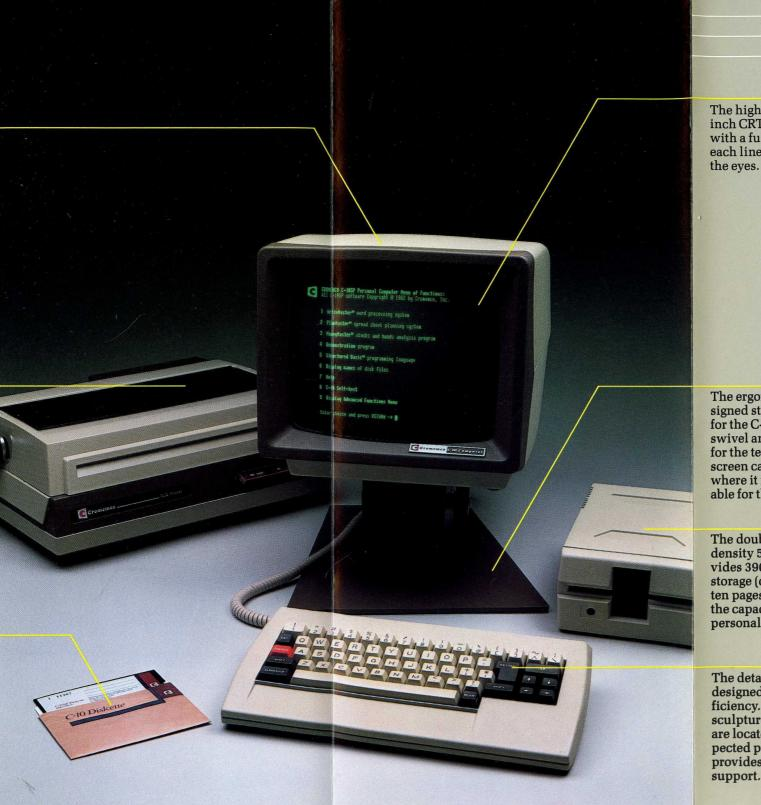
The high-resolution 12inch CRT displays 25 lines with a full 80 characters on each line. And, it's easy on the eyes.
