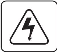
**DANGEROUS VOLTAGE:** The lightning flash with arrowhead symbol, within an equilateral triangle, is intended to alert the user to the presence of uninsulated “dangerous voltage” within the product's enclosure that may be of sufficient magnitude to constitute a risk of electric shock to persons.
