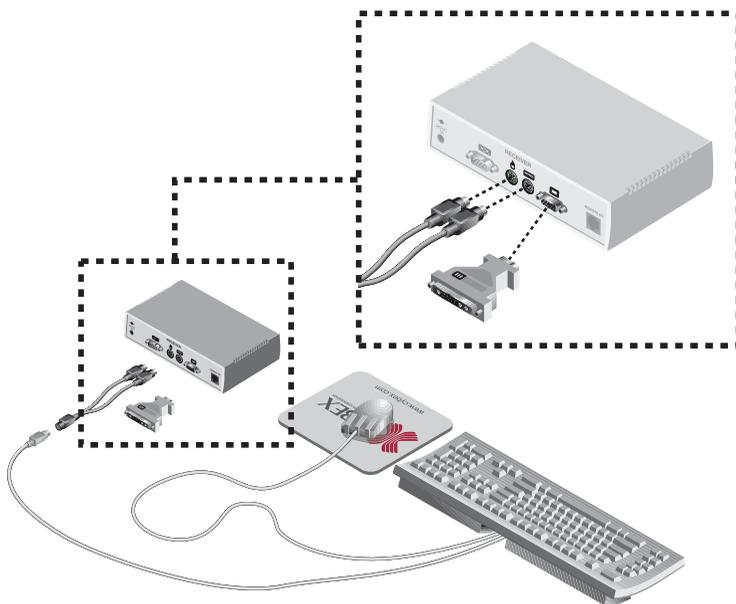
6. Connect the Category 5 cable to the modular jack on the rear of the Receiver.
