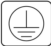
**PROTECTIVE EARTHING TERMINAL:** A terminal which must be connected to the earth prior to making any other connections to the equipment.
