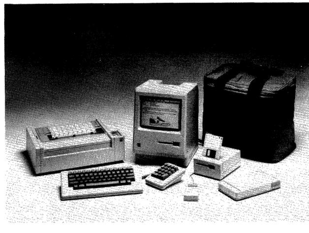
**Mass Storage** • two 3.5-inch, 400K-byte hard cover diskettes, 1 internal drive standard, 1 external drive available; available from third-party vendors include: Winchester hard disks, cartridge hard disks, and tape backup in first, second, and third quarters of 1984.
