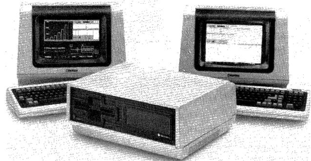
TS 804 comes with 320K bytes of RAM and 64K bytes of cache; TS 816/40 comes with 128K bytes of RAM.
