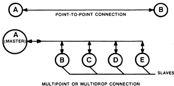
Figure 1 • direct connection arrangements.
