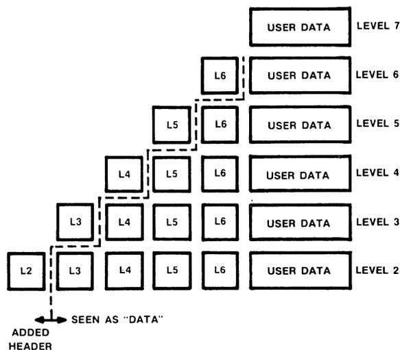
Figure 7 • header usage in an OSI-model protocol.
