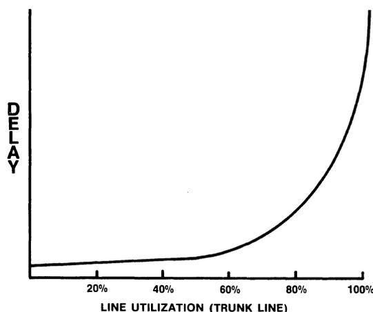
Figure 7 • statistical multiplexer delay.
