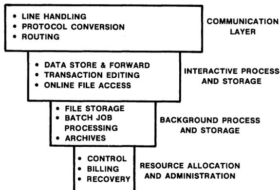
Figure 6 • logical layers of a processing services network.
