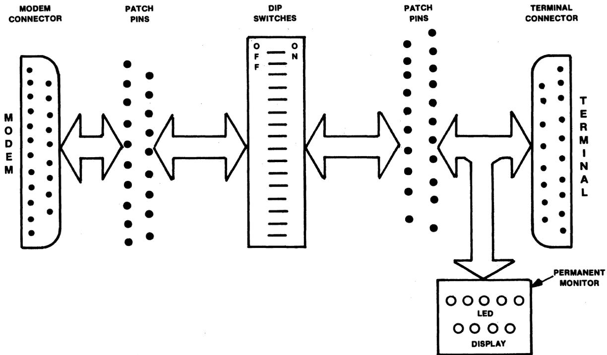
Figure 9 • inside a typical breakout box.
