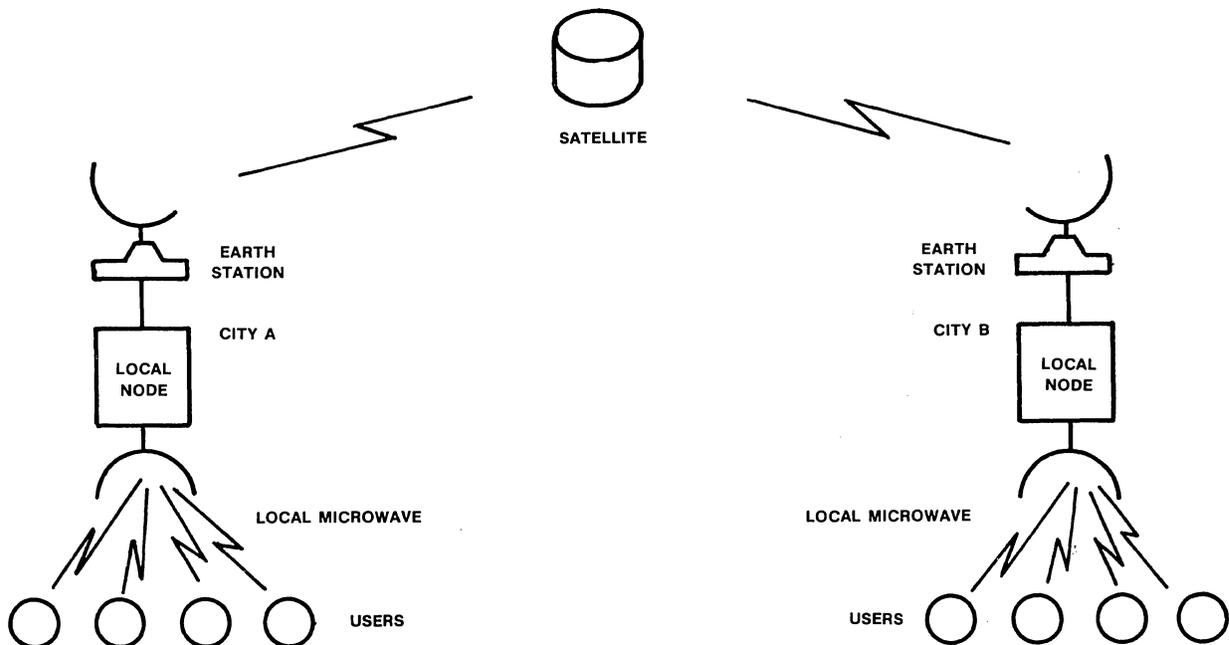
Figure 10 • a typical digital termination system.
