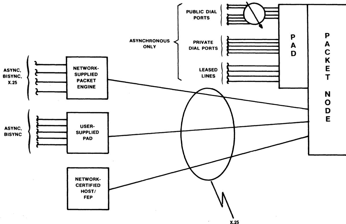
Figure 9 • connecting to a packet network.
