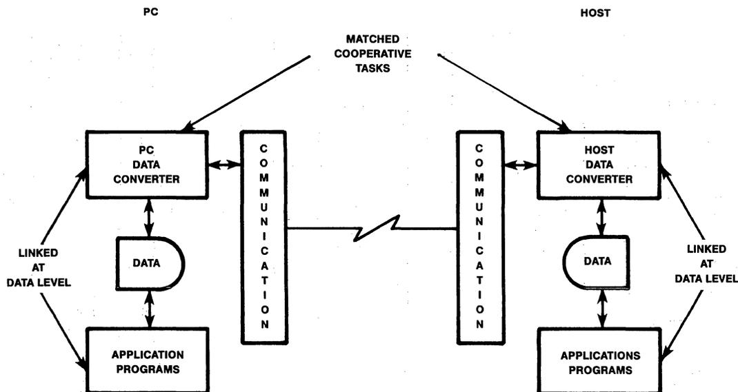
Figure 7 • a loosely coupled integrated application.
