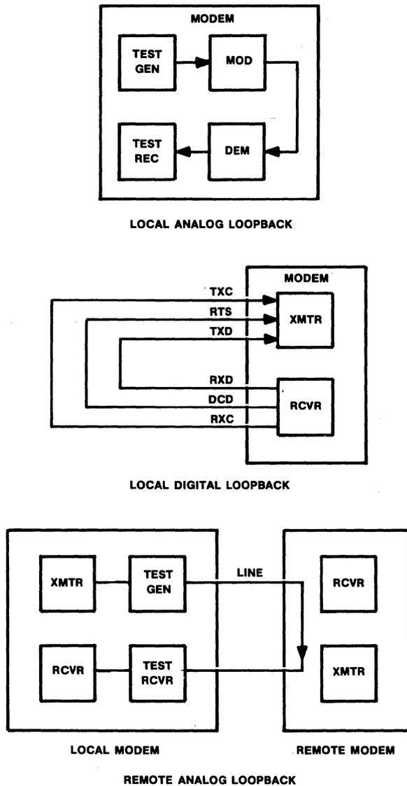
Figure 7 • modem loopback configurations.
