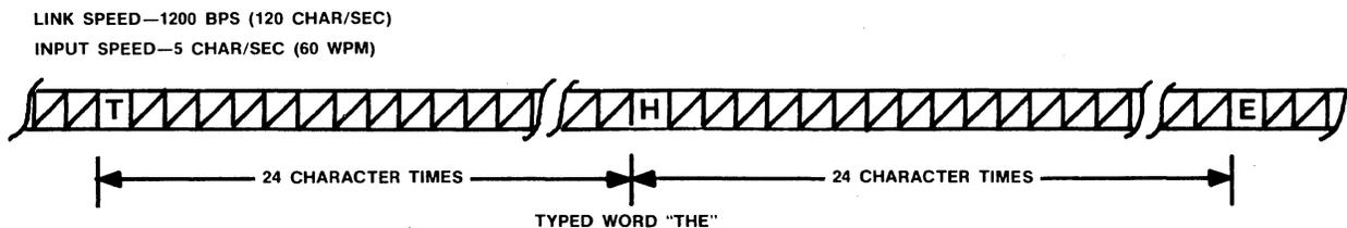
Figure 8 • example of relative line utilization of unbuffered terminal.
