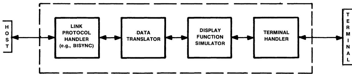
Figure 2 • protocol converter structure.
