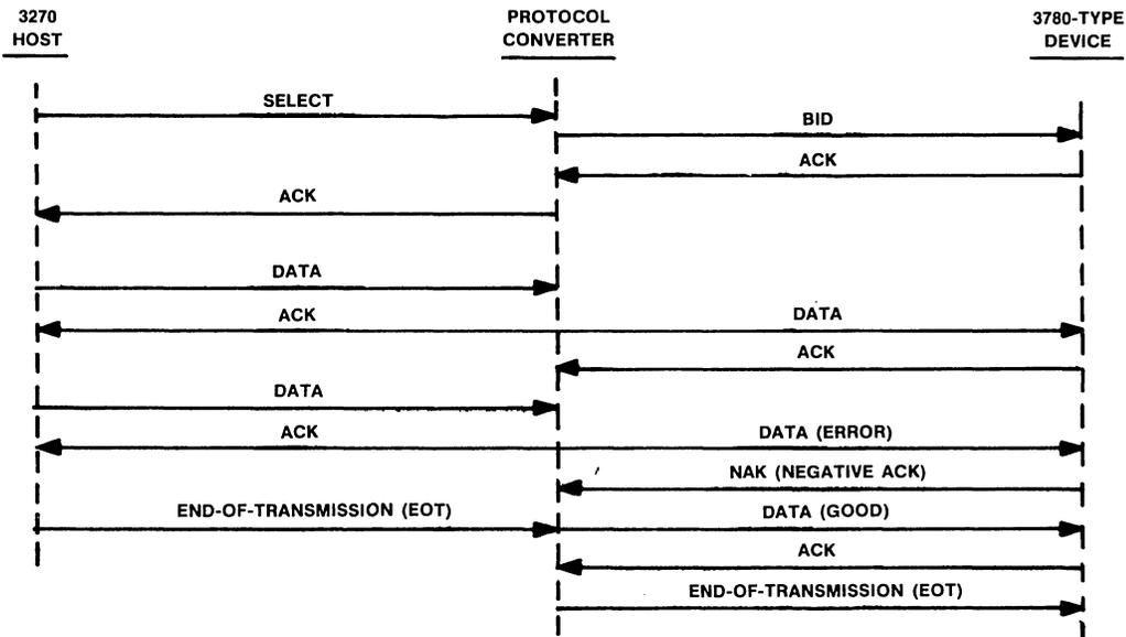
Figure 6 • a complete sequence in protocol conversion.
