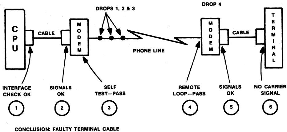
Figure 2 • example of sequential testing.
