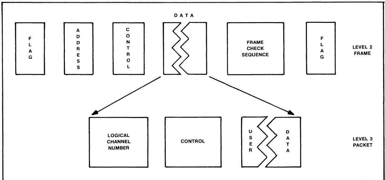
Figure 2 • X.25 frame and packet structure.
