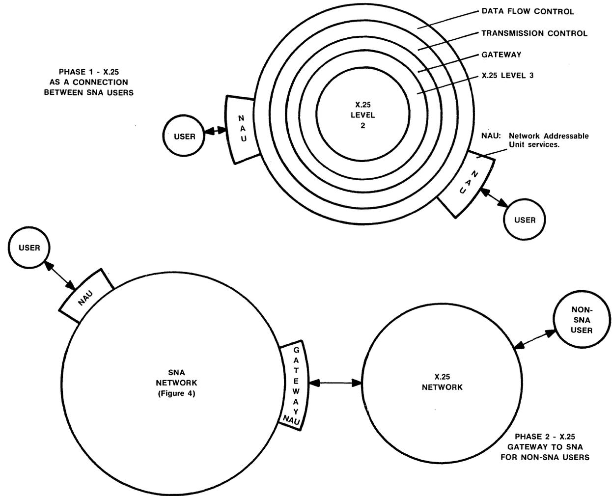
Figure 10 • IBM X.25 support models.
