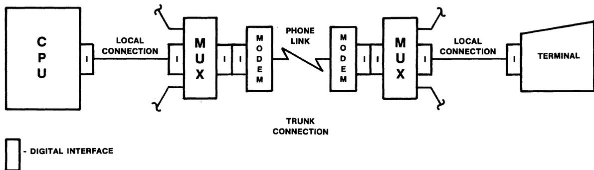
Figure 4 • the digital path as a system.
