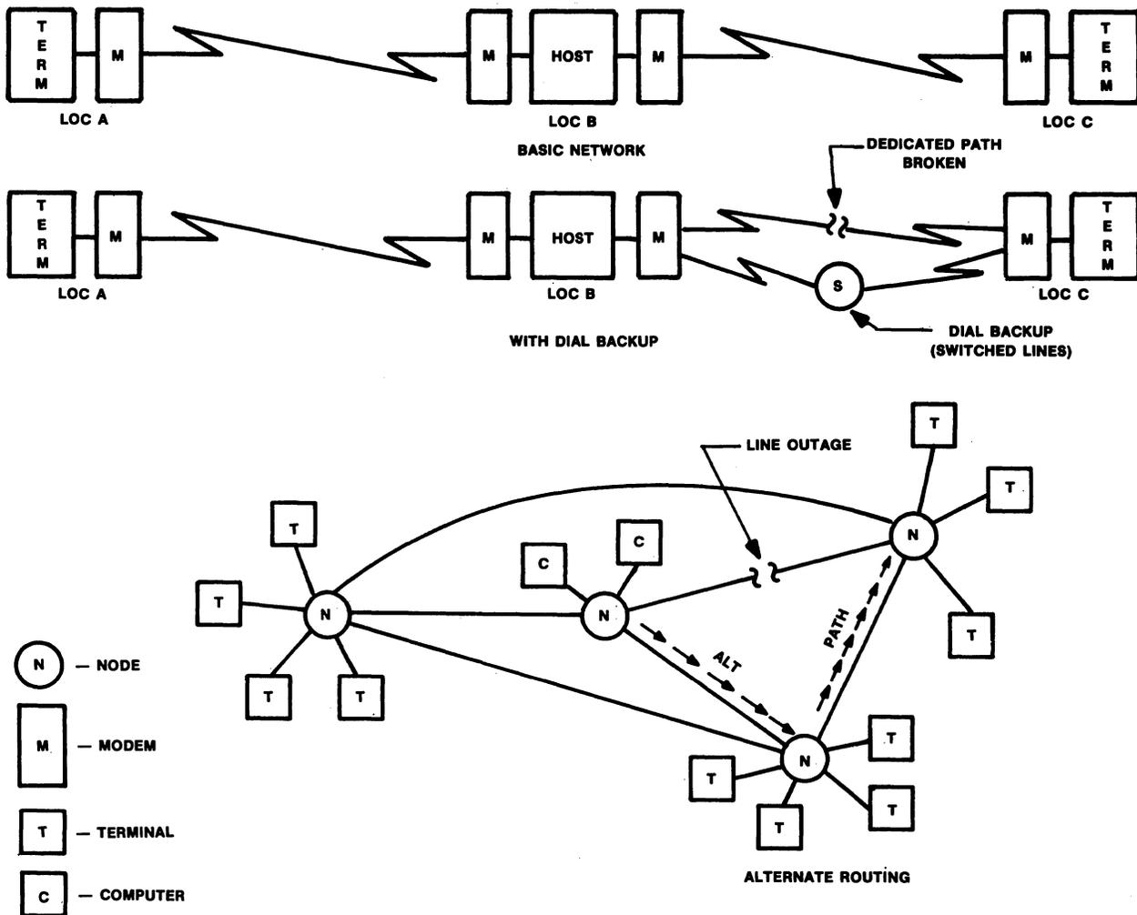
Figure 1 • networks and fault tolerance.
