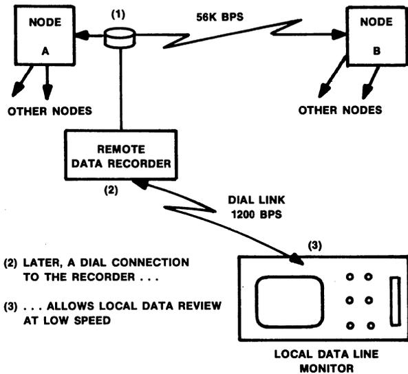
**Figure 14** • example of remote data recorder application.
