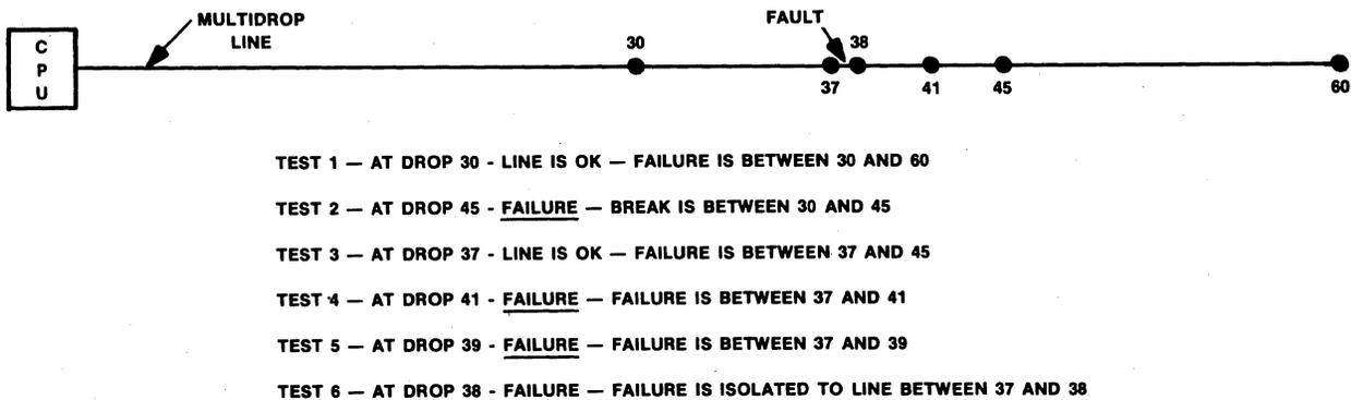
Figure 3 • failure isolation using halving & bracketing.
