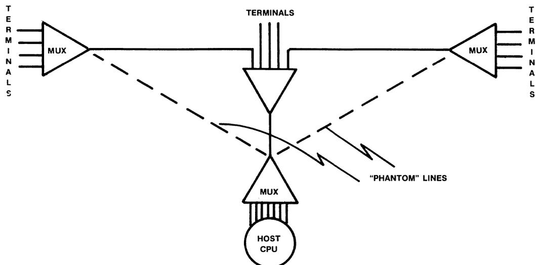
Figure 1 • "phantom lines" hidden from host control.
