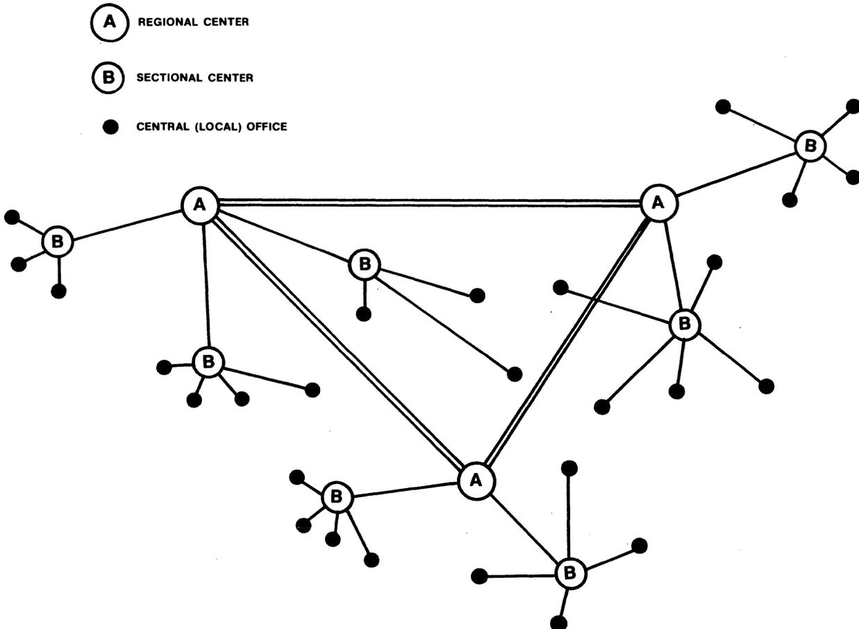
Figure 7 • telephone switching structure.
