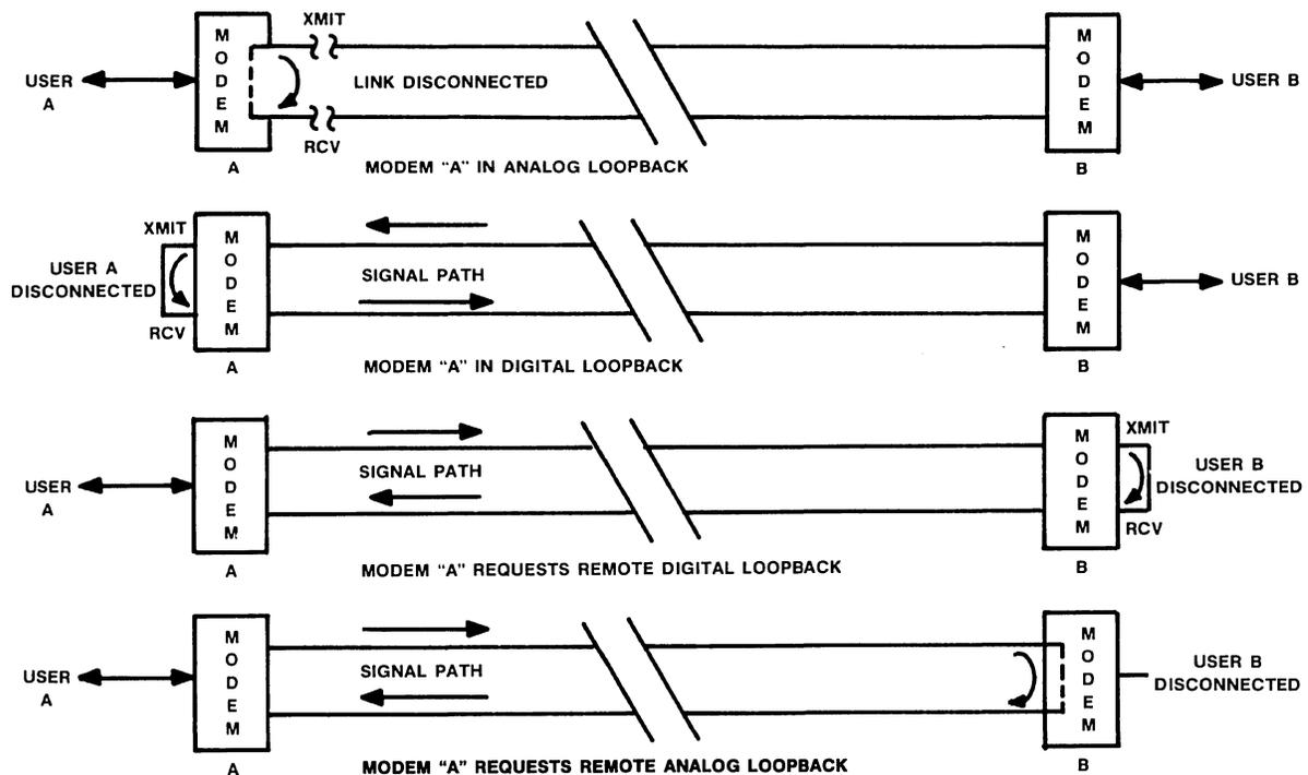
Figure 6 • analog and digital loopback.
