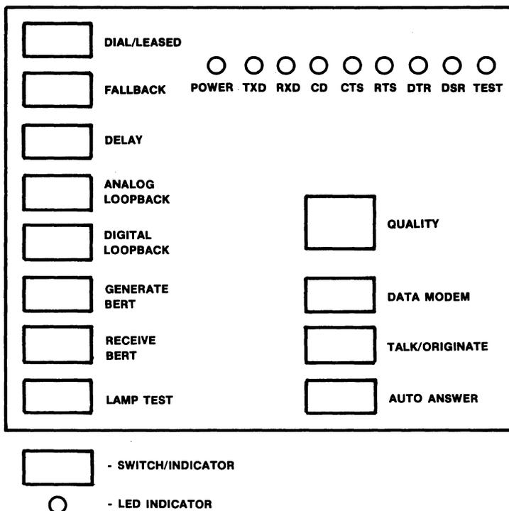
Figure 5 • typical modem front panel.
