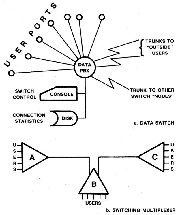
Figure 2 • data switches and multiplexers.
