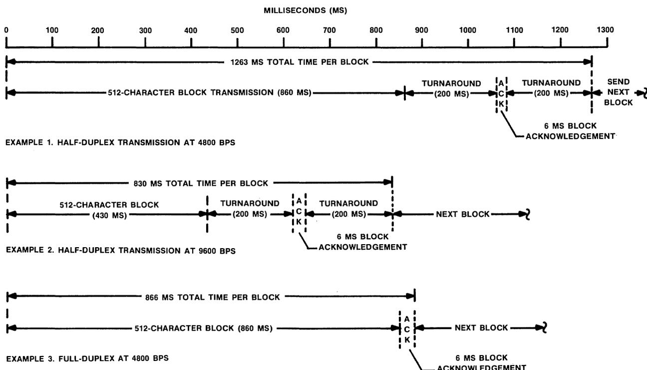
Figure 5 • effects of half-/full-duplex vs speed on transmission time.
