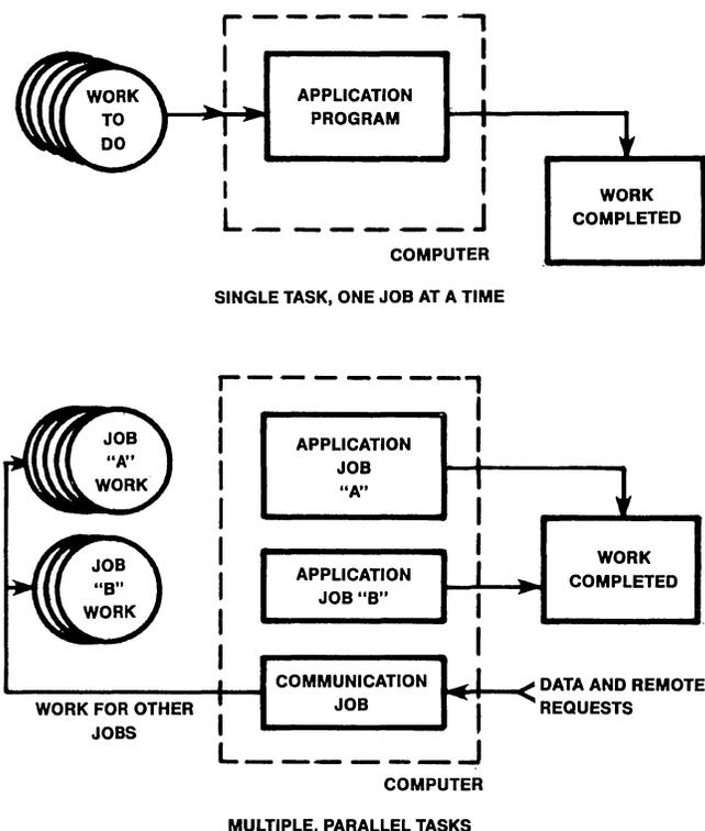
Figure 2 • work flow in single and multitask systems.
