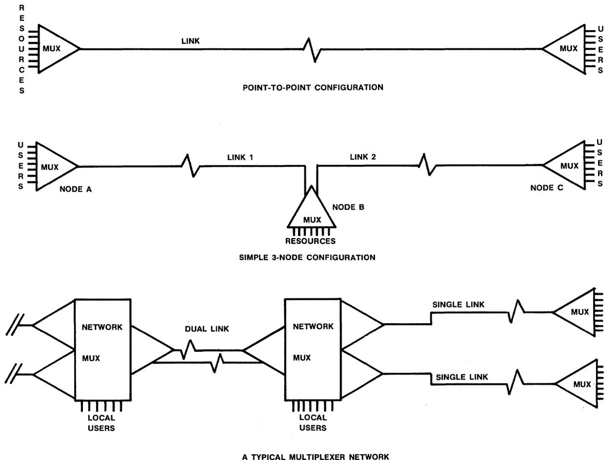
**Figure 12** • typical multiplexer configurations.
