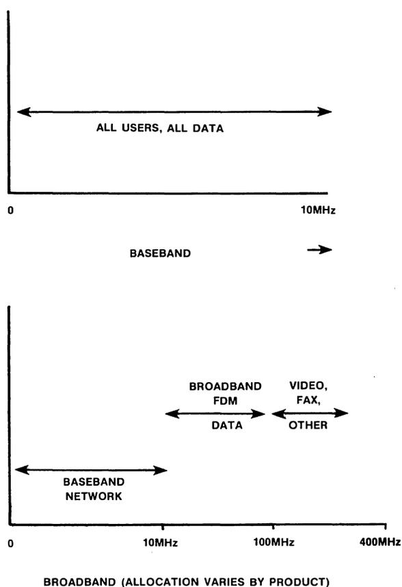
Figure 4 • broadband/baseband frequency uses.
