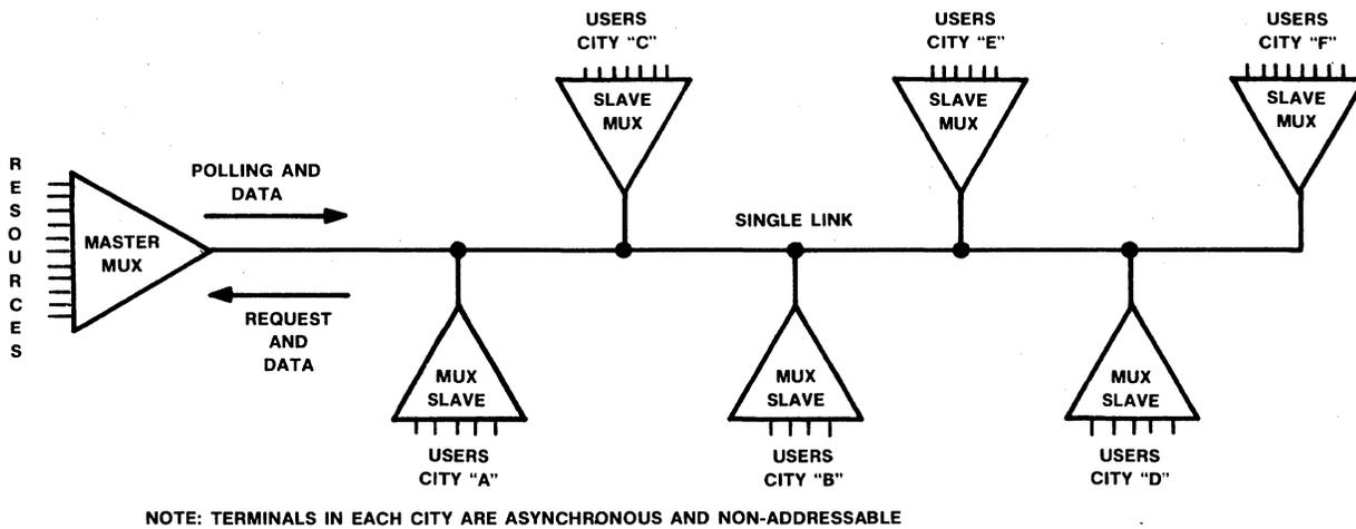
Figure 13 • typical multipoint multiplexer configuration.
