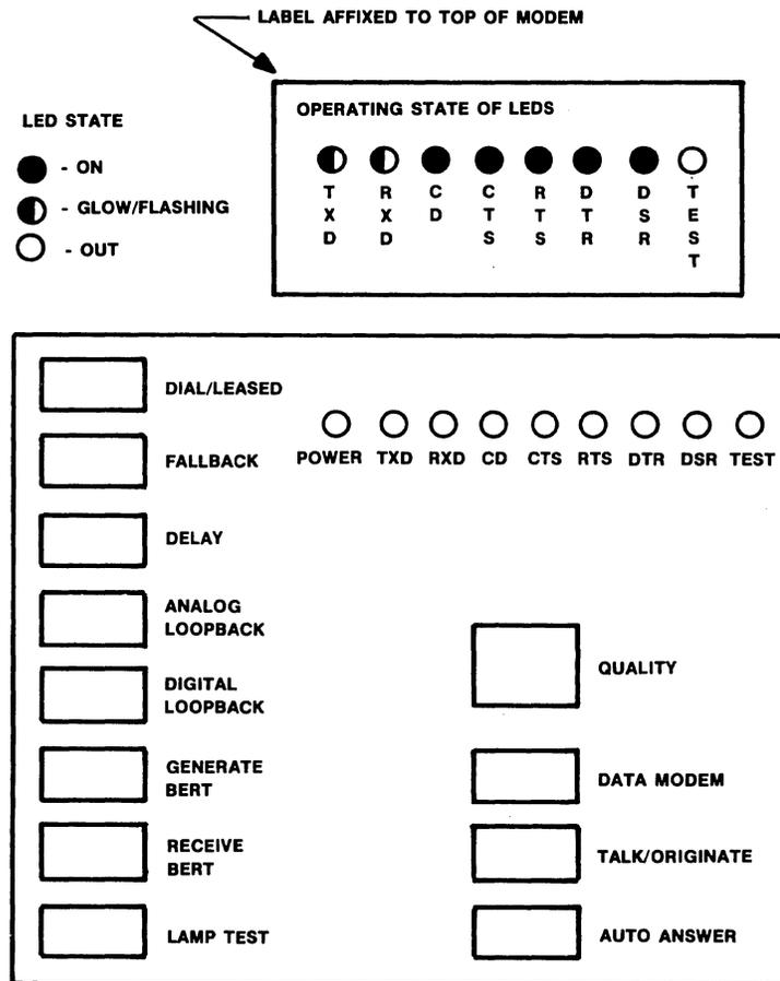
Figure 6 • labeling a modem for indicator states.
