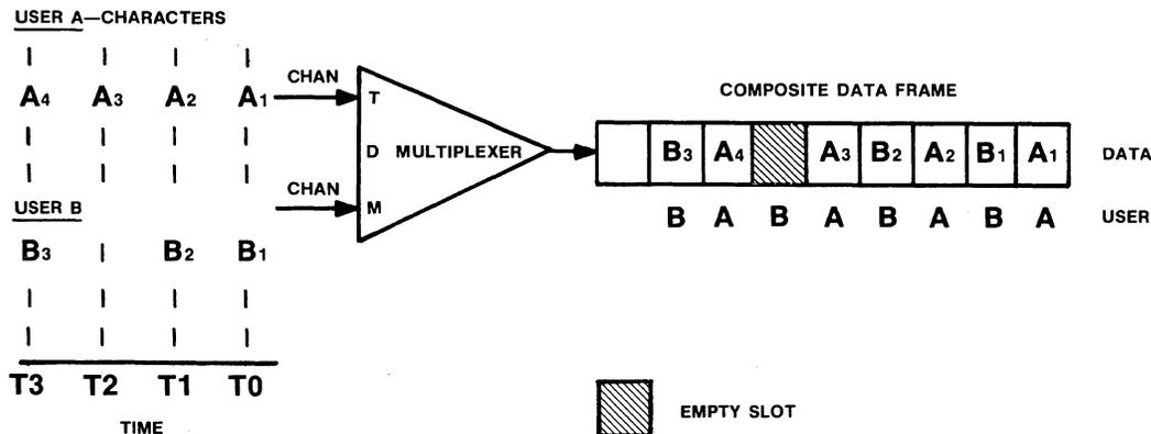
**Figure 10** • character interleaved TDM operation.
