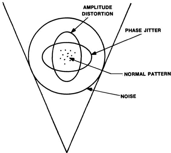
Figure 20 • effects of line problems on the eye pattern.
