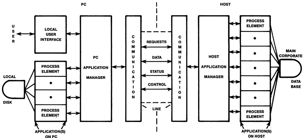
Figure 6 • a tightly-coupled integrated application.
