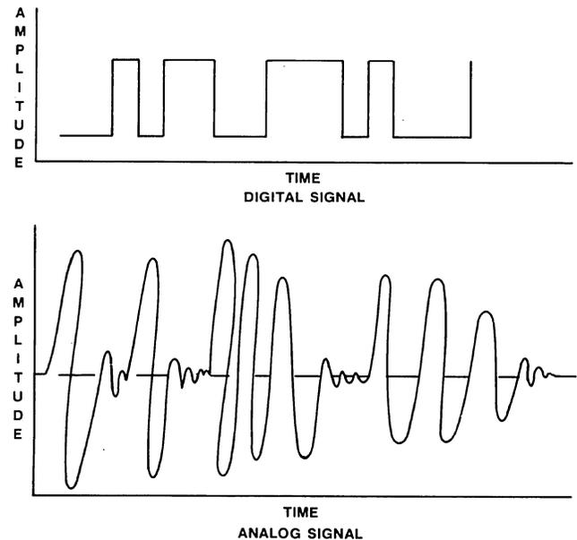
Figure 1 • digital vs analog signals.
