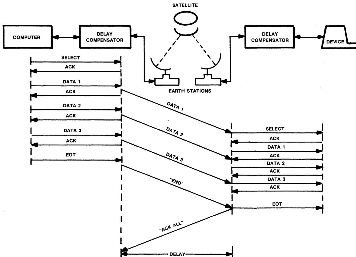
Figure 8 • delay compensation.
