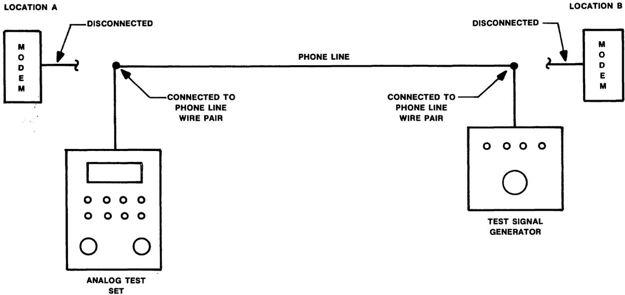
Figure 17 • using analog test equipment to determine phone line parameters.
