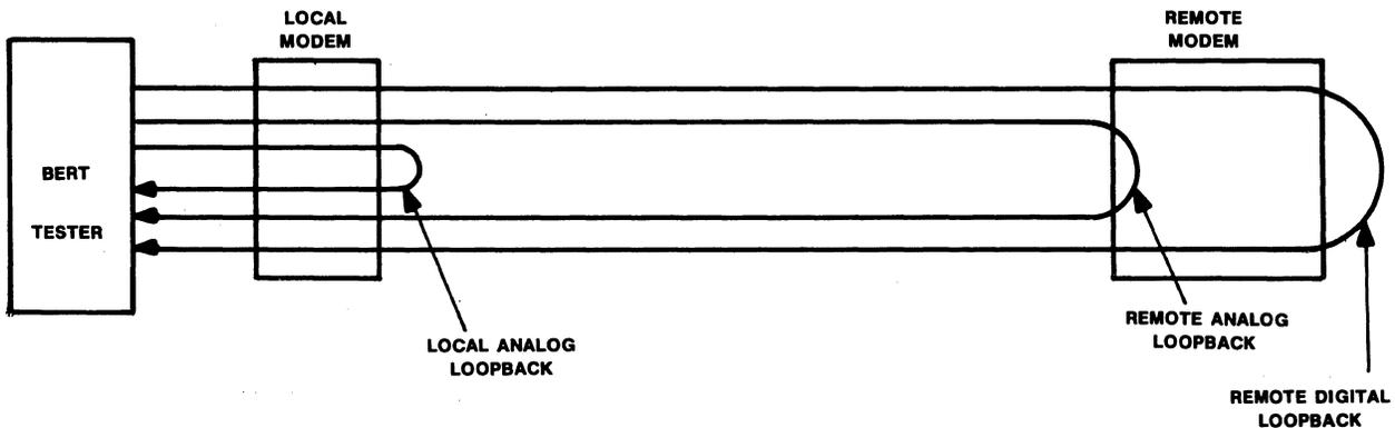
Figure 10 • bit error rate testing.
