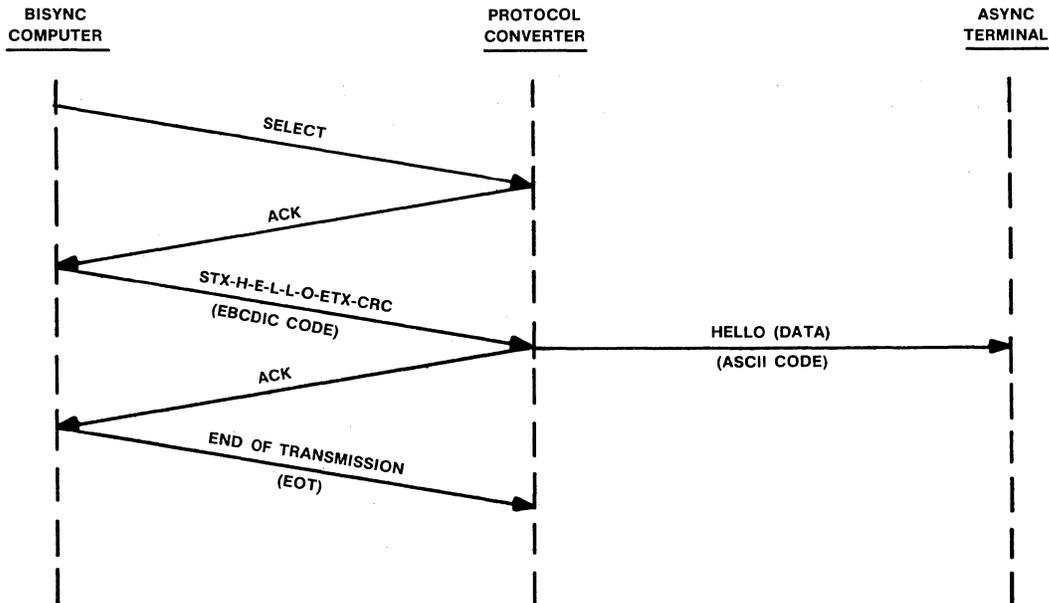
Figure 4 • data isolation in protocol conversion.
