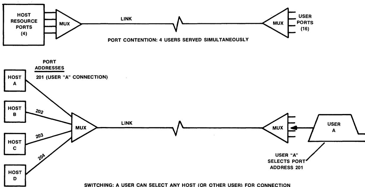
Figure 14 • examples of port contention and port switching.
