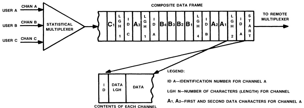
Figure 11 • statistical multiplexer operation.
