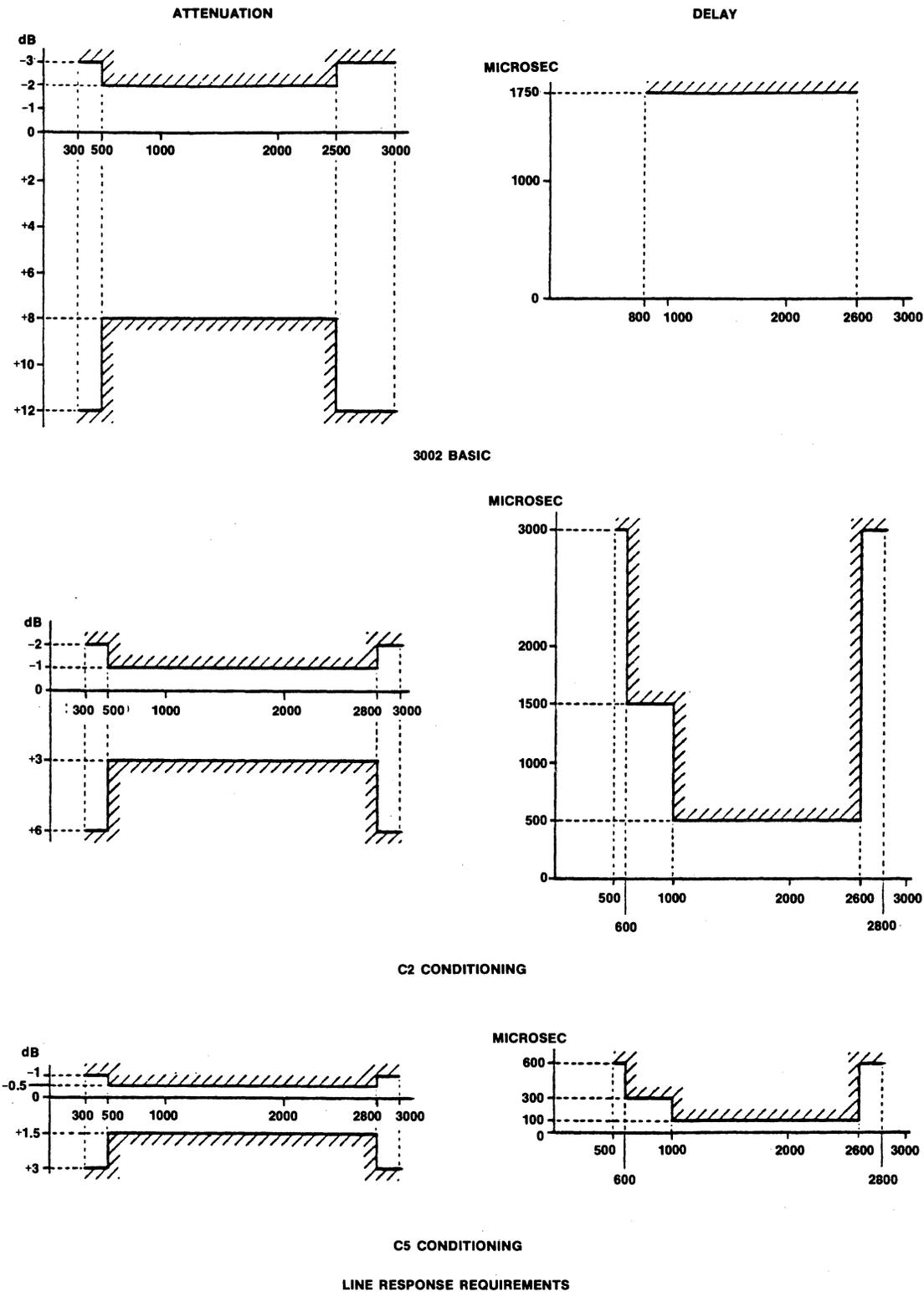
Figure 16 • effects of line conditioning.
