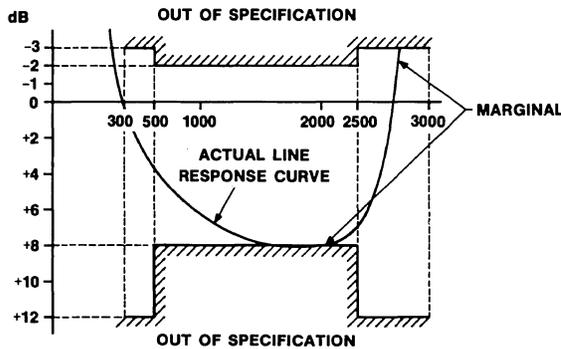
Figure 18 • line parameter display—3002 attenuation vs specification.
