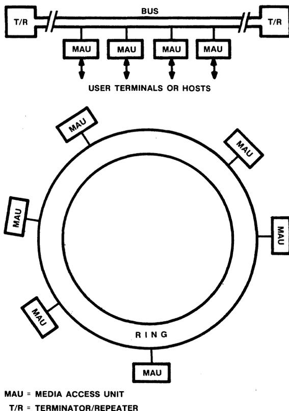
**Figure 3** • ring and bus cable networks.
