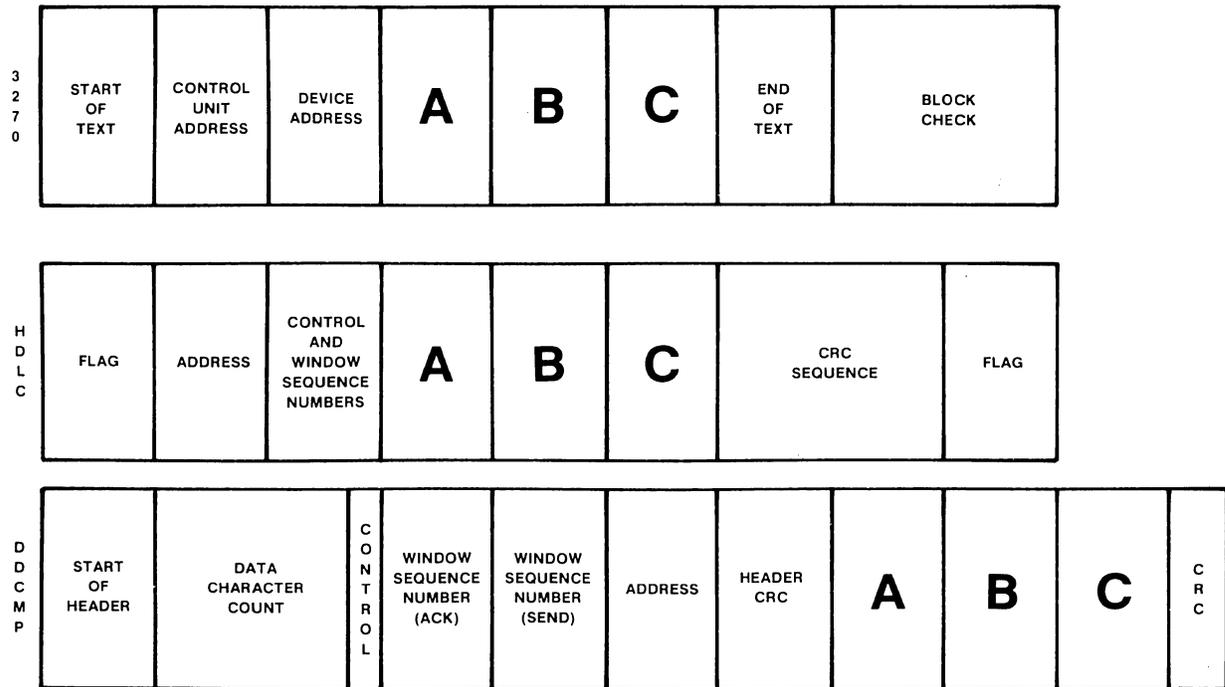
SDLC/HDLC FIGURE SHOWS AN I-FRAME, NOT AN SNA OR X.25 "PACKET"
