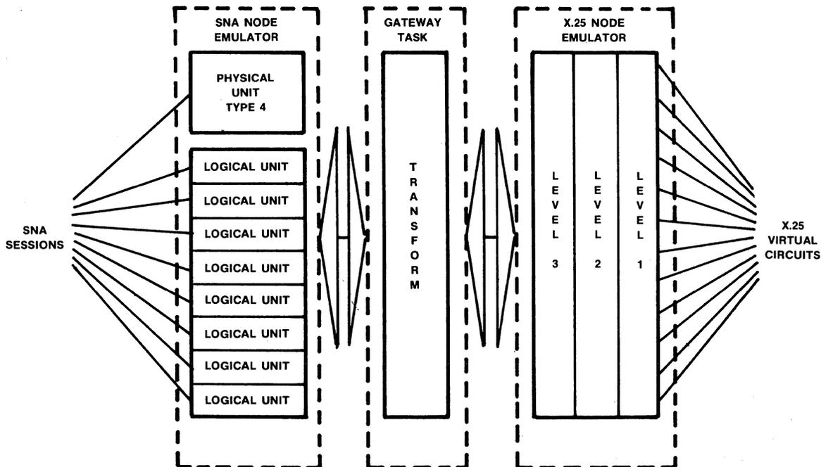
**Figure 11** • IBM SNA to CCITT X.25 gateway.
