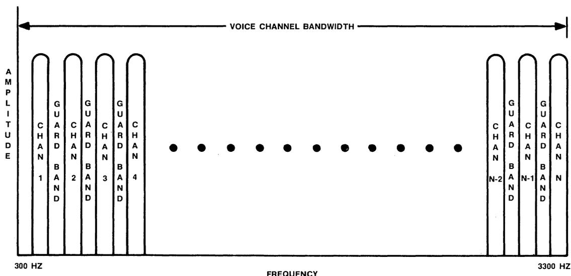
Figure 9 • FDM multiplexing technique.
