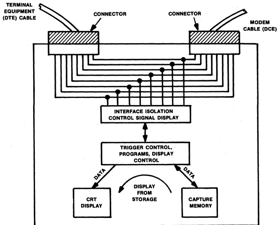
Figure 12 • internal configuration of a data line monitor.
