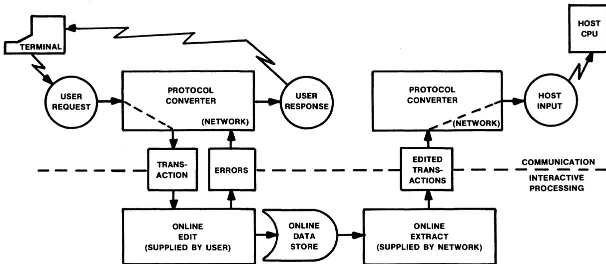
Figure 13 • an example of using network processing services.
