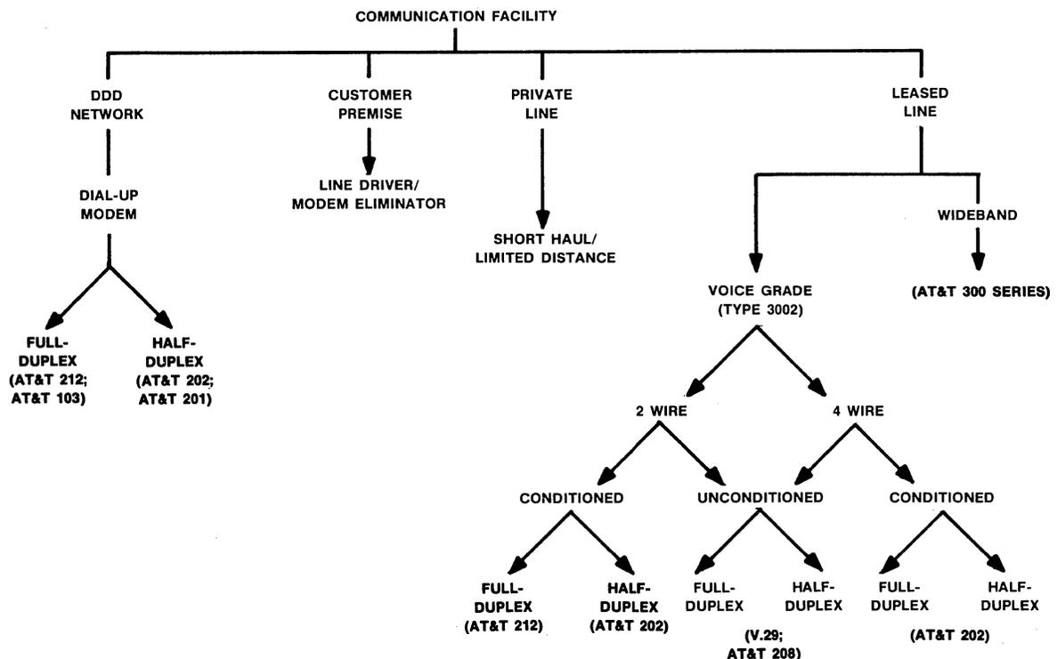
**Figure 3** • communication facility vs modem type.
