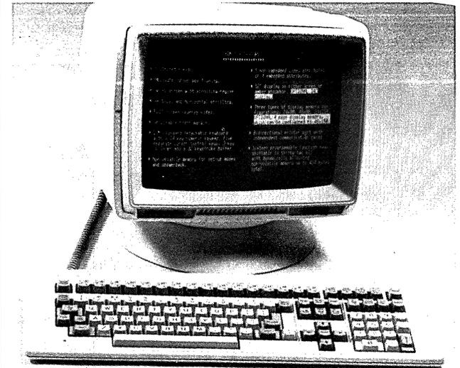
The new ADM 12plus terminal features a 24-line x 80-/132-column display format, up to 4 pages of display memory, and 16 programmable function keys (shiftable to 32 functions).
