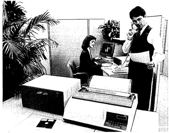
The NCR 7950 competes against the IBM 3274 C models and supports up to 32 terminals/printers. No color display or personal computer support is offered, however.
