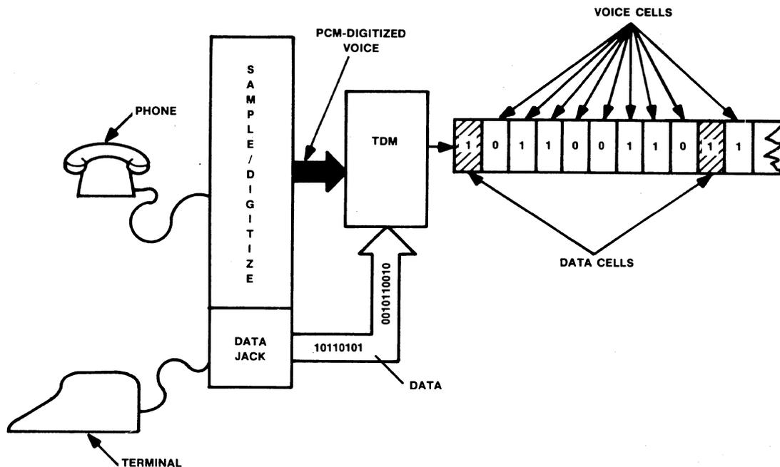
Figure 8 • digital data in a PCM-based digital PBX.
