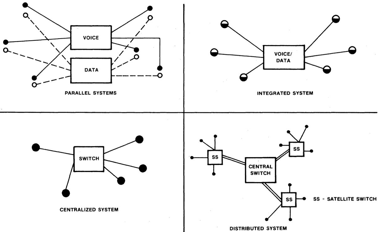
Figure 1 • PBX architecture alternatives.
