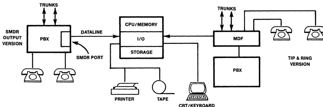
Figure 1 • Call Accounting System Configuration
