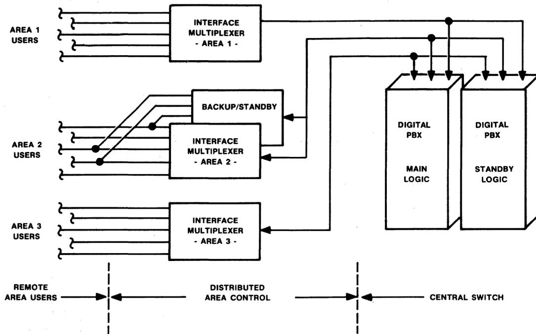
Figure 11 • parallel and distributed elements in a high-reliability switch.
