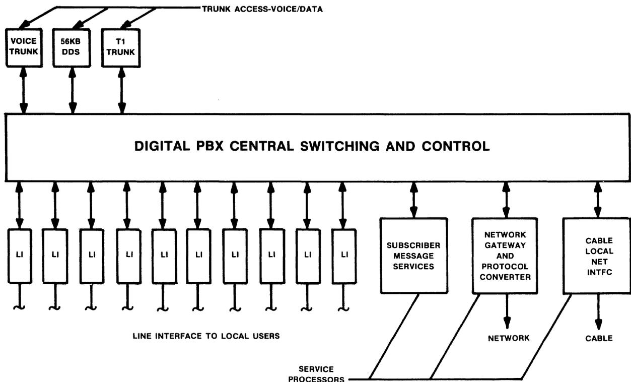
Figure 12 • service processors/gateways in a digital PBX.
