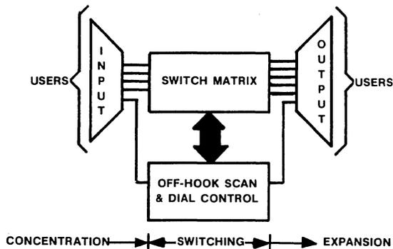
Figure 2 • basic electromechanical switch.
