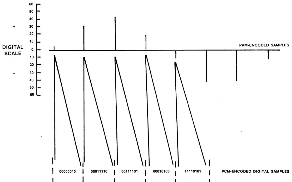
Figure 7 • digital pulse code modulation (PCM).
