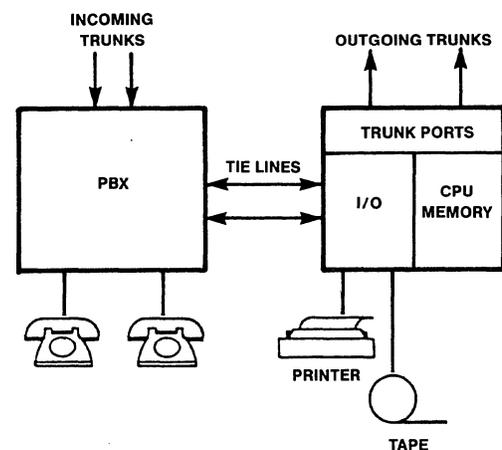
Figure 2 • Least Cost Routing System Configuration
