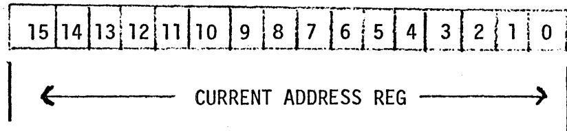
The current address register is used to supply the actual memory location where data is transferred. This register is incremented after each transfer.
