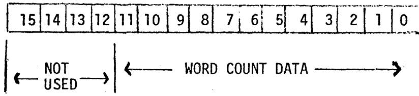
The word count register is a 12 bit counter/register which determines the number of transfers that will occur. The register is loaded with the two's compliment of the desired word count. An interrupt is generated on overflow signifying the end of range in data transfers.
