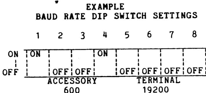
When you have completed setting the baud rate switches to the baud rate specifications required by your equipment, reconnect the leftmost ribbon cable and carefully slide the I/O Logic Board into its slot in the card rack. If you meet resistance, gently rock the board from side to side until it slips in--DO NOT FORCE IT! Close up the back of the unit (per Section 3.5) and re-plug the AC IN to a power source.
