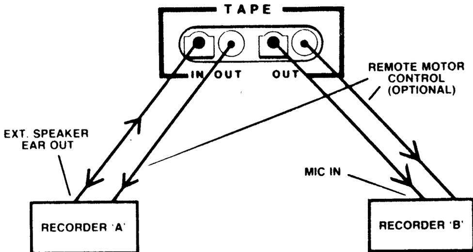
This configuration enables you to easily read files into memory from Recorder A (the "player"), edit them, and then write the new versions to another tape in Recorder B (the "recorder").
