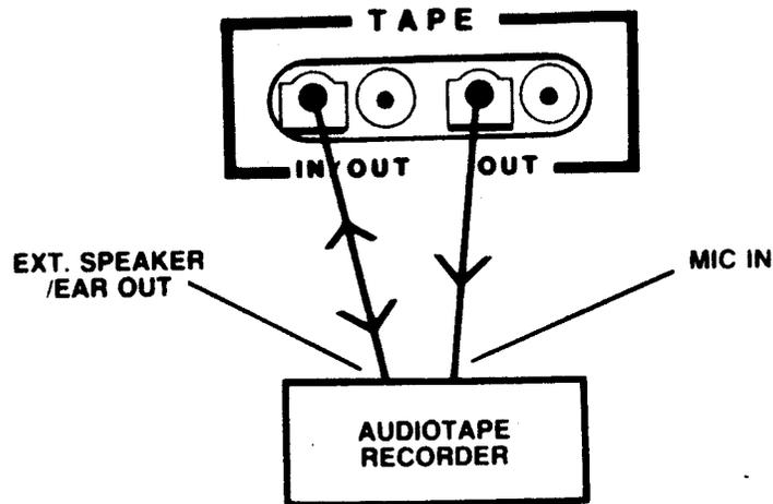
With this configuration, reading files into memory from the tape as the tape plays back and writing files onto tape from memory are separate tasks, usually punctuated by changing tapes or fast-forwarding past existing files.
