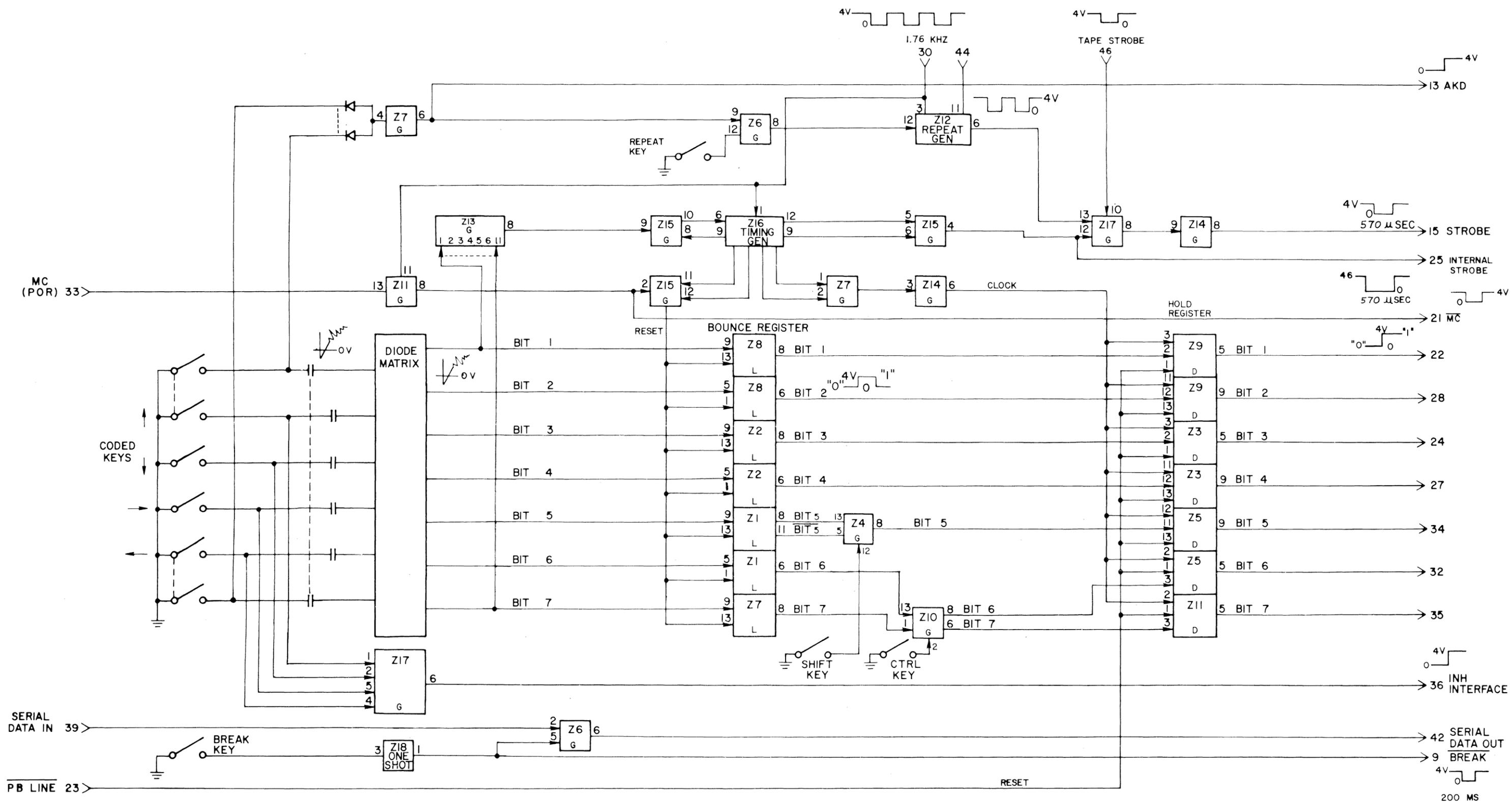
Figure 2-3. Block Diagram, Keyboard
