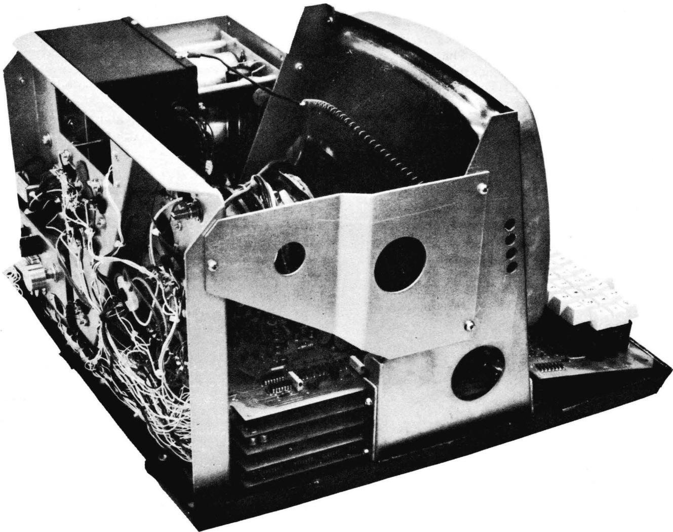
Figure 3-1. Datapoint 3300 with Cover Removed
