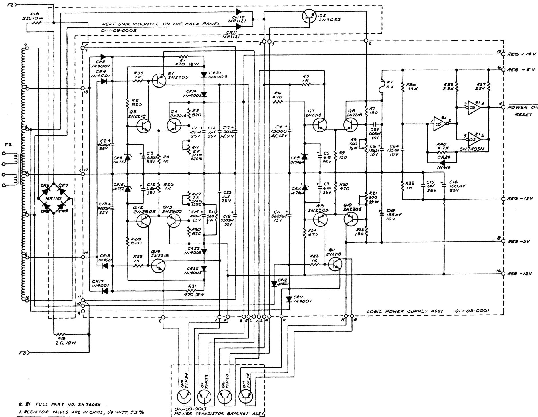
Figure 2-23. Schematic Diagram, Logic Power Supply
