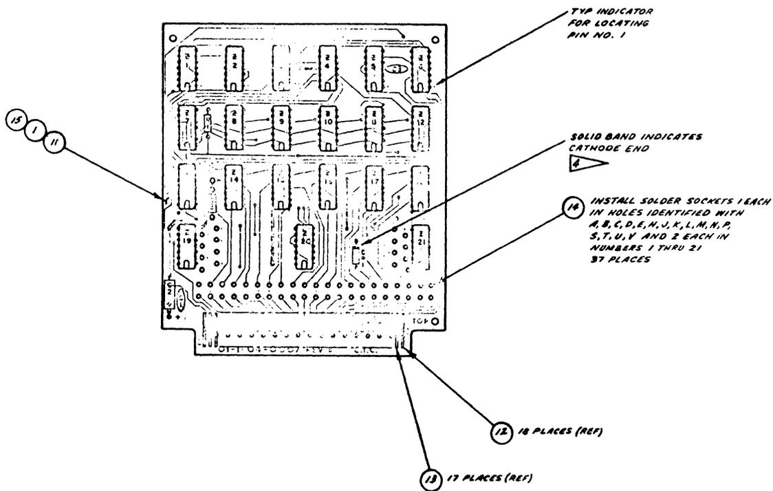
▲ THE CATHODE END OF ALL DIODES IS INDICATED BY EITHER A COLOR BAND, A DOT, OR THE END FROM WHICH THE BANDS ORIGINATE.
