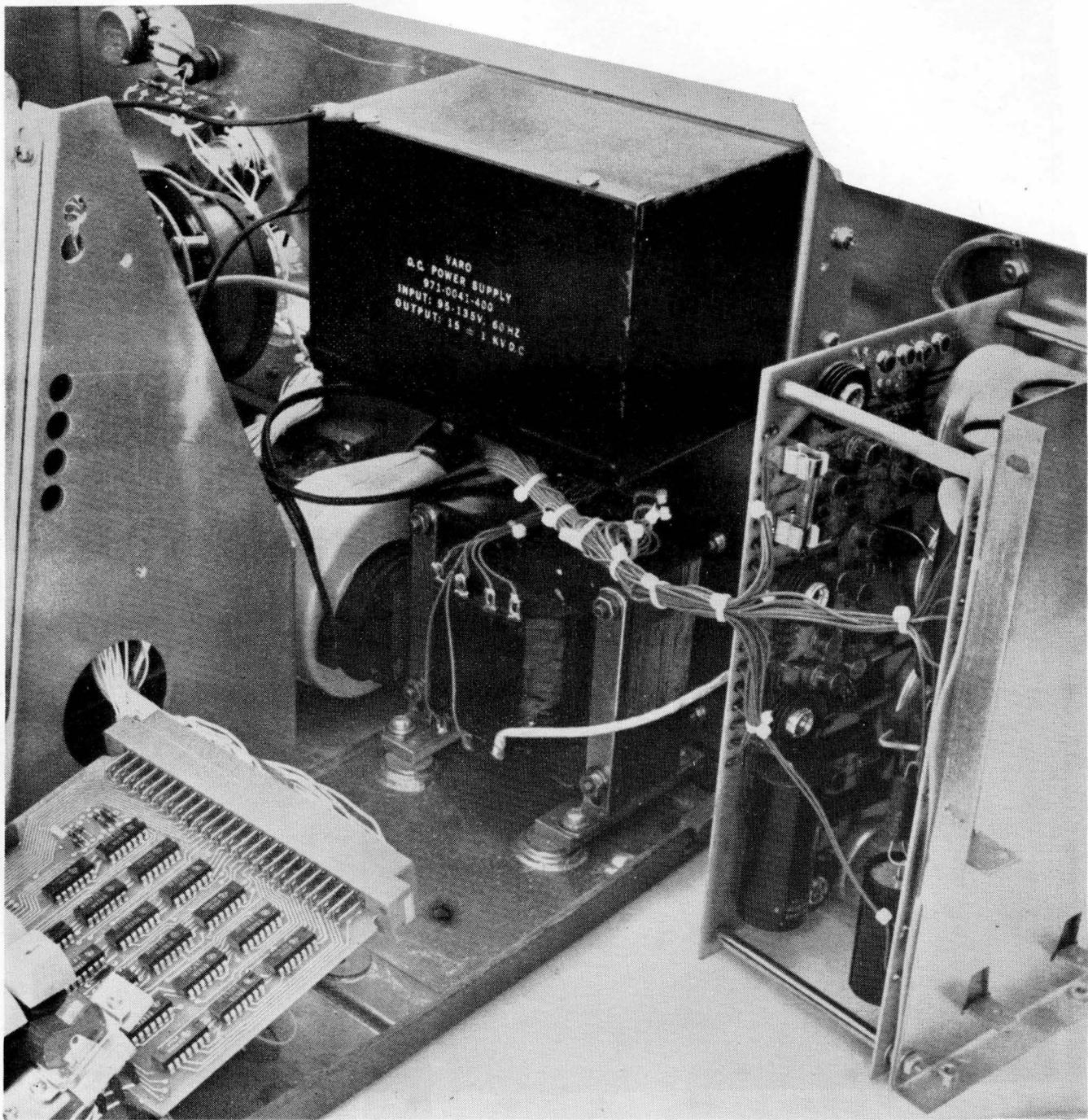
Figure 3-5. Logic and Deflection Power Supplies
