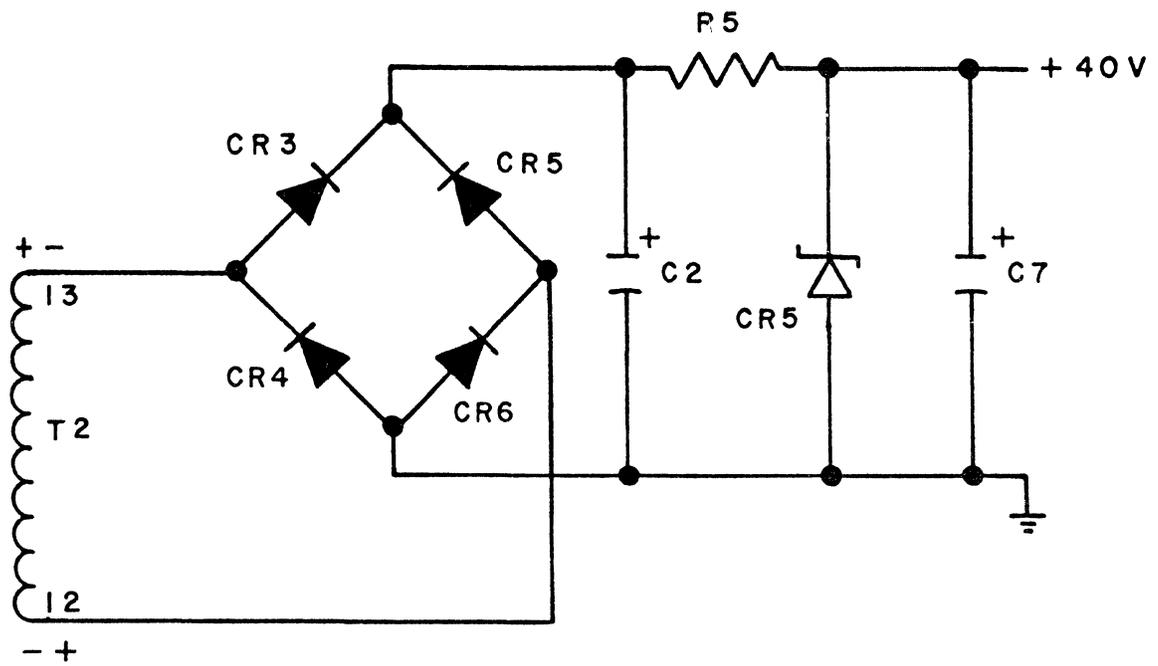
Figure 2-24. +40VDC Circuit
