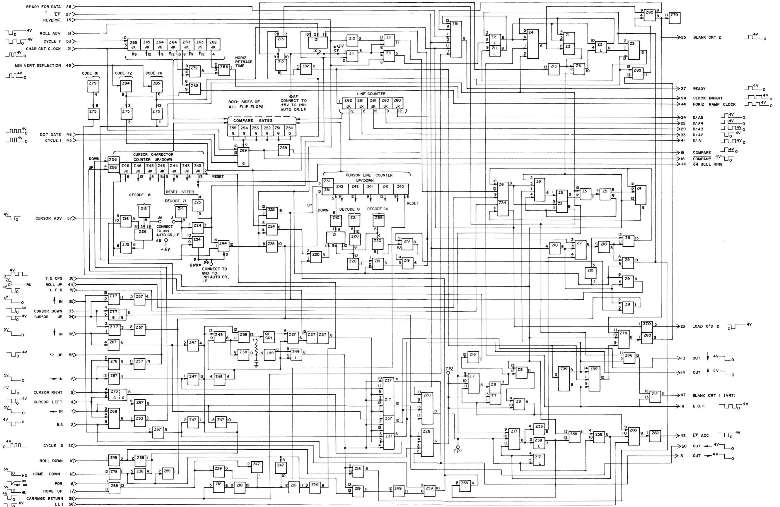
Figure 2-27. Block Diagram, Control Logic
