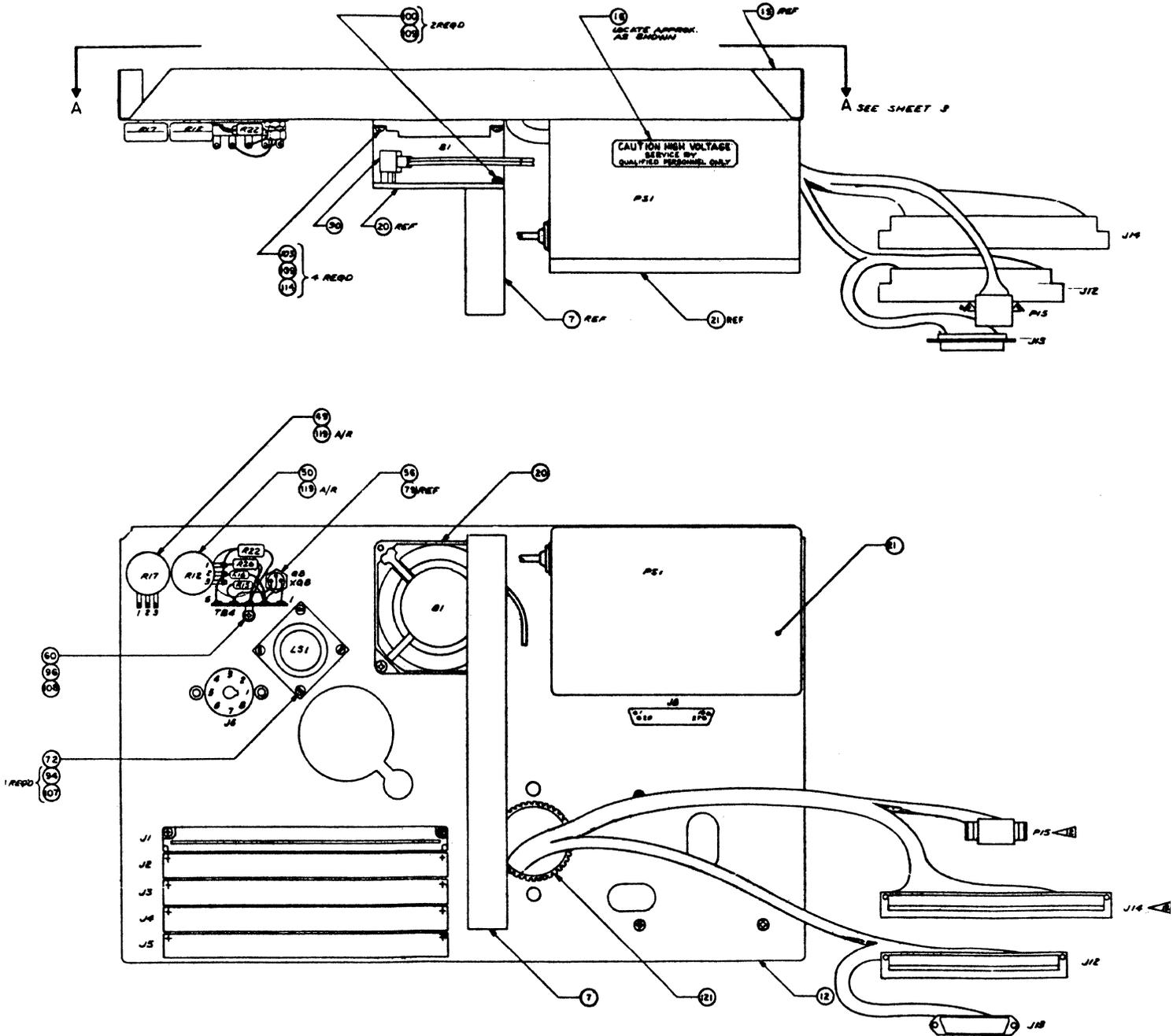
Figure 3-14. Rear Panel Assembly (1 of 3)
