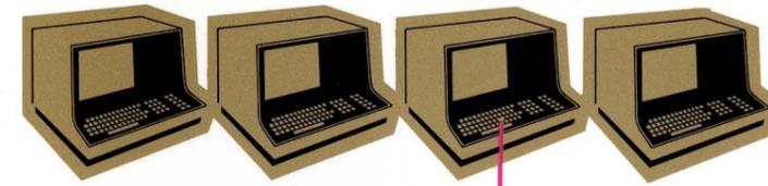
Data communications between the central processor and the field work stations can be accomplished either through "hard wires" — as when the stations are located near the central processor — or through telephone lines — as when the stations are located cross-country many miles away.
