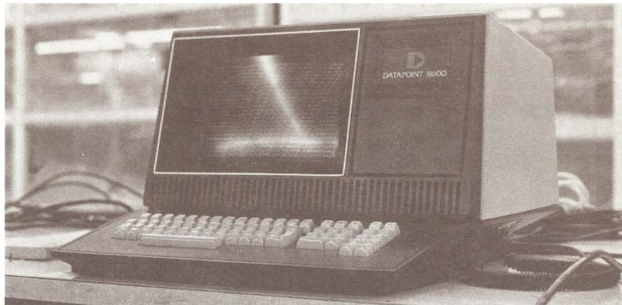
**Newest addition to the Datapoint family** - *Designed with the user in mind, the Datapoint 8600 features a powerful central processor and a memory capacity of up to 256K.*
