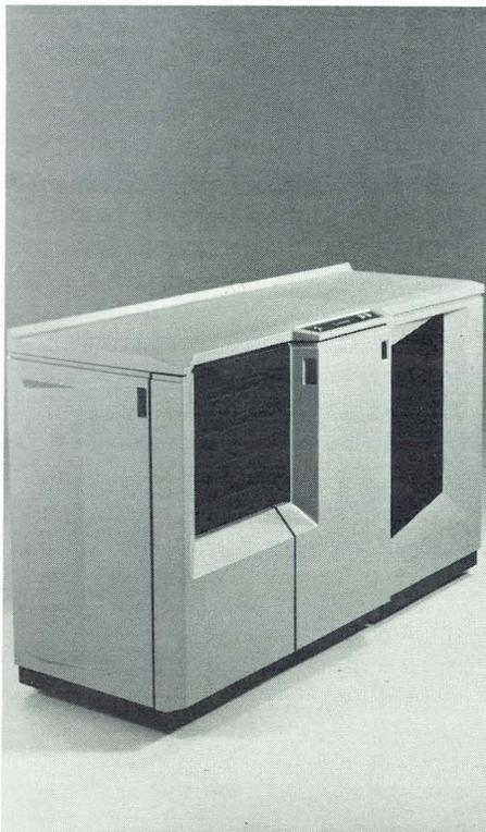
Datapoint's new 9660 Laser Printer is a laser-scanned electrophotographic, non-impact printer. The excellent print quality is one feature that makes the 9660 Laser Printer well suited for office applications.
