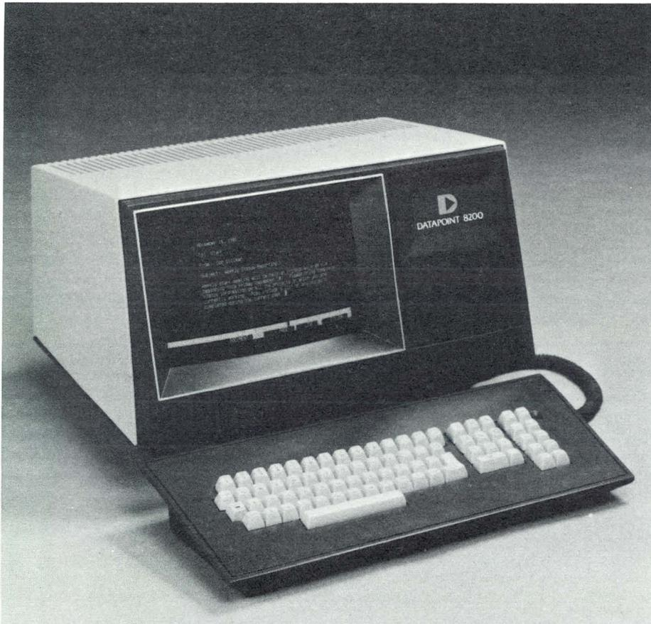
An 8200 may be attached to a packet switching network via a Program Access Device (PAD). This allows for protocol translation.
