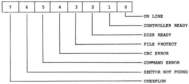
All of the bits have been explained in the previous discussion except for FILE PROTECT which is simply connected to the corresponding button on the front of the selected drive. If this bit is true (the button on the front of the drive is lit), no data will be written on the disk, even though it will appear to the program that the write operations are being performed. None of the status bits are affected by the EX STATUS command.
