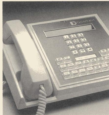
INFOSET II is the multi-line phone with 16 programmable keys for single-button line and feature selection. Selectable features include such things as automatic call back, call forwarding, call privacy, paging access, directed call pickup, leave message, and timed reminder. A built-in speaker gives you hands-free operation and a 24-character alphanumeric display presents status, call, or directory information.
