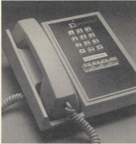
INFOSET I is the basic, single-line telephone with the most commonly used call handling features - connect, pickup, transfer, conference, and hold - on single-button feature keys. Other features available with ISX can be accessed by dialing a feature access code. Automatic dialing of up to 19 numbers and automatic redialing are also available.
