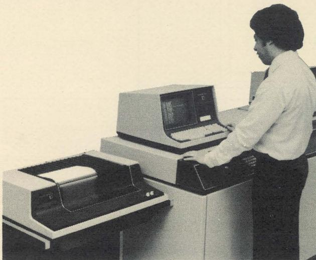
Manufacturing Systems' 8800 Processor with an 8200 Workstation as system console and 80 CPS printer for hard-copy output of system messages.
