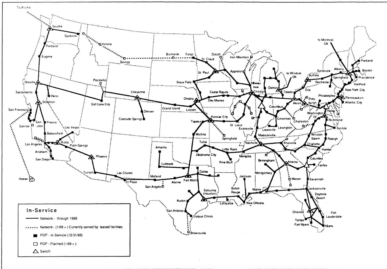
Figure 1. US Sprint's Nationwide Digital Fiber Optic Network.
