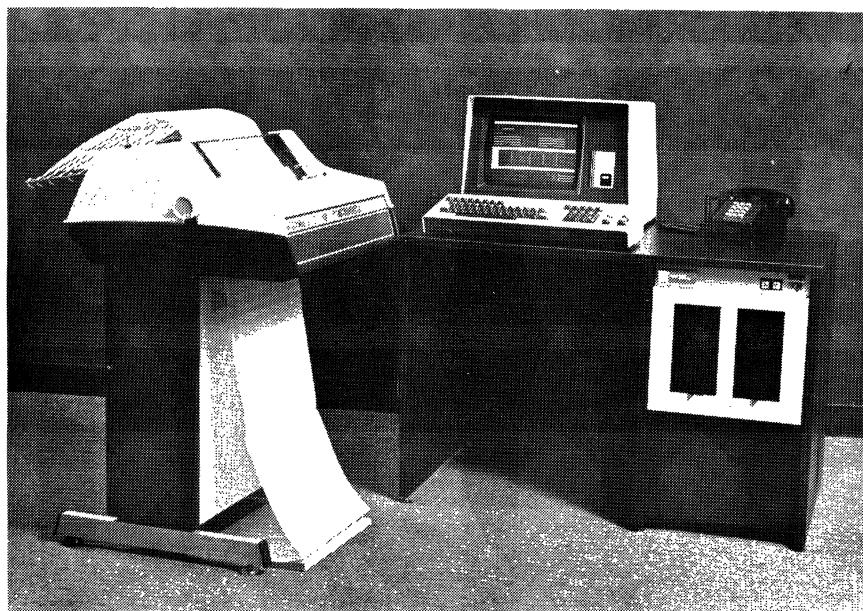
This Western Union terminal configuration, which includes a Video 200 terminal, a serial impact printer, and dual floppy disk drives, illustrates the types of ancillary devices which can be interfaced with display terminals. Other devices include cassette or cartridge tape drives, disk drives, line printers, magnetic stripe, card, and tape readers, optical character and bar code wand readers, and paper tape punches.
