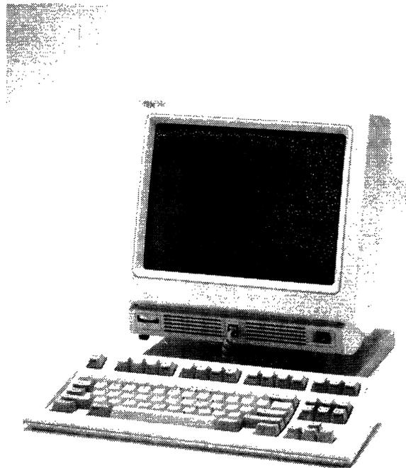
*The IBM 3151 ASCII Display Stations are available in three models and feature 10 non-IBM ASCII emulations including TeleVideo, Zentec, ADDS, and Hazeltine. In addition, the Models 310/410 include IBM 3101 emulation and accept five optional slim-line cartridges supporting a total of 20 additional emulations.*
