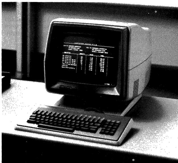
*The ET 1100 display terminal is Burroughs' general-purpose workstation for the company's computer systems. The standard ET 1100 is equipped with RS-232-C/TDI interfacing; the ET 1101 version features Burroughs BDAA communications.*
