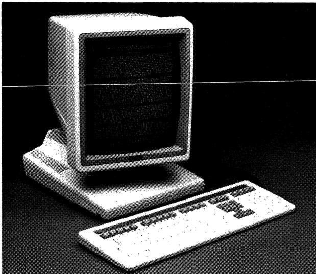
*The CIT-500 is a word processing/text editing display with full overstrike capability. The 15-inch vertically oriented display screen provides a full-page display of 64 lines by 80 characters.*
