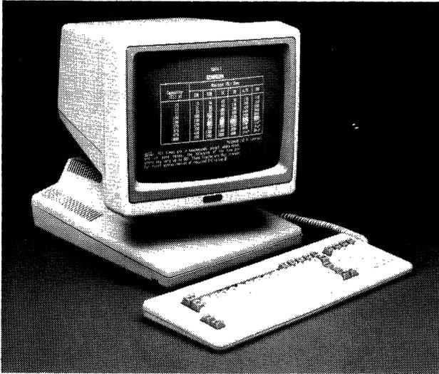
*The CIT-101e is an ergonomically designed DEC VT100 (and VT200) emulator. The unit contains a 14-inch tilt/swivel display with selectable 24-line by 80/132-character formats. The keyboard is detached and features a low-profile design.*
