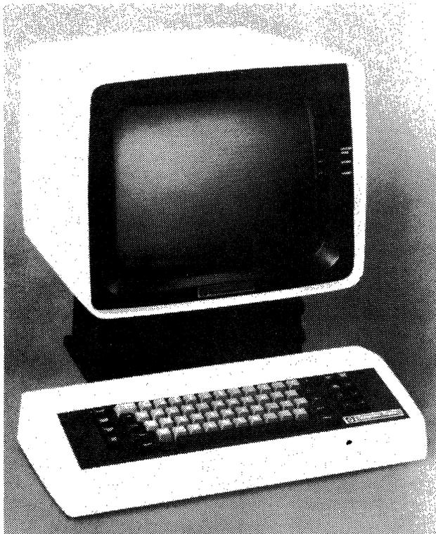
The Computer Optics Mark IV Clustered Display System was originally marketed as the CO:77 Information Display System. The system is a plug-compatible replacement for the IBM 3270 Information Display System. Computer Optics is now a division of Four-Phase Systems, which supplies maintenance service to users.
