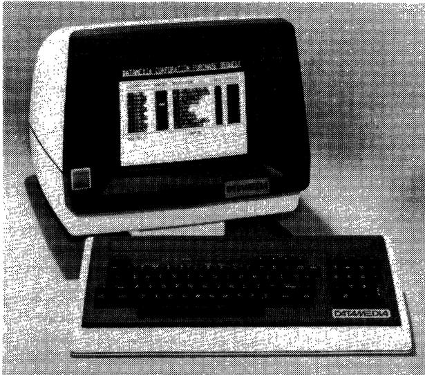
*Datamedia's Excel Series of display terminals are ergonomically designed. The display monitor can be tilted from 5° to 15° to achieve the most comfortable viewing angle. The keyboard is detachable, and connected to the monitor via a six-foot coiled cord. A choice of 12-inch or 14-inch screen sizes is available.*
