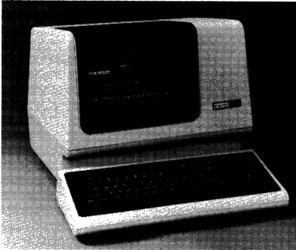
*The DEC VT100 is one of the most popular, as well as one of the most widely emulated, video display terminals on the market today. When equipped with the Advanced Video Option, the terminal can display 24 lines of 80 or 132 characters, and features video attributes such as bold, blink, underline, and reverse on a character-by-character basis.*
