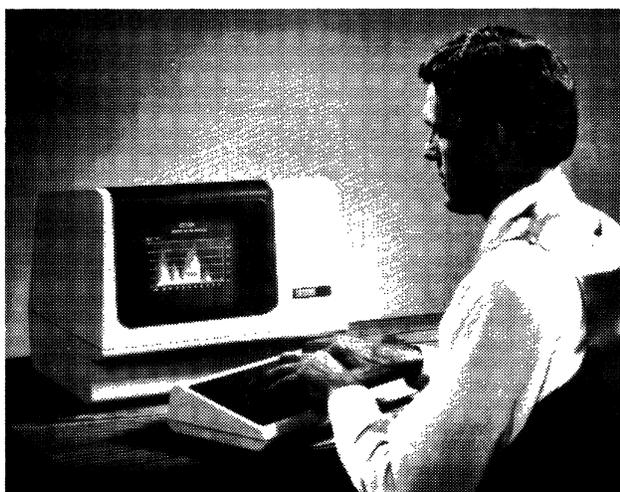
The VT125 features business graphics, as well as alphanumeric, capabilities. Using DEC's Remote Graphics Instruction Set (ReGIS), pictorial data is created and stored as simple ASCII text.
