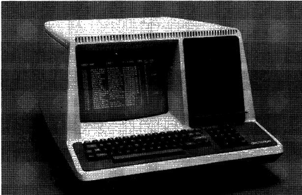
The VT52 has the same physical appearance as the VT50, but features an auxiliary keypad (standard), a 1920-character screen, and several other significant features not found on the earlier VT50.
