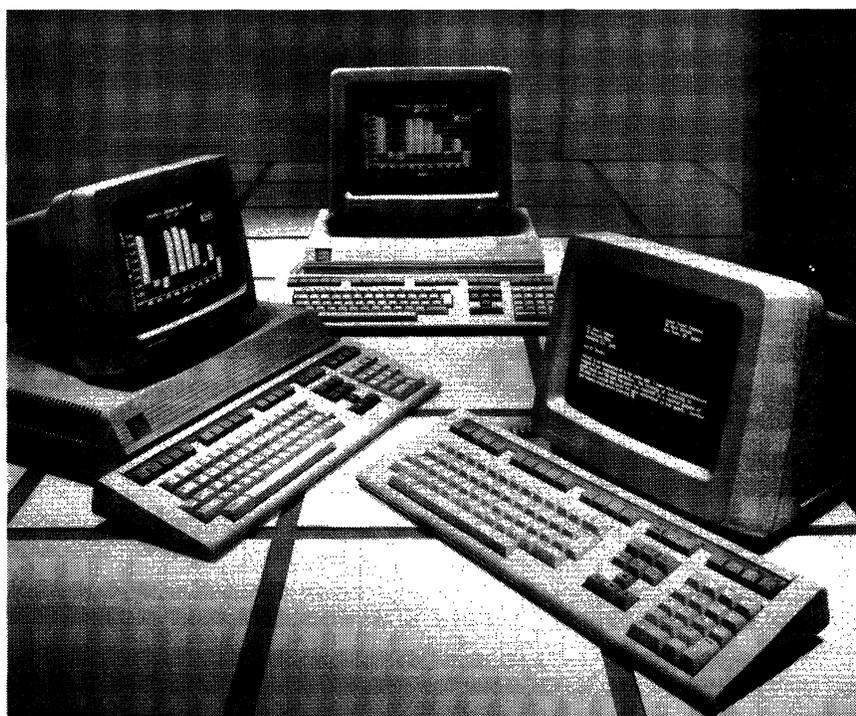
*The Digital VT200 family of video display terminals consists of three models. The VT220 features full VT100 compatibility, the VT240 provides bit-mapped graphics architecture and text/graphics capabilities, and the VT241 replaces the monochrome display of the VT240 with a color monitor.*
