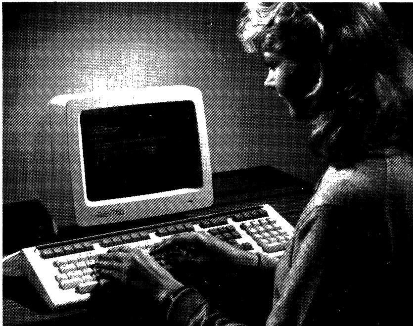
*The VT220 is the low-end model in DEC's new VT200 terminal family. The VT220 features two-piece modular construction, with a 12-inch monochrome display and a detachable, low-profile keyboard. As with all of the new VT200 terminals, the VT220 boasts full DEC VT100 compatibility, including 80-/132-column display capability and compatibility with the ANSI X3.64 standard. As was the case with the VT100, several vendors have recently introduced terminals designed to emulate the VT220.*
