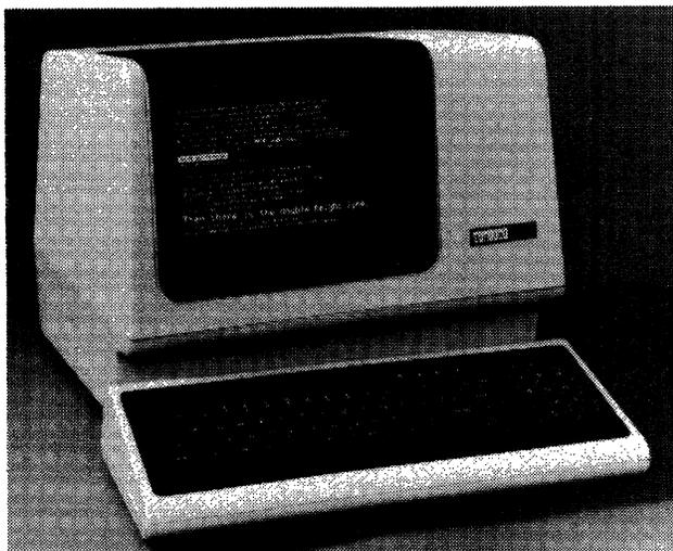
A stand-alone teletype compatible display terminal capable of displaying either 80 or 132 characters per line. Standard features include detached keyboard, reverse video, split screen addressable cursor, selectable transmission rates, and parity.
