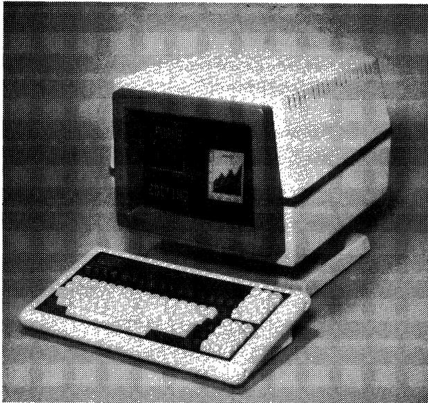
The Human Designed Systems (HDS) Concept Series features a 12" diagonal display mounted on a pedestal base. The keyboard (shown here with the 11 additional function keys) is detached. The photo reflects some style changes in the display console which were made recently by HDS.
