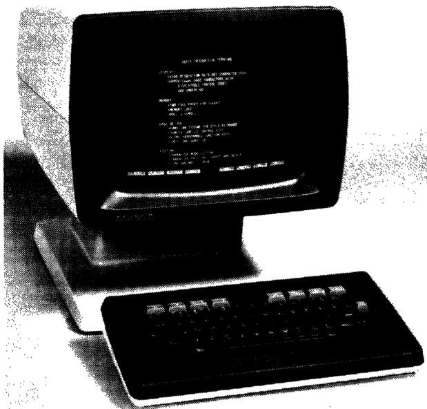
This Hewlett-Packard 2621A terminal features a 12-inch diagonal CRT display with a screen capacity of 1920 characters and 68-key detachable keyboard. Terminal operation is controlled by a Zentec Z-80 microprocessor.
