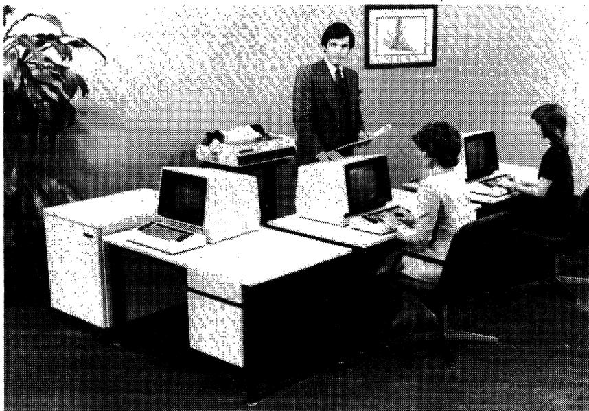
Harris' 9200 system is a family of IBM 3270-compatible components. Two system models are currently available: the 9210 and 9220. Both models can support up to 32 devices per processor, with both local and remote communications capabilities. Shown here are the 9200 processor (left), 9287 matrix printer, and 9278 CRT displays.
